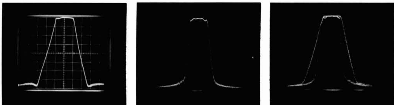
A. 2.1-kHz i-f passband of the stock 455A21 mechanical filter.
