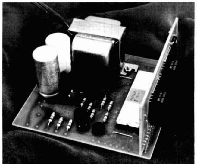
Layout of the digital clock PC board. Three-terminal voltage regulator is not installed, nor is the phototransistor display control circuitry.
