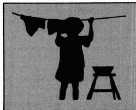
Silhouette as broadcast by the Jenkins Laboratories in 1928. The image size shown here is the approximate size of the image seen by "lookers in."
