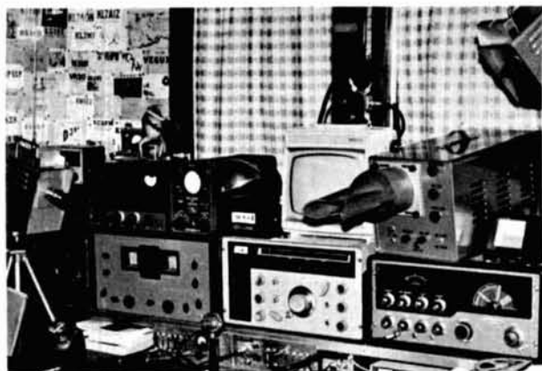
Slow-scan setup used by Don Miller, W9NTP, in 1969. Equipment was very up to date at the time, included a sampling slow-scan camera (left), a shuttered camera (upper right) and both slow- and fast-scan monitors. Don's sampling camera was one of the first of its type and was widely duplicated by amateurs.
