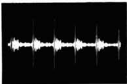
Fig. 1 SSB signal before processing. See the high peaks and the low valleys. Our NCX-3 is putting out only 25 watts average power.
