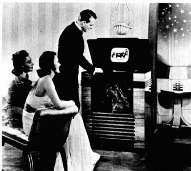
This television set, first introduced by RCA for public use at the New York World's Fair in 1939, featured a picture reflected from the top of the kinescope to a mirror on the underside of the cabinet's uplifted lid. (Photo courtesy RCA)
