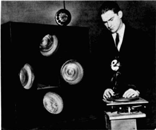
In the early 1930s, Felix the Cat was the first "star" to appear before RCA-NBC experimental television cameras. Felix whirled around on his phonograph turntable for hours on end while four hot arc lights beat down on him. In those early days the crude TV images of Felix looked like he was being viewed through a venetian blind. (Photo courtesy RCA)
