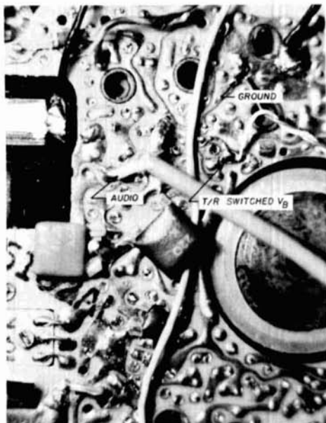
Interconnect points for the Touch-Tone encoder installed in a Motorola HT-220.
