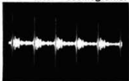
Fig. 1 SSB signal before processing. See the high peaks and the low valleys. Our NCX-3 is putting out only 25 watts average power.
