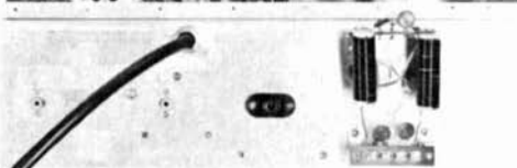
Rear view of output components of the linear showing the 4-1000A and B&W pi-network inductor.
