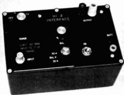
The high-impedance meter interface instrument is built into a cast aluminum box, Bud type CU347.
