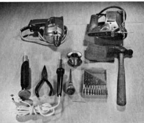
fig. 1. A few simple tools are required for building your own printed-circuit boards.
