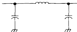
fig. 1. The pi network is so named because of its basic resemblance to the Greek letter \pi .
