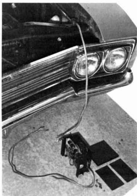
Above, mobile power supply and cable. Photo below shows routing of coaxial cable under side panels.
