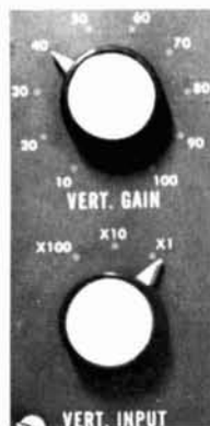
fig. 5. Vertical input knobs affect size of display on screen; on some scopes, they (along with graticule lines on the screen) help with voltage measurements.
