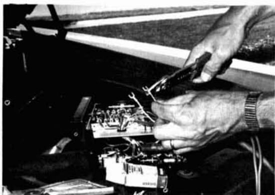
Finishing the wire ends.
