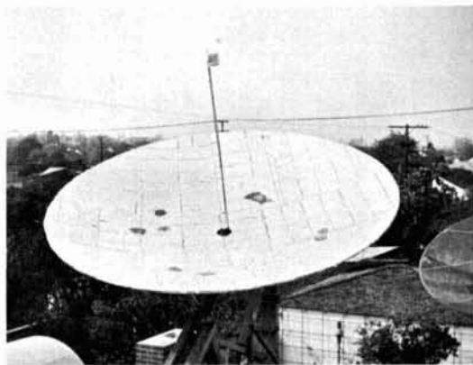
Newly installed reflector with a temporary feed for sun noise measurements.
