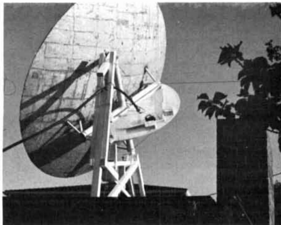
Completed dish and polar mount. Co-axial feedline is 1-5/8" Heliax.
