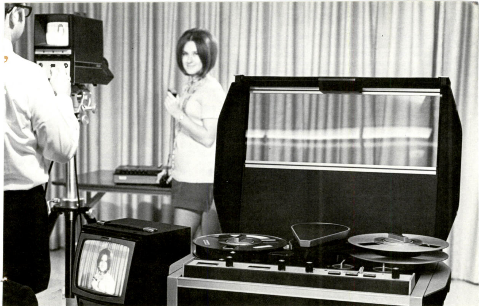
The cornerstone of most cablecasting operations is the video tape recorder.
