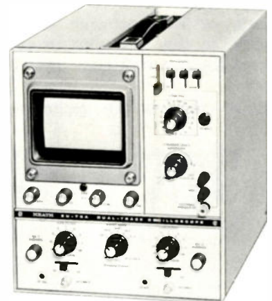
This oscilloscope (EU-70A Heath Dual-Trace) has the triggered sweep feature, recommended for studio testing.
