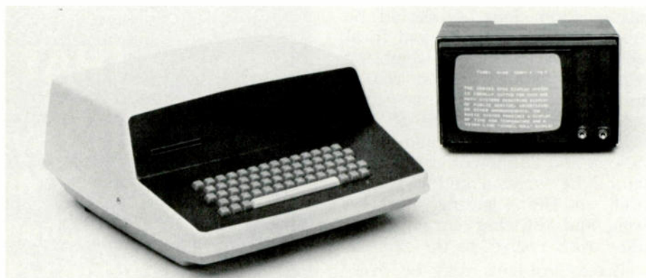
The Data Technology keyboard (shown here) contains all the electronics for the message display system. The monitor is used to edit messages before they are exposed to viewers.
