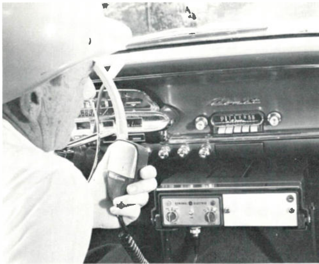
Control head of GE UHF radio fits limited spaces.
