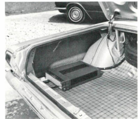
Remote control head (top photo) allows trunk-mounting of transceiver chassis in system manager's car.
