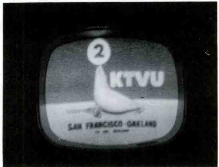
This type of picture can be improved by application of a low-noise pre-amp.
