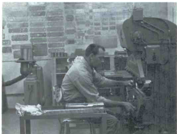
AMECO amplifiers, splitters and the 101 other CATV units start here in the metal stamping room.
