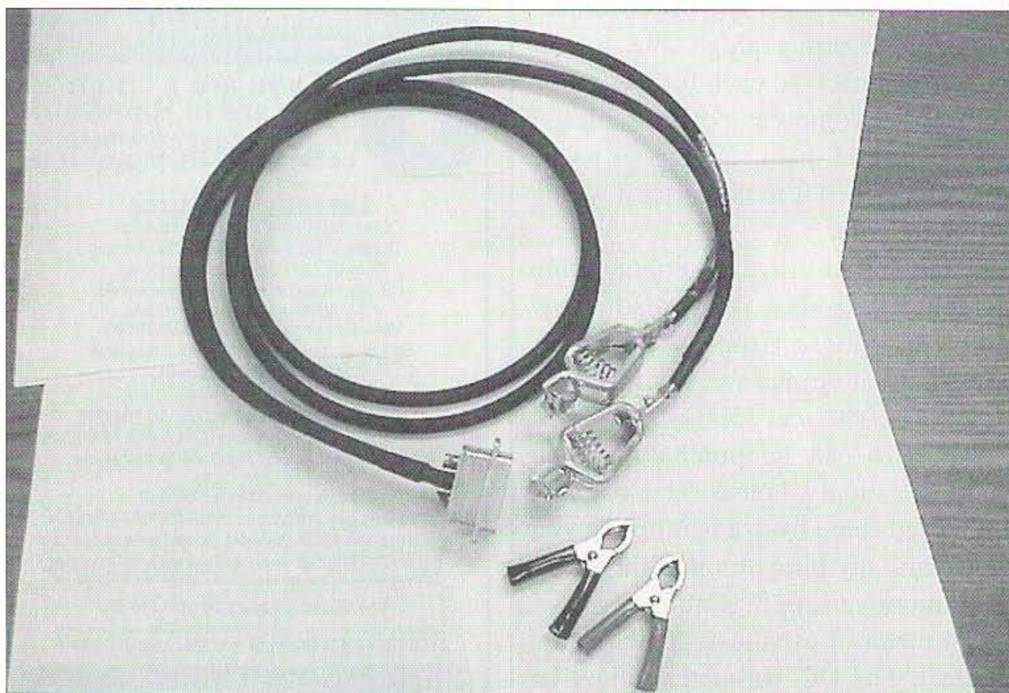
Photo 1. This cable plugs into the inverter assembly and can be connected to any 12-volt battery. The small clamps below came with the inverter.
