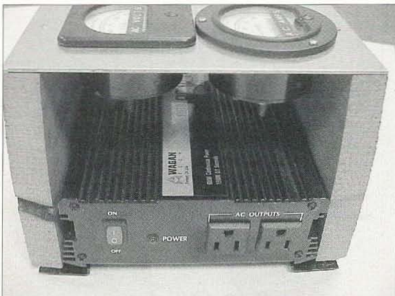
Photo E. This shows the front end of the inverter assembly. Wood screws attach the inverter mounting brackets to the wood sides.
