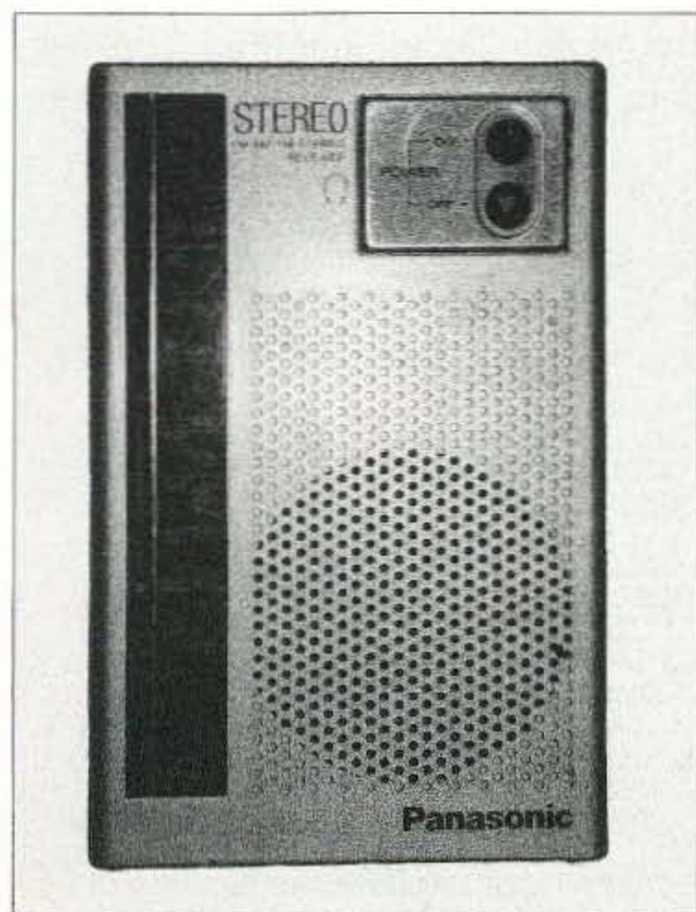
Photo A. Shown is the front face of a Panasonic model RF-455 broadcast AM/FM/FM-STEREO pocket radio.
