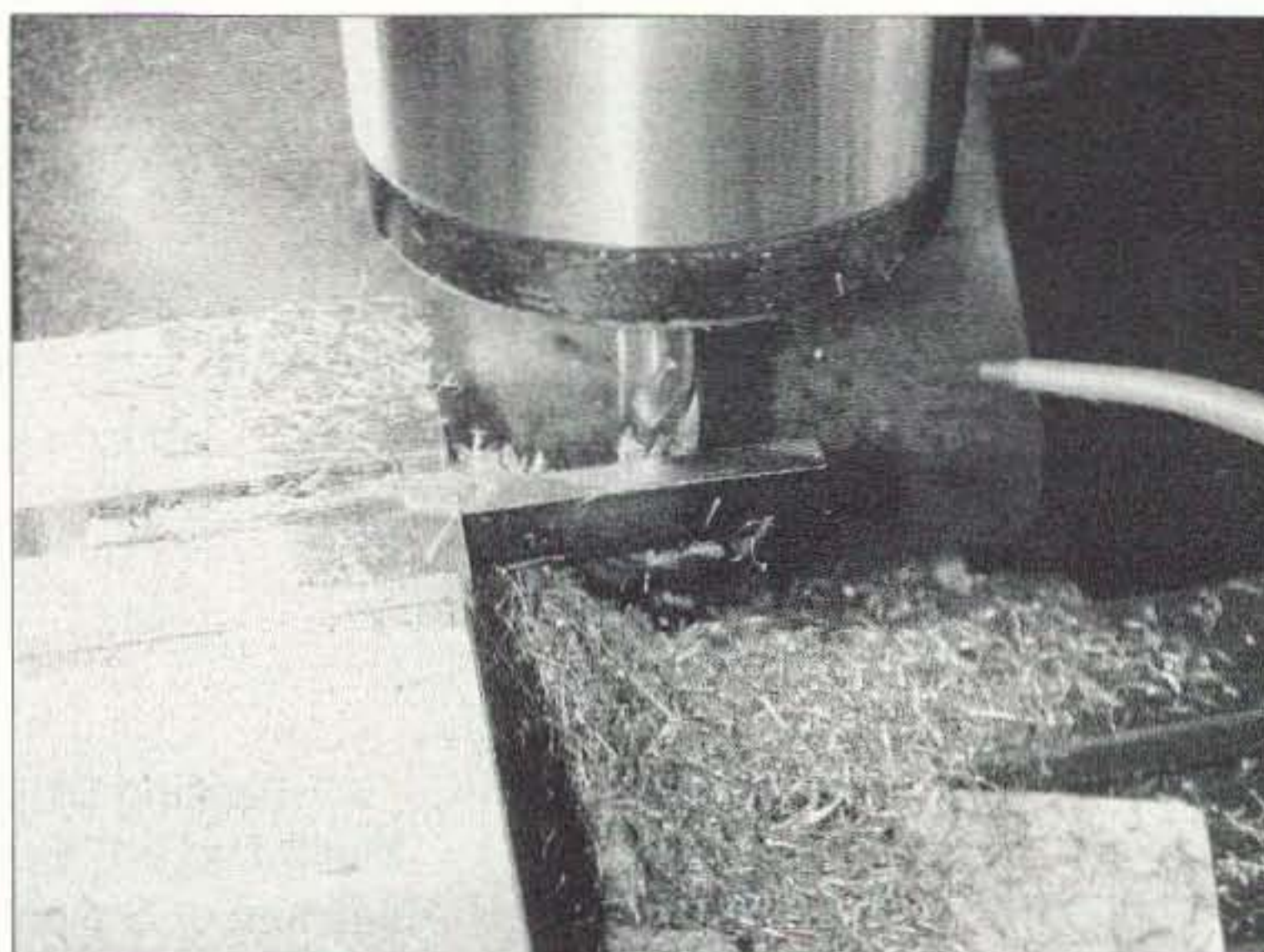
Photo D. Milling the reduced part of the armature.
