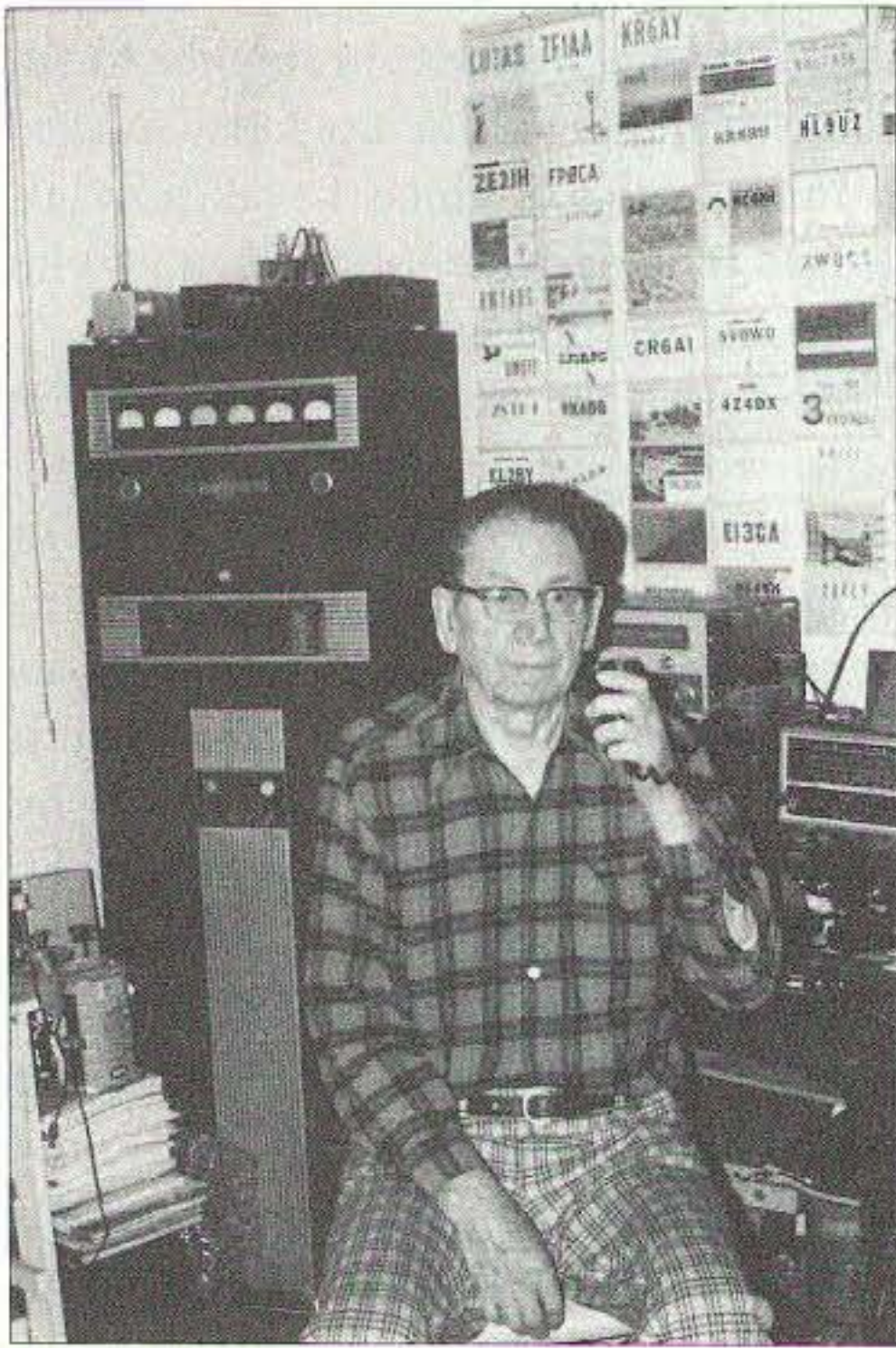
Photo B. Joe W9CYT/SK, long-time Elmer and friend, shown operating 220 MHz. Note the 160m AM Collins cabinet in the background; and home-brewed coffee-can duplexers for 220 MHz standing on a stack of magazines next to the Collins.
