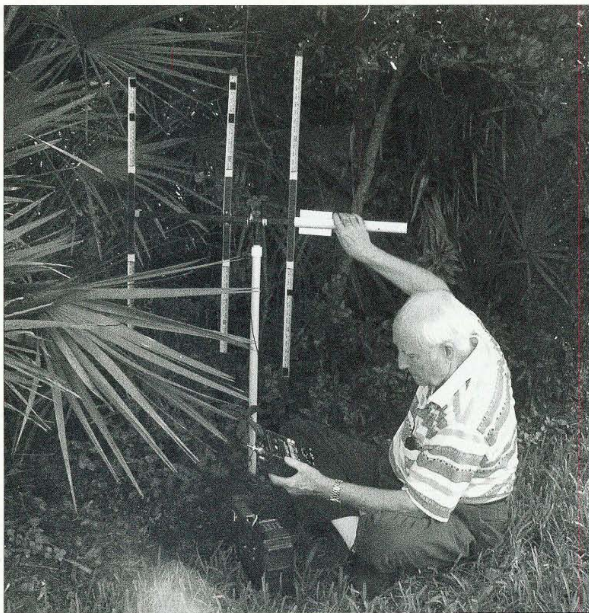
Photo A. Hider John Munsey KB3GK checks the SWR and pattern of his tape-measure beam just before the hunt starts. The strong signal in front of his beam will entice the hunters to come in through a swamp instead of a dry route from the back. (All photos provided by KB3GK)
