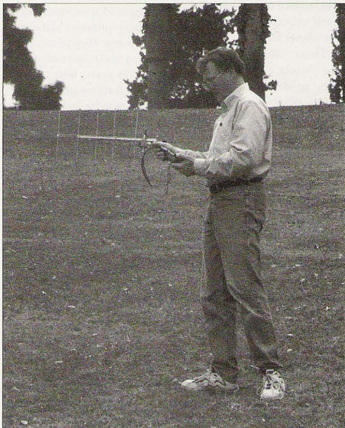
Photo D. Dave Reeves AC6PP uses a small yagi and his scanner on the SuperSystem 440 MHz transmitter hunts in Orange County CA. Such a setup is easily adapted to foxhunting on the FRS band.
