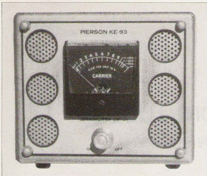
Photo D. Front panel view of the Pierson base power supply. The "S"-meter and manual transmit standby switch are shown.
