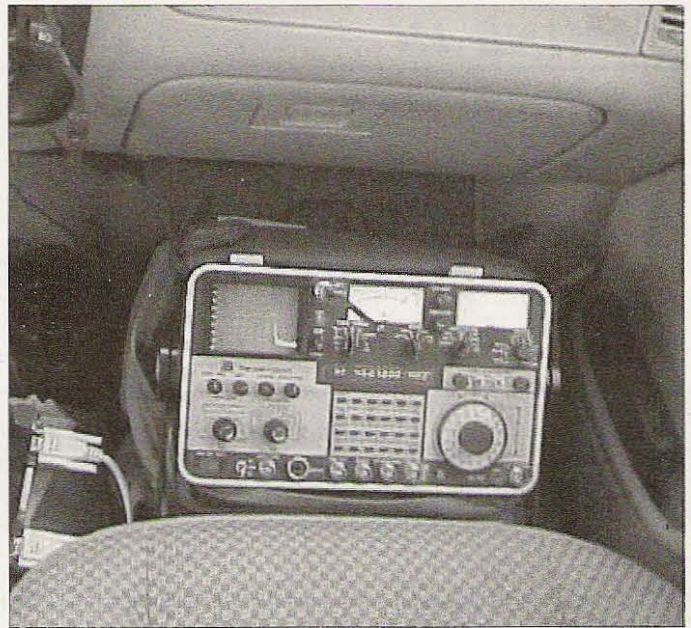
Photo C. KG6AOH usually does his transmitter hunting alone. His IFR-1200 Service Monitor sits where the passenger's legs would normally be. (Photo by Paul Shinn)
