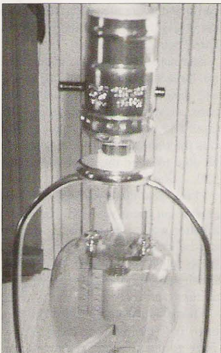
Photo E. The light fixture mounted to the harp.
