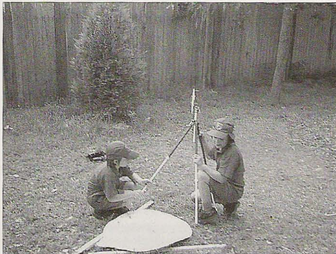
Photo A. Julian and Daniel orienting and setting up the antenna pedestal.
