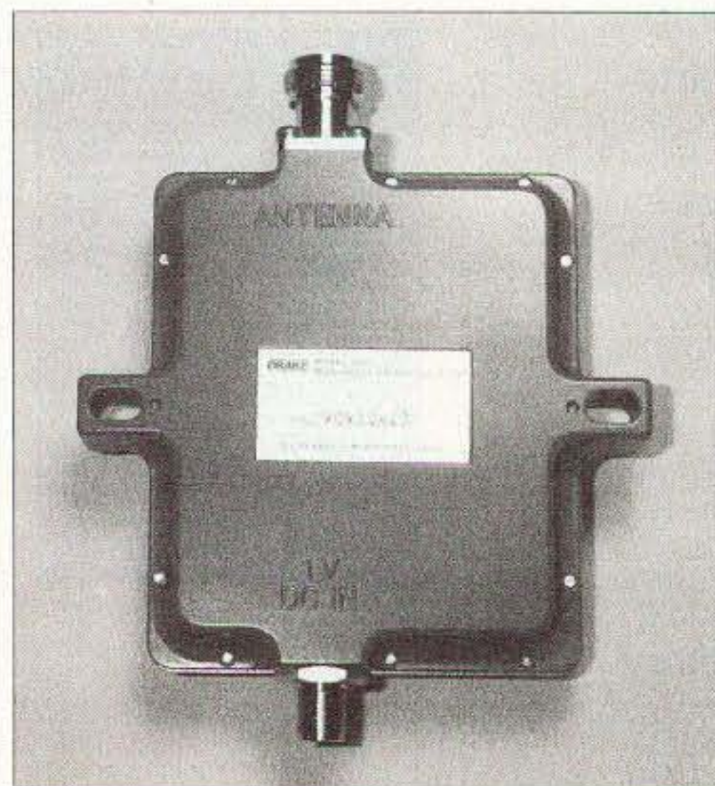
Photo A. The Drake 2880 commercial microwave downconverter.
