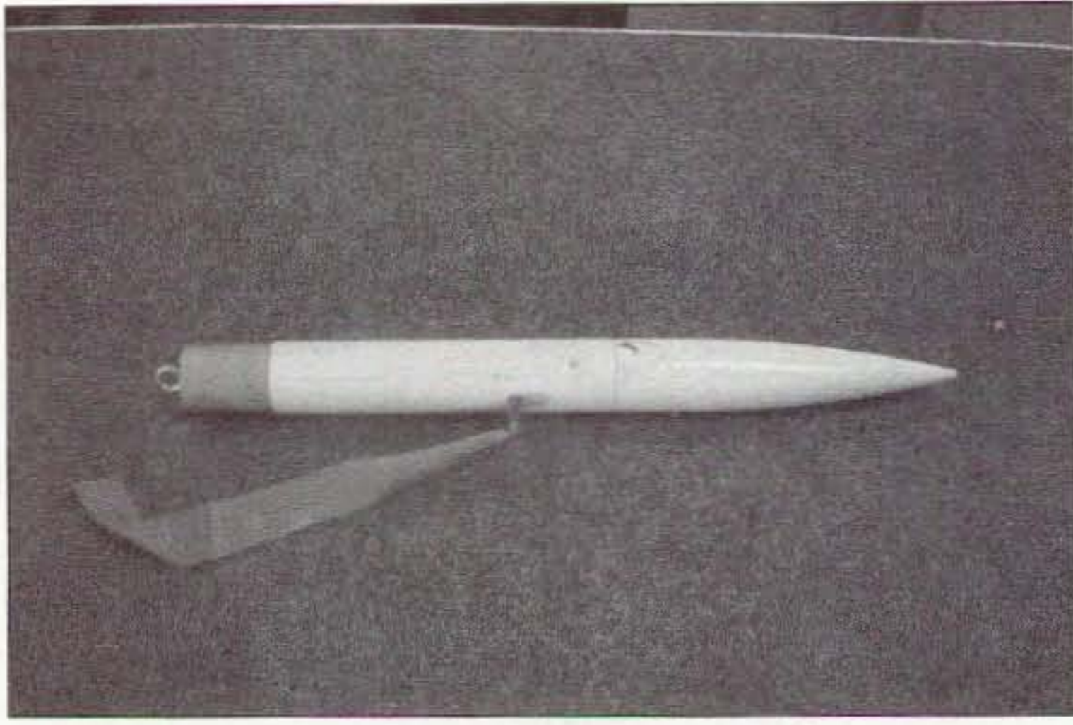
Photo D. Payload section, with arming jack in place.
