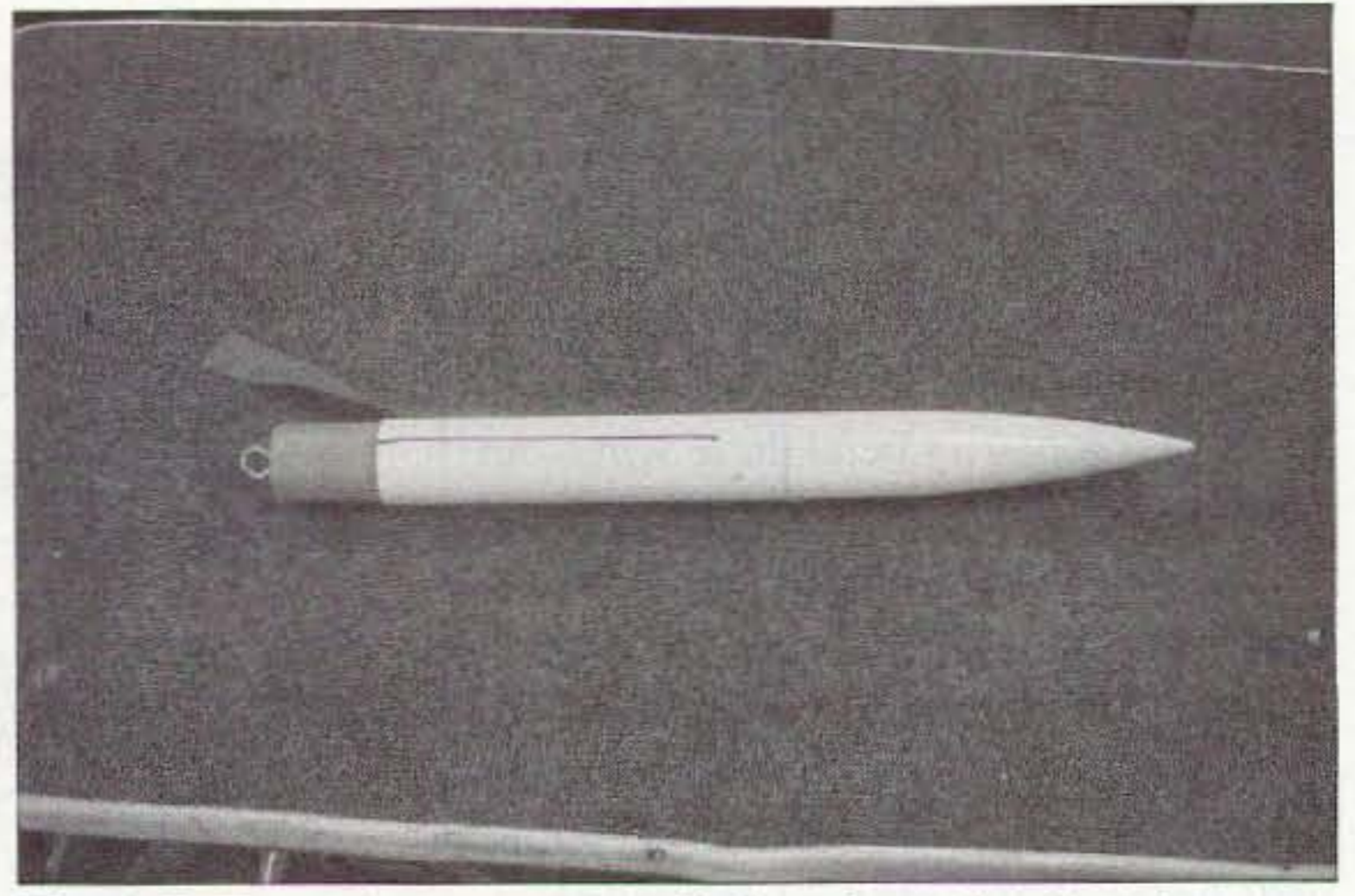
Photo E. Transmit antenna installed on the payload section.
