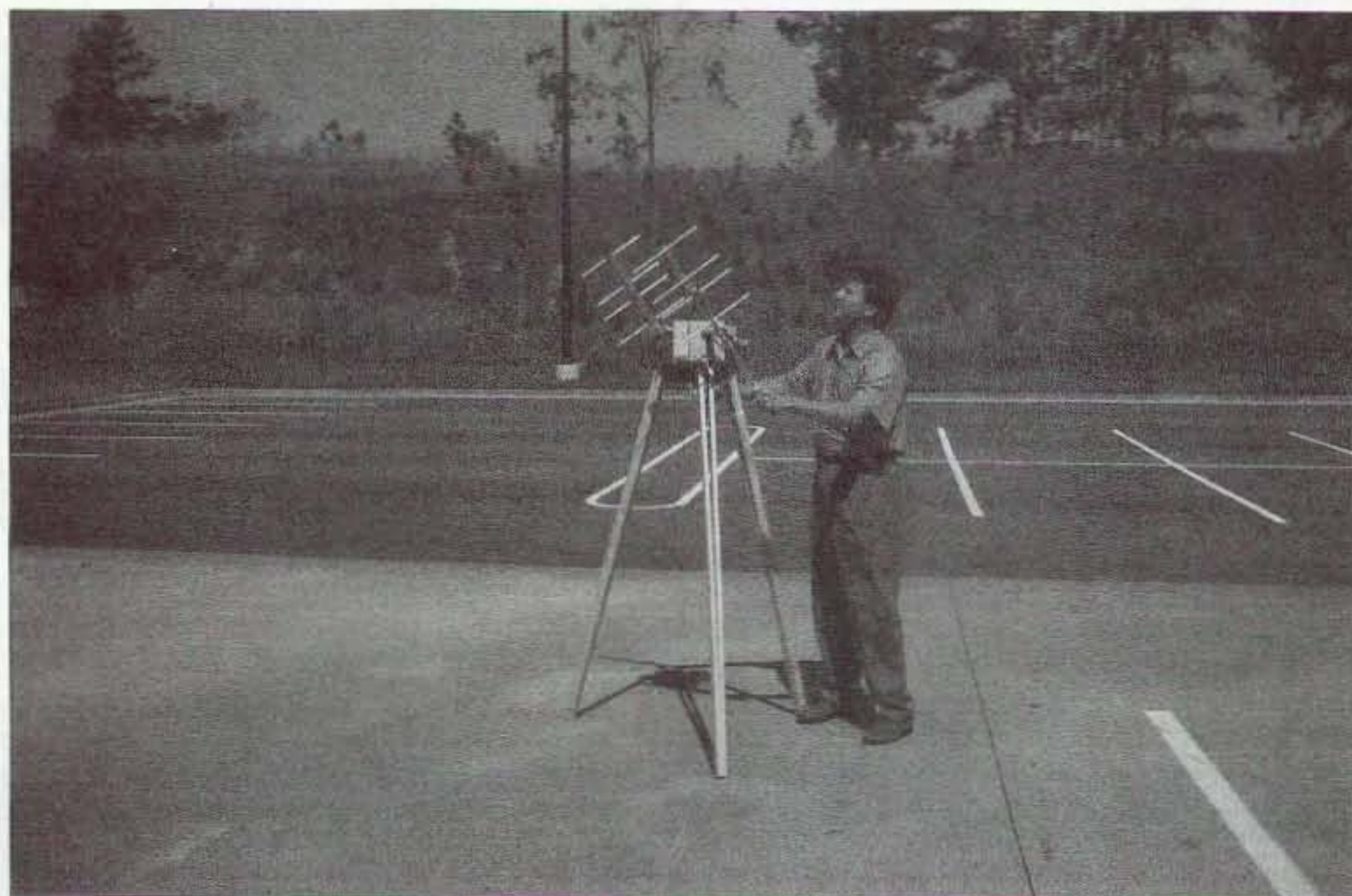
Photo A. Completed antenna array in tracking mode.
