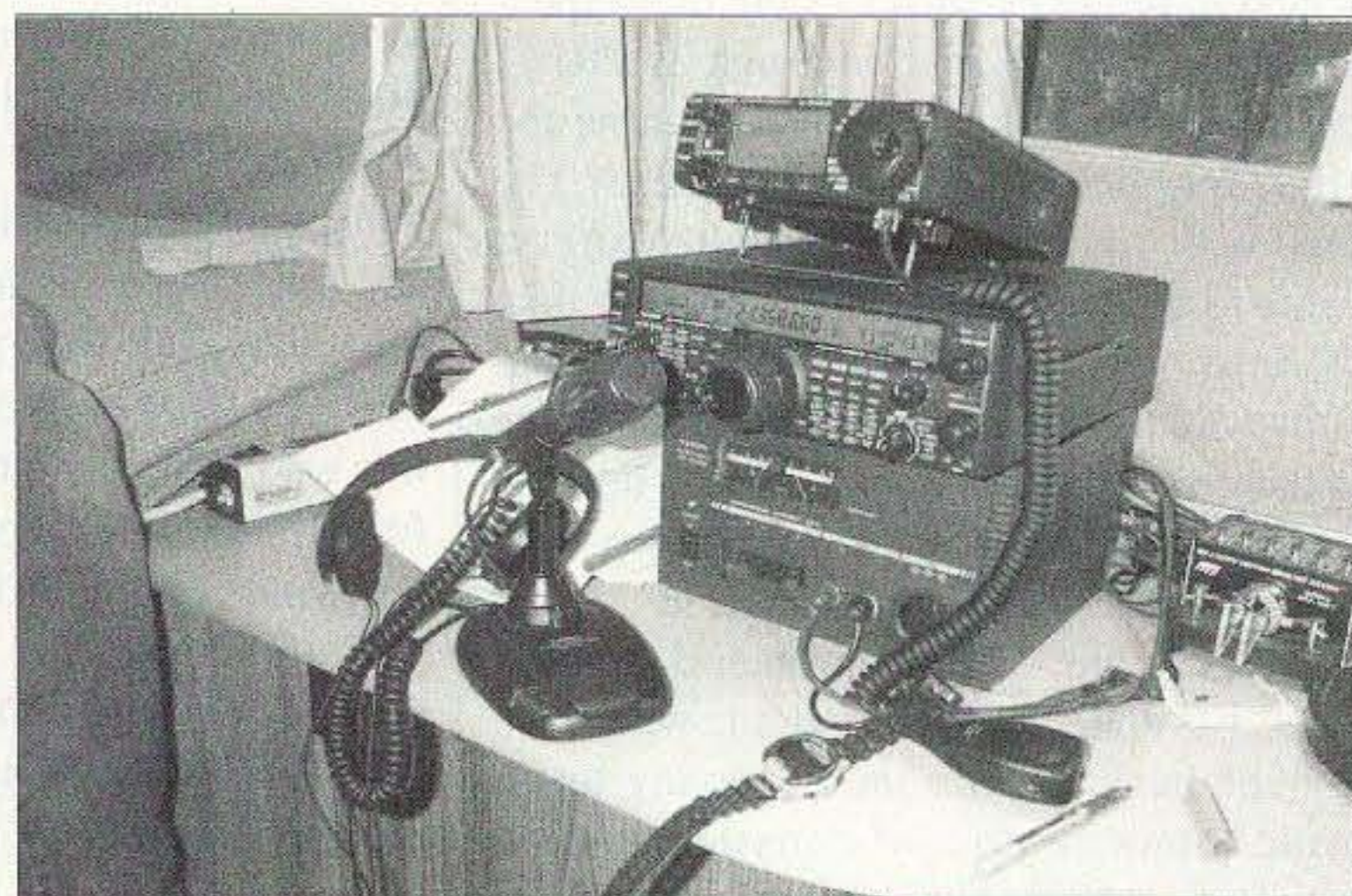
Photo B. Yaesu FT-847s were used for both HF and satellite use during Field Day at W5ACM.
