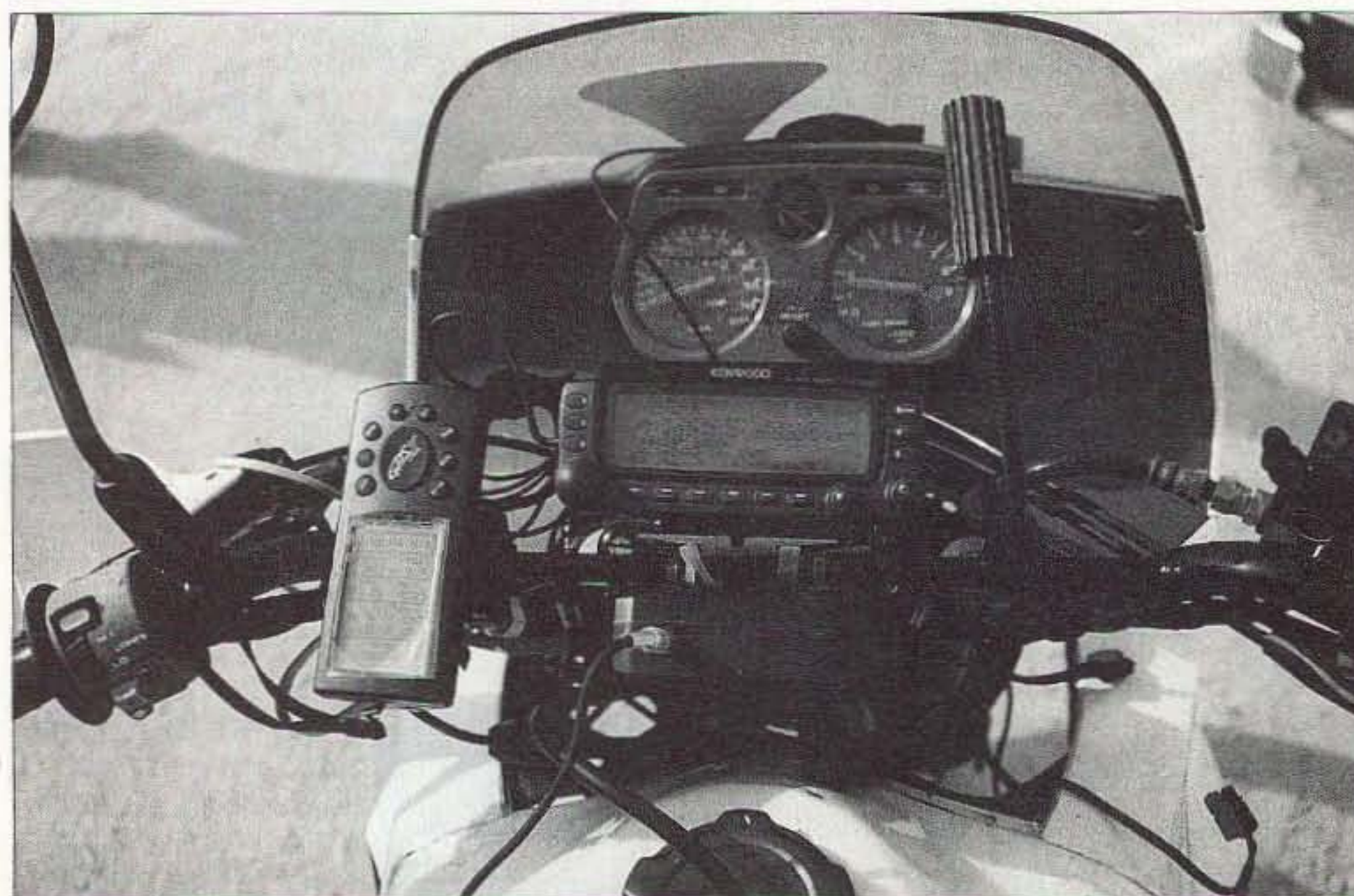
Photo E. Motorcycle mobile ham is a great class demo! This system has full APRS capability.
