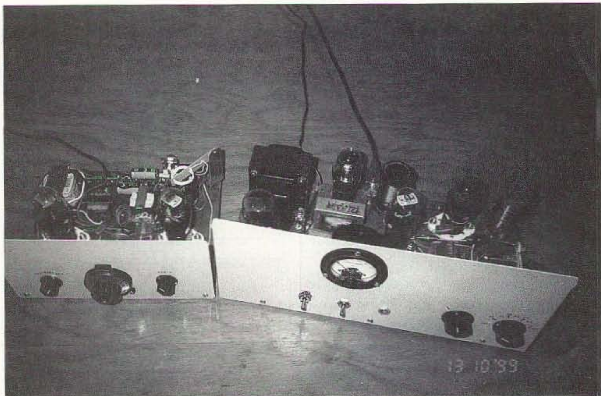
Photo A. The receiver at K8JWR consists of a type-27 triode regenerative detector and 27 audio amp. The transmitter uses a 27 Hartley oscillator and 27 neutralized amp at 4 watts output. The power supply uses a type-80 rectifier and VR-150 regulator. It's all built on pine boards with aluminum front panels.
