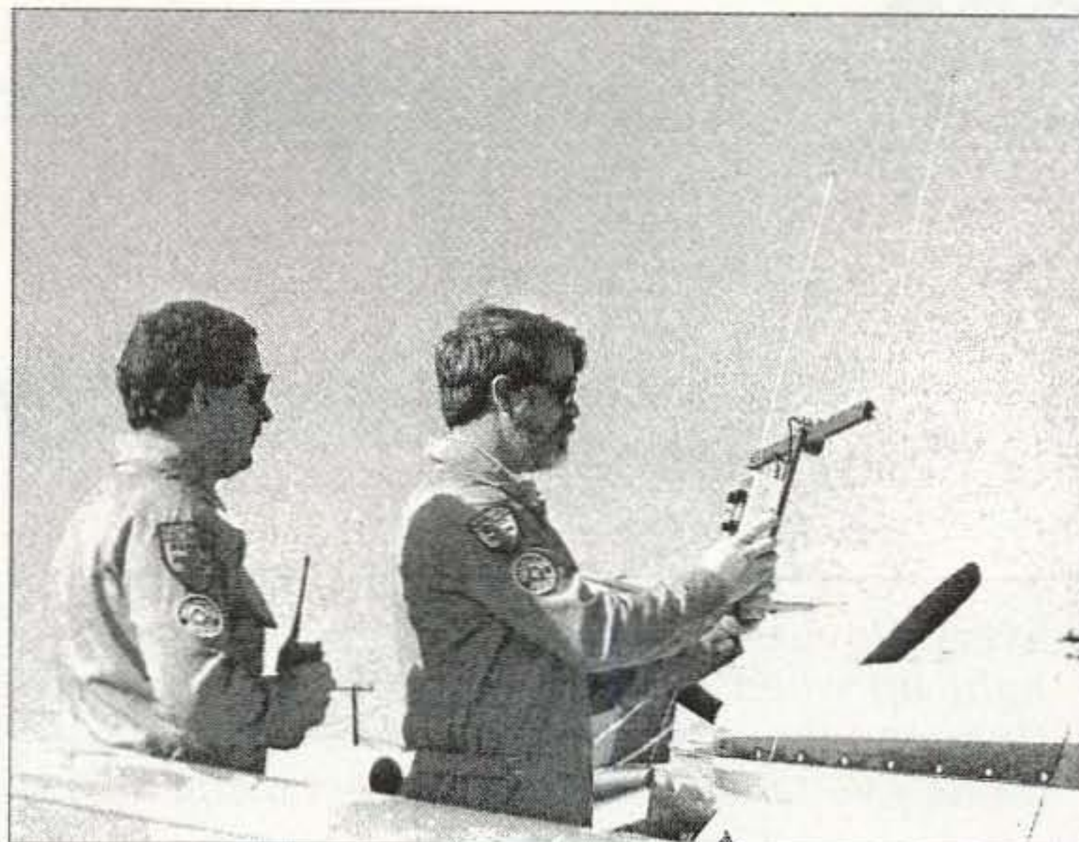
Photo B. It's that one! Steve Kirkman KB6IMB (left) and Jim Frank KB6ONC of the Los Padres Search and Rescue Team use their RDF set to find a squawking ELT at the Santa Barbara airport. (Photo courtesy of Lou Dartanner N6ZKJ and Austin Rudnicki K6IA)
