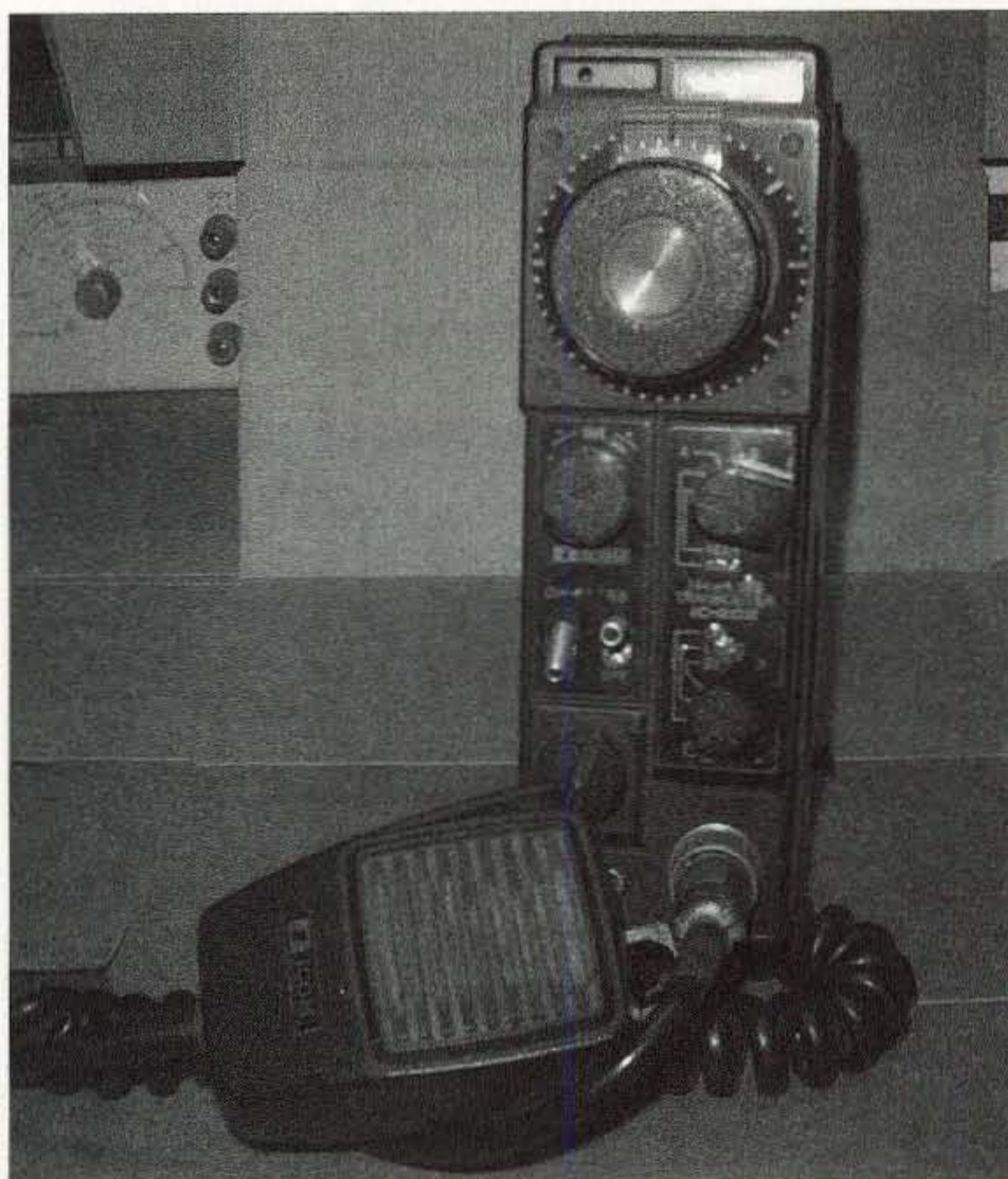
Photo A. Older Icom IC-202 SSB portable uses 9 internal "C"-size cells for portable operation.
