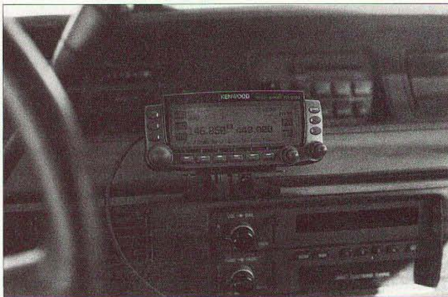
Photo B. The control panel's light weight allows it to be mounted almost anywhere. It is easily removable to discourage would-be thieves.
