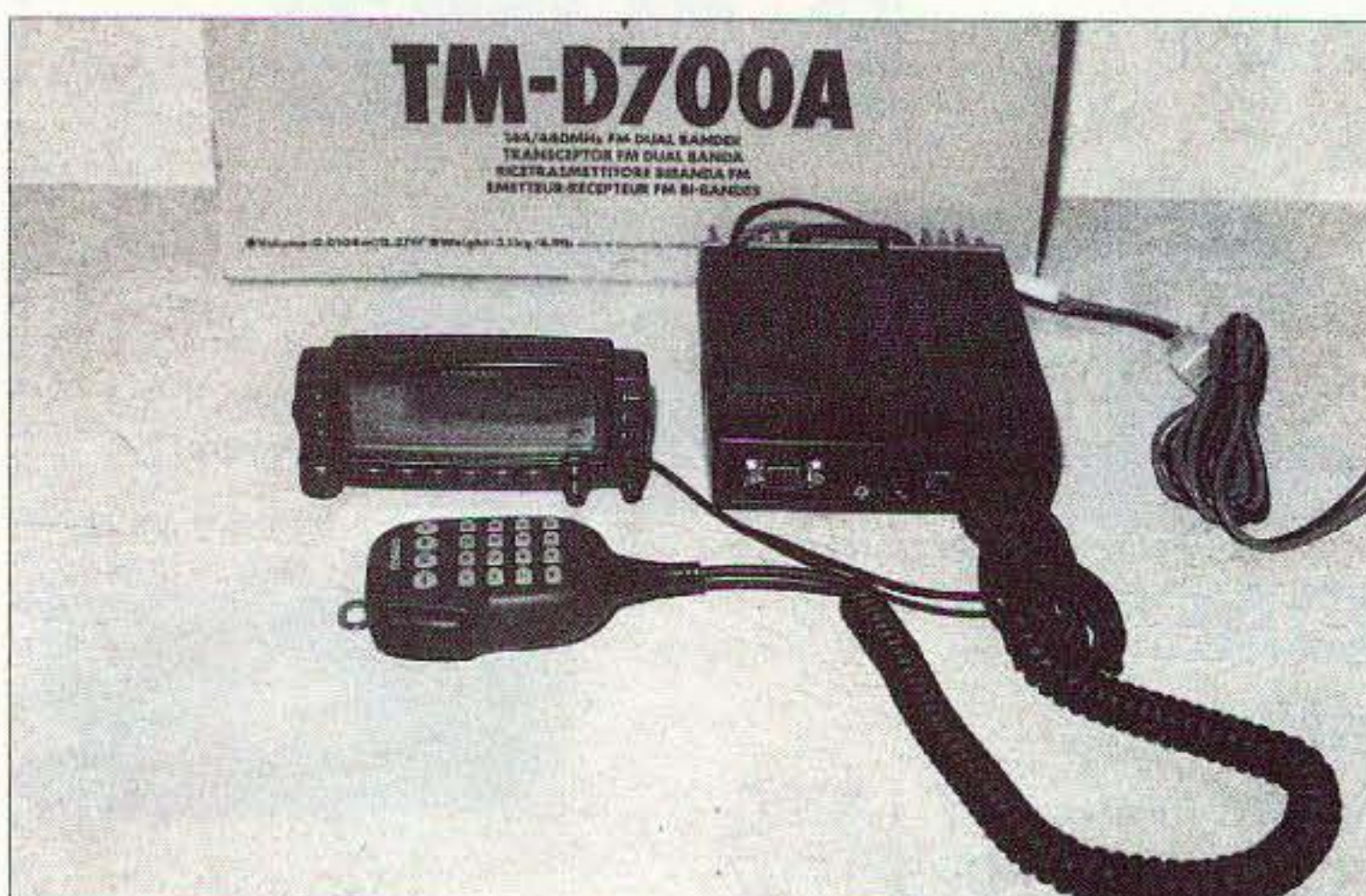
Photo A. The Kenwood TM-D700A comes complete with main unit, control panel, MC-53DM programmable microphone with alphanumeric keys and all necessary cables, brackets, and hardware. It even includes the cable for connection to a GPS receiver.
