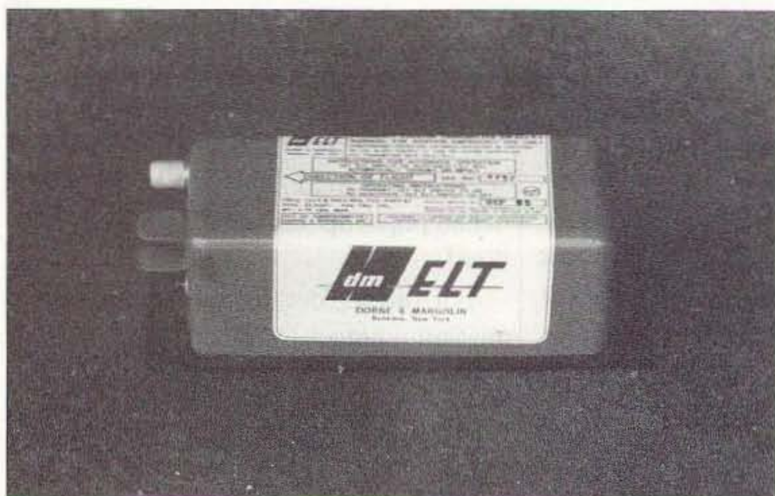
Photo A. This Emergency Locator Transmitter (ELT) mounts in the tail of a small plane and activates on impact. (Photo by Tom Curlee WB6UZZ)
