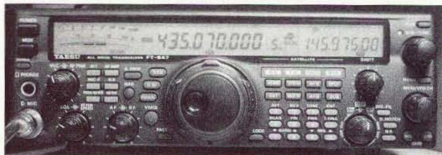
Photo A. A Yaesu FT-847 tuned and ready for a UoSAT-OSCAR-14 FM-voice pass.
