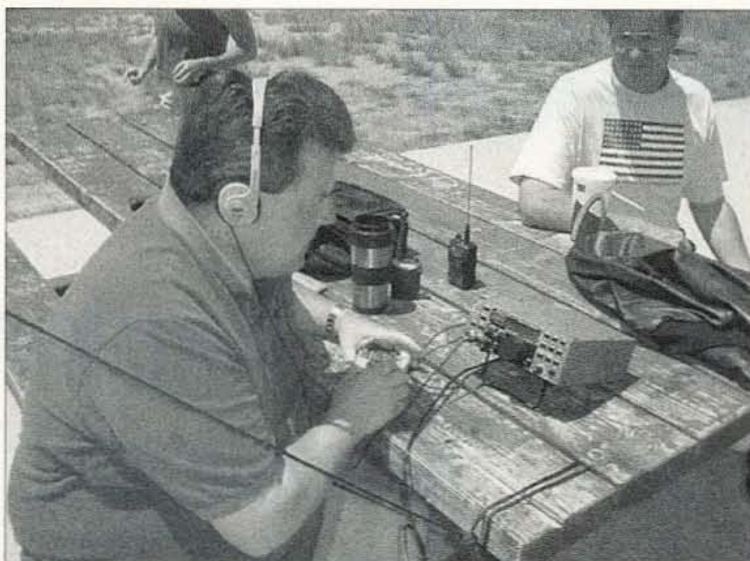
Photo D. A QRP station capable of working the world will fit in a briefcase.
