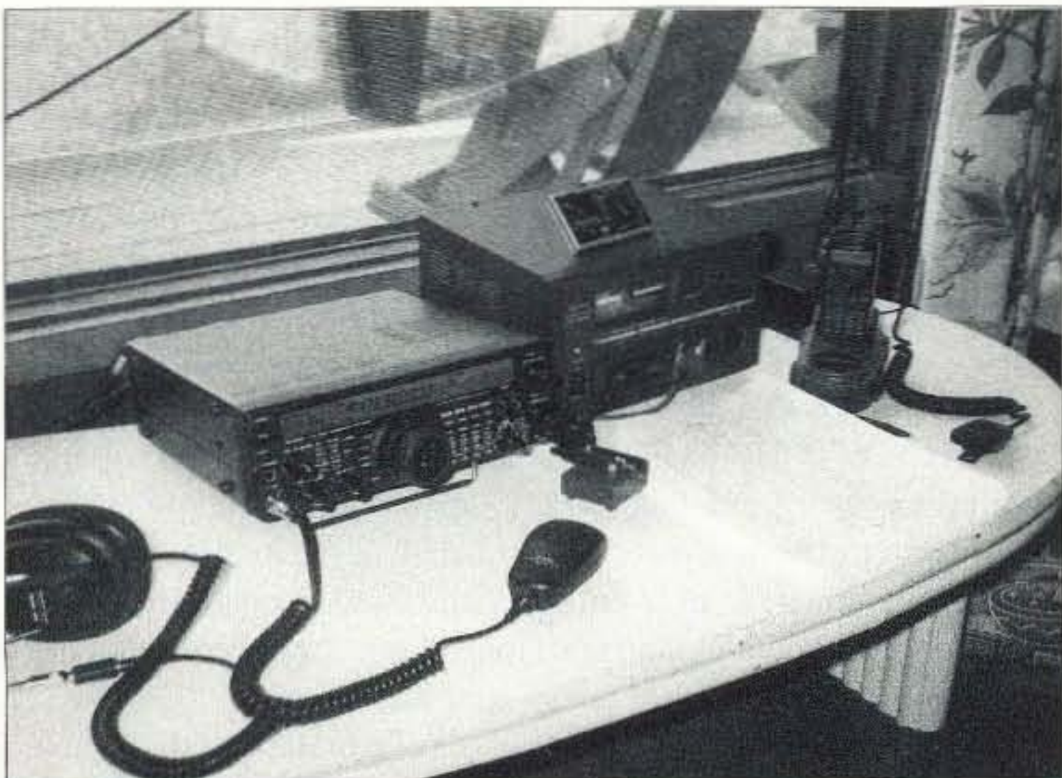
Photo C. A close-up of the Yaesu FT-847 portable station with the FP-1030A power supply and a Whiterook Products Company keyer paddle (Model MK-44).
