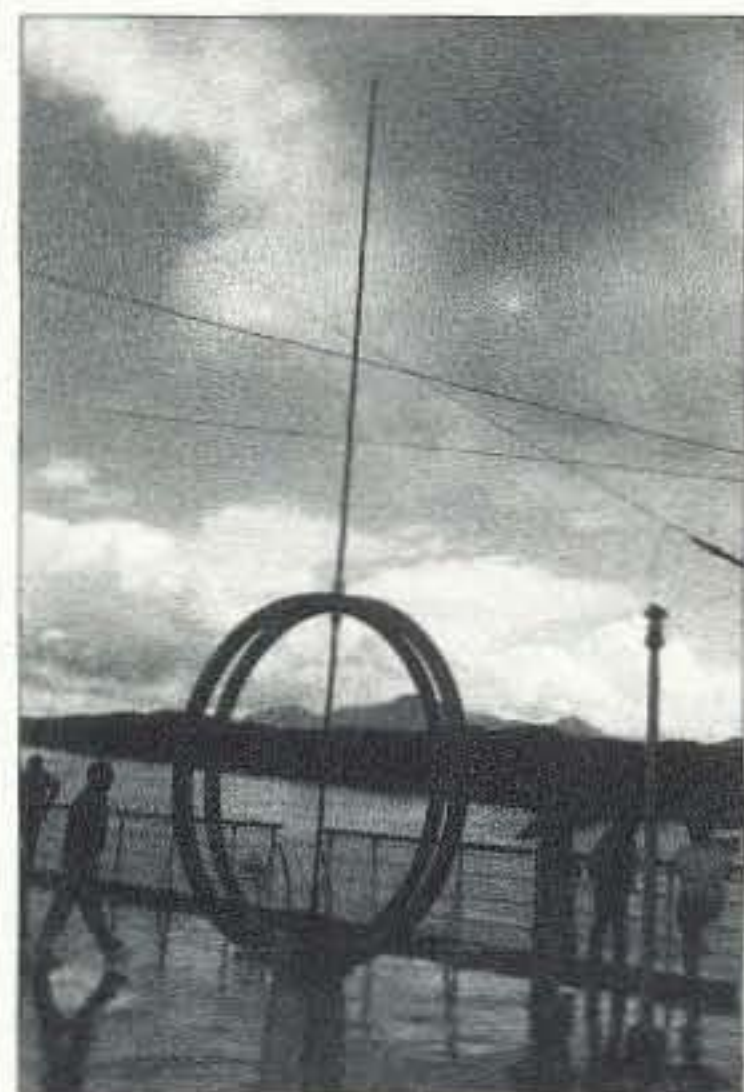
Photo B. Shipboard CW operators aren't required nowadays, but the classic Bellini-Tosi dual-loop RDF antenna is still a common sight on vessels of all sizes.
