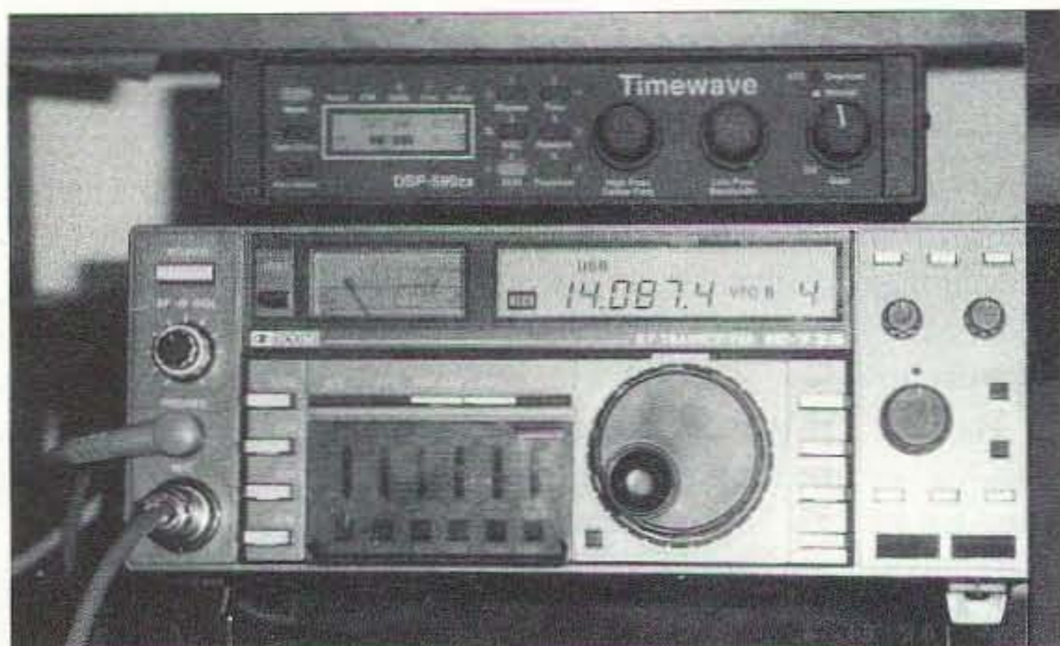
Photo A. The DSP-599zx has a relatively small footprint, about 7-1/2 inches wide. I thought at first the size of the buttons would make operation difficult, but there is plenty of room for me to get to side-by-side buttons to press them simultaneously. The display window keeps you abreast of the many functions and is quite readable from across the operating table.
