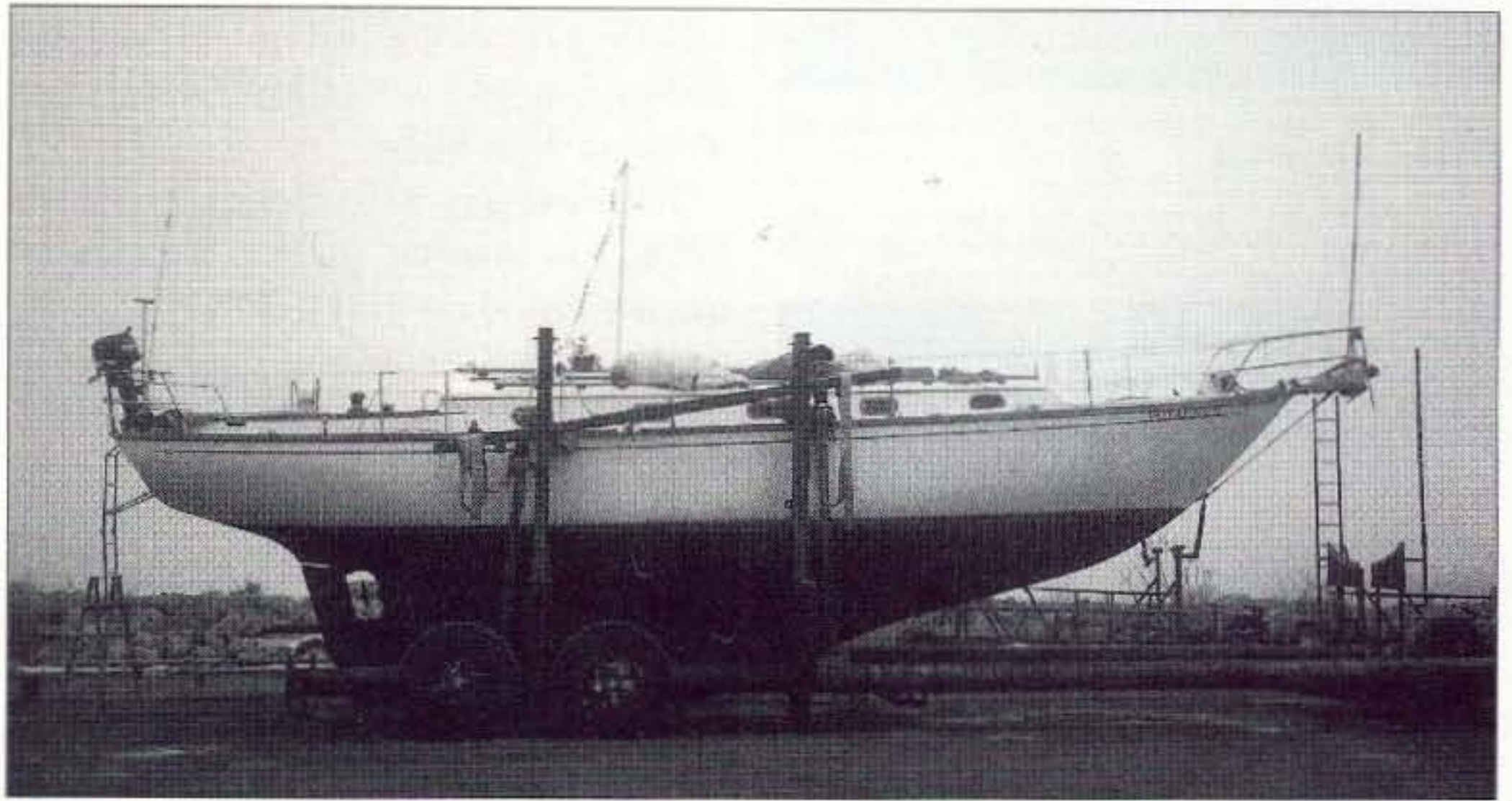
Photo D. Voyageur awaiting the truck. Just visible are the ladderline to dipole on deck and the "Foxhole Antenna" on stern rail.
