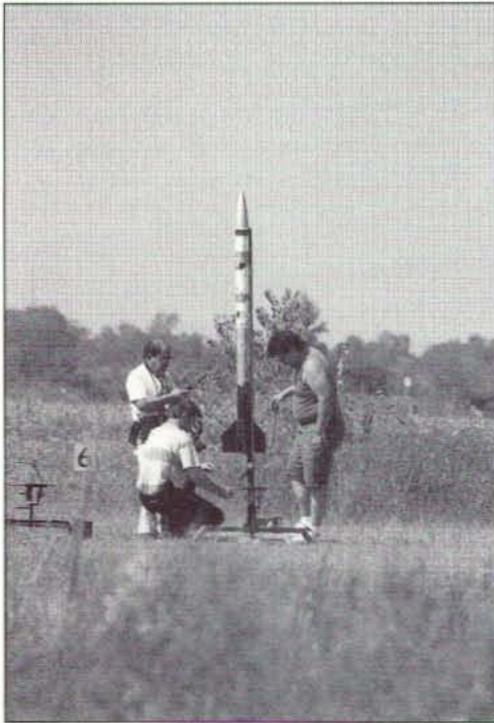
Photo A. The experimental rocket is being prepared for launch. The author inserts the pyrotechnic igniter into the composite motor while two friends check the ATV test transmission. The CCD camera looks through a window below the silver ring underneath the nose cone.
