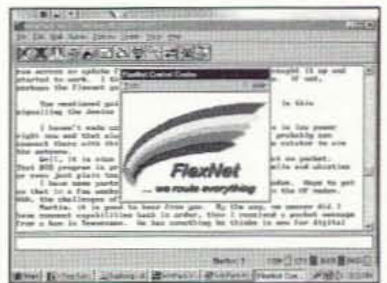
Fig. 1. Screen shot of Winpack software operating with Flexnet running idle in the background. The PC Flexnet pop-up screen is available for special controls and is normally not visible. There appears to be no conflict with other programs when the Flexnet modules are loaded, even when Winpack is active on a Comm port.
