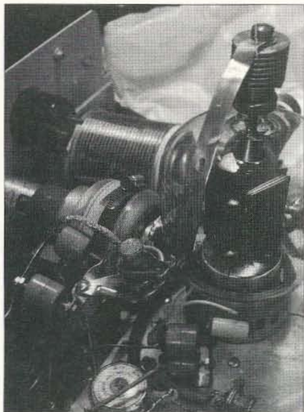
Photo G. The heavy copper strapping from the 4-1000 A plate cap, the plate parasitic choke, door knob supports, and the 8U coax shielding, which directs RF to the tank circuit and plate-tune vacuum variable, have all been dressed in a new coat of silver.
