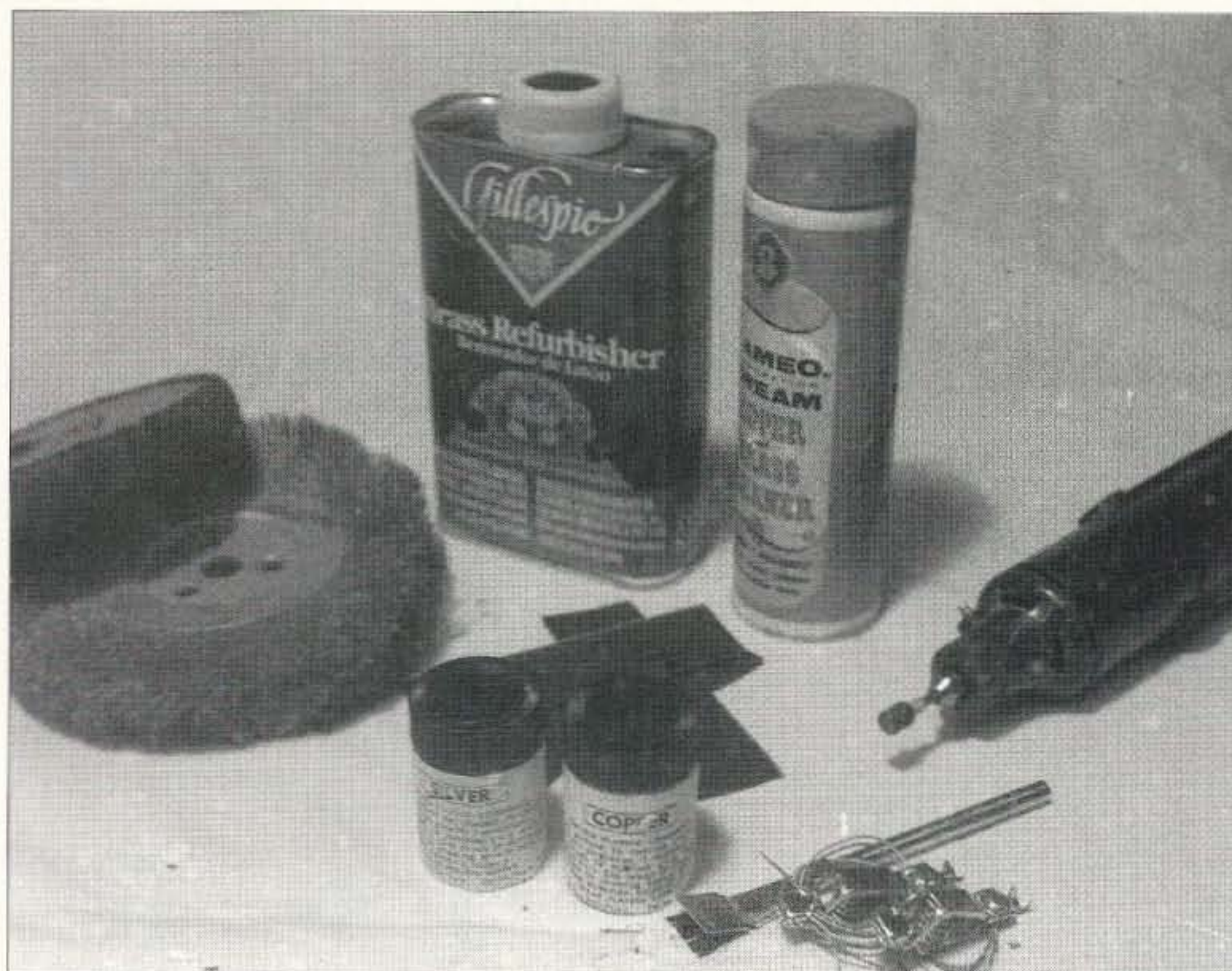
Photo B. Silverplating kit (foreground) containing the jars of silverplating gel, copperplating gel for steel (see text), wire, clips, and plating brush. Note the metal "flap" on the top side of the brush that presses the bristles to the work being plated and completes the circuit. In the background is an array of chemical and abrasive cleaning materials, a wire-and-fabric abrasive wheel, emery cloth strips, and the optional Dremel tool for polishing those difficult-to-reach places.
