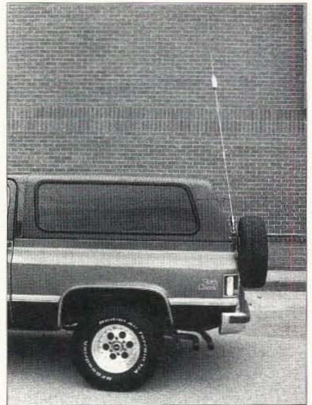
Photo A. Truck with 40-meter Hustler mobile whip. Loop not visible, inside.
