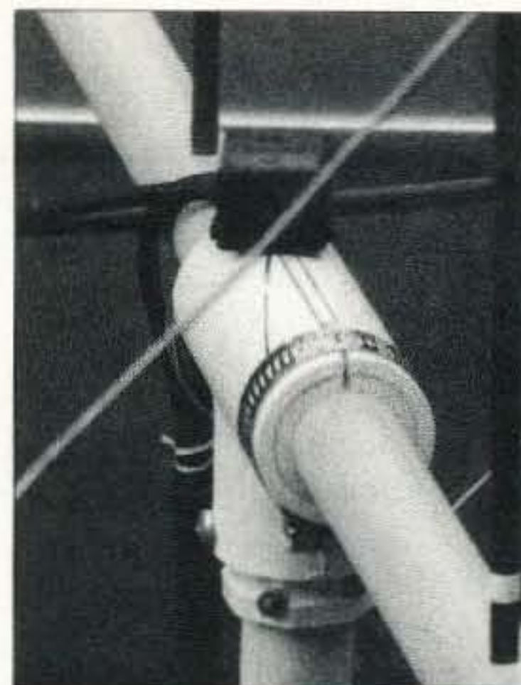
Photo D. I attached the sensor module to the top of the Cubex quad boom. Before mounting, I marked a line at exactly +15 degrees from the boom axis. I then aligned the sensor with the line to compensate for magnetic declination.
