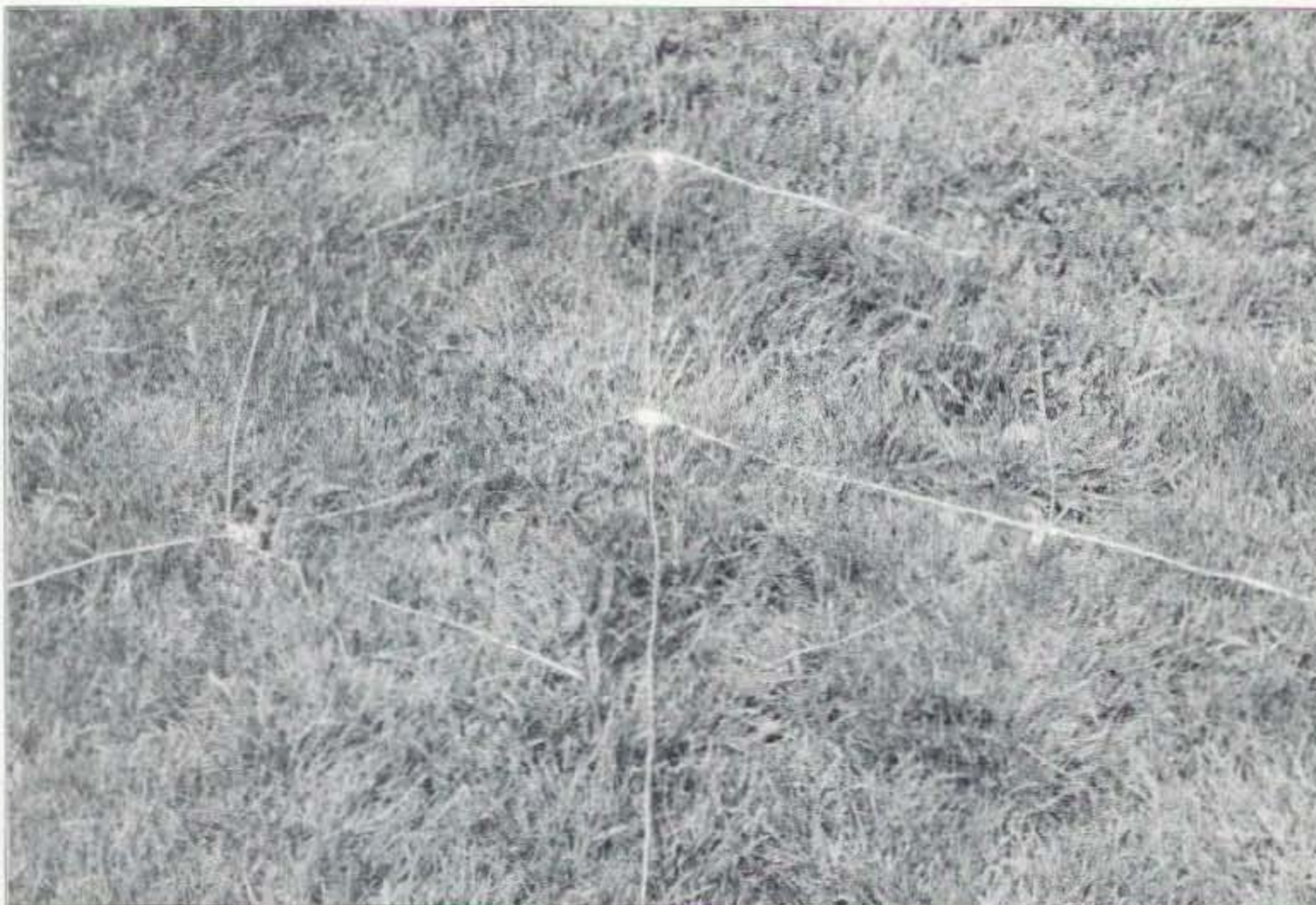
Photo A. The author's 20m version of a fractal counterpoise; like a spiderweb, it's not as fragile as it appears.
