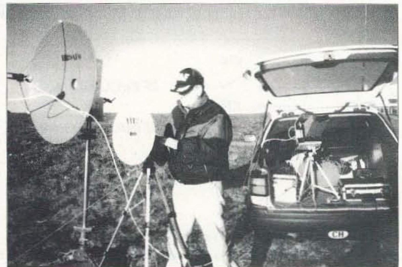
Photo A. Michel Vonlanthen HB9AFO successfully completes a two-way 10 GHz ATV QSO of 592 km (368 miles) with F1JSR on the island of Corsica on 10 GHz ATV, from his vantage point near Barcelona, Spain.
