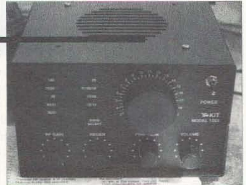
Photo A. You get a lot of controls to play with. There's RF gain, regeneration, main tuning, fine tuning and the volume control.
