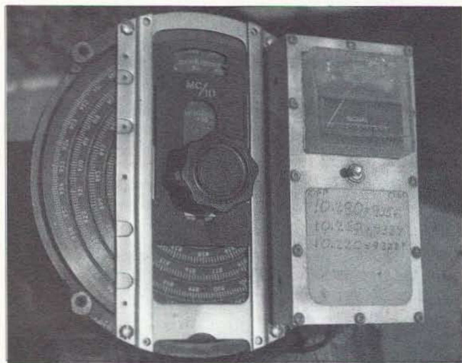
Photo B. Surplus waveguide frequency wavemeter with amplifier and meter indicator attached. The unit had calibration readings noted for 10.220, 10.250, and 10.280 GHz. It was very useful when using simple Solfan or burglar alarm type Gunn oscillators for WBFM.
