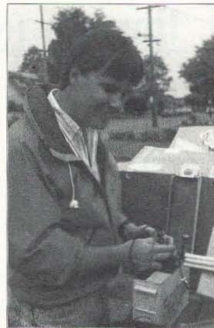
Photo C. Surplus ammunition cans make excellent waterproof fox enclosures. Kevin Kelly N6QAB is preparing this foxbox for the Friendship Radiosport Games.
