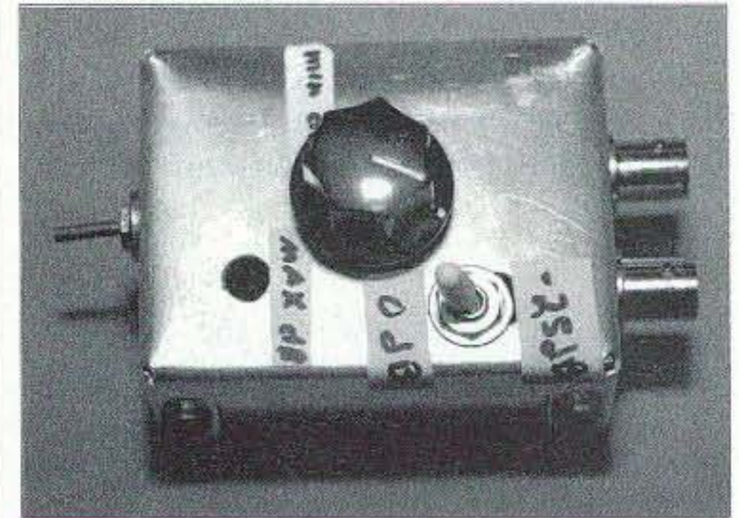
Photo A. Top view of a completed attenuator. (Disregard the hole below the words "MAX dB" ...nobody's perfect.)
