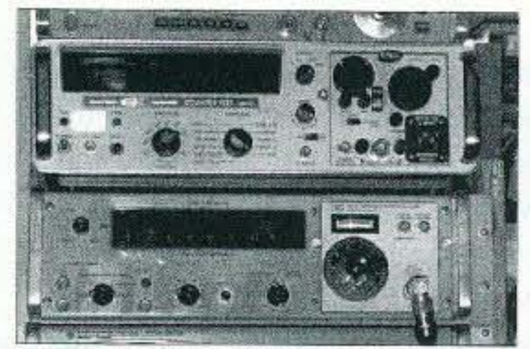
Photo A. Two older HP frequency counters: the Systron Downer 1037 counter with a transfer oscillator that goes to 18 GHz (top unit); and the author's HP-5245 workbench workhorse with a 3 to 12.4 GHz plug-in.
