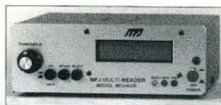
Photo B. The MFJ Multi-Reader, a little box that decodes a plethora of digital modes.
