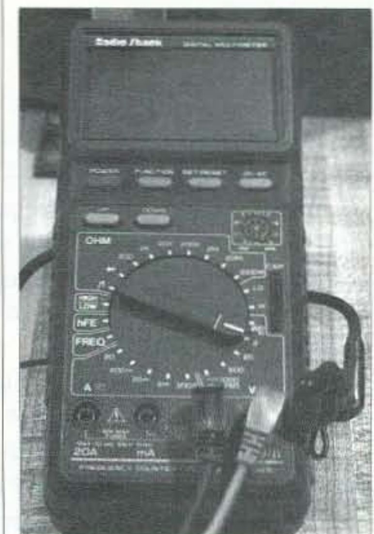
Photo B. Radio Shack computer-interface digital multimeter.
