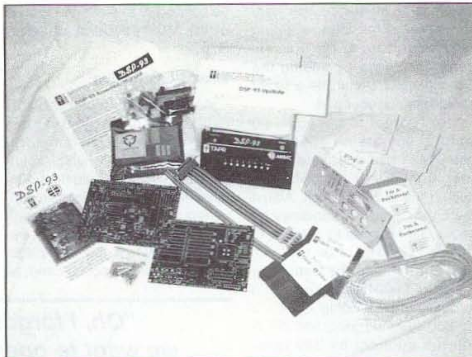
Photo A. The DSP-93 modem kit from TAPR includes all parts, circuit boards, cables, connectors, case, and instructions.
