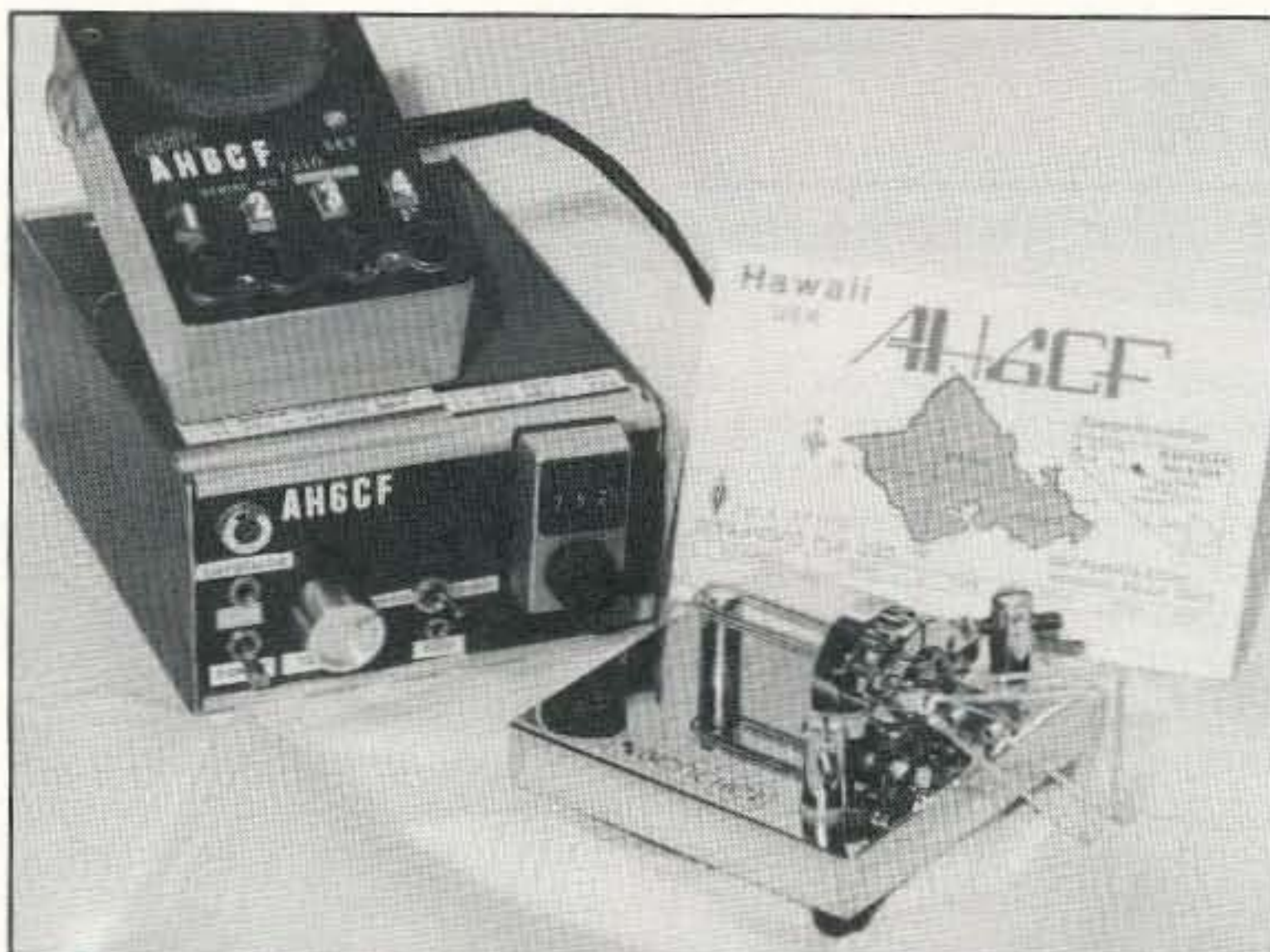
Photo A. Here is AH6CF's version of Dave's transceiver. Note the multi-turn dial for tuning.
