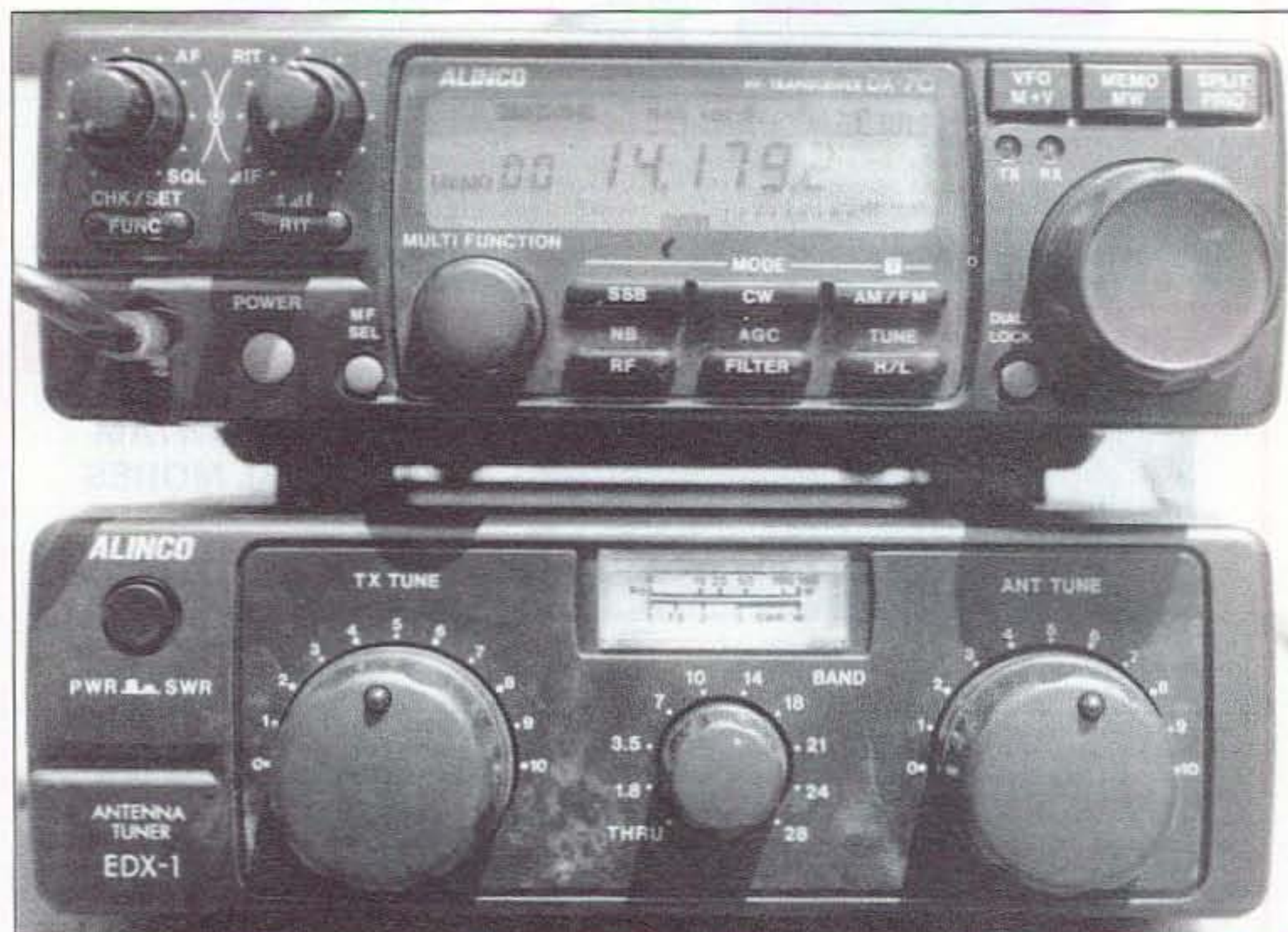
Photo A. The Alinco DX-70 and the matching Alinco Antenna Tuner combine to form a compact "field" radio.
