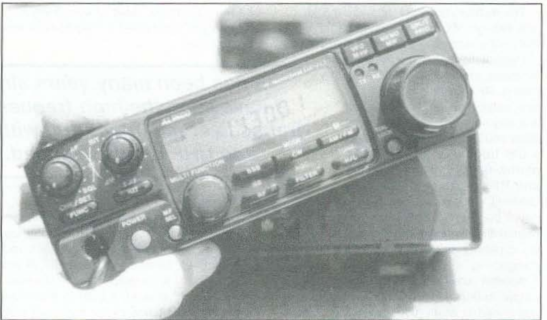
Photo C. The head detaches in 3 seconds for purposes of security.
