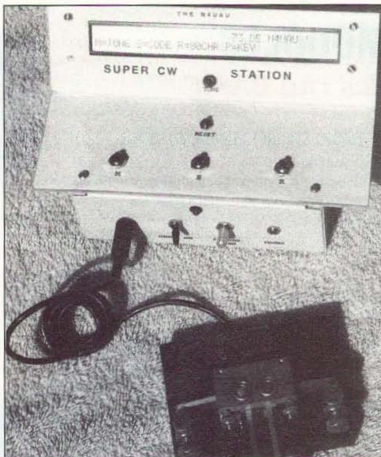
Photo C. The keyer connected to a paddle.
