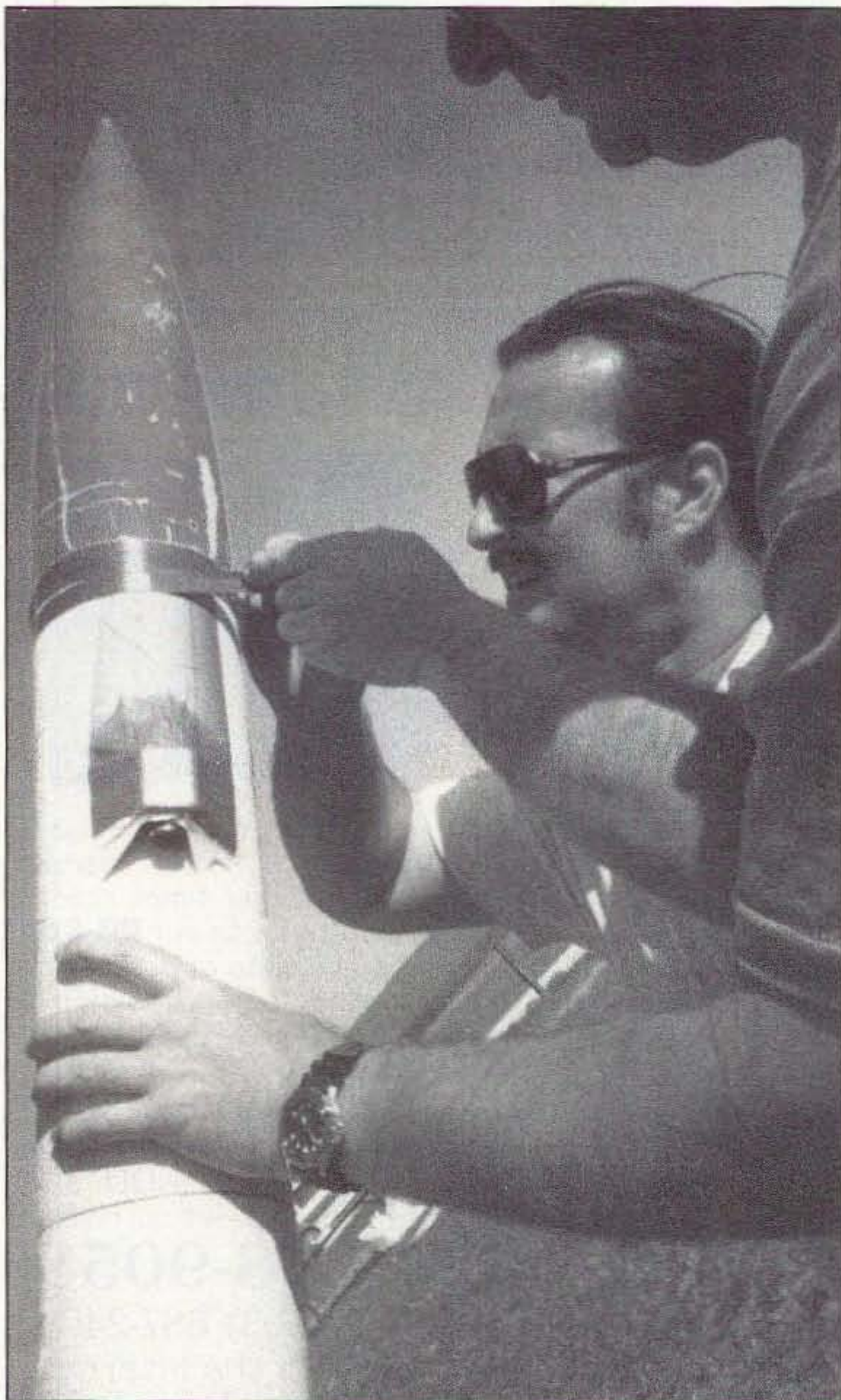
Photo B. Korey Kline puts the finishing touches to the duct tape "cowling" holding the TV camera to the outside of the rocket as Adam Germann braces the fuselage.
