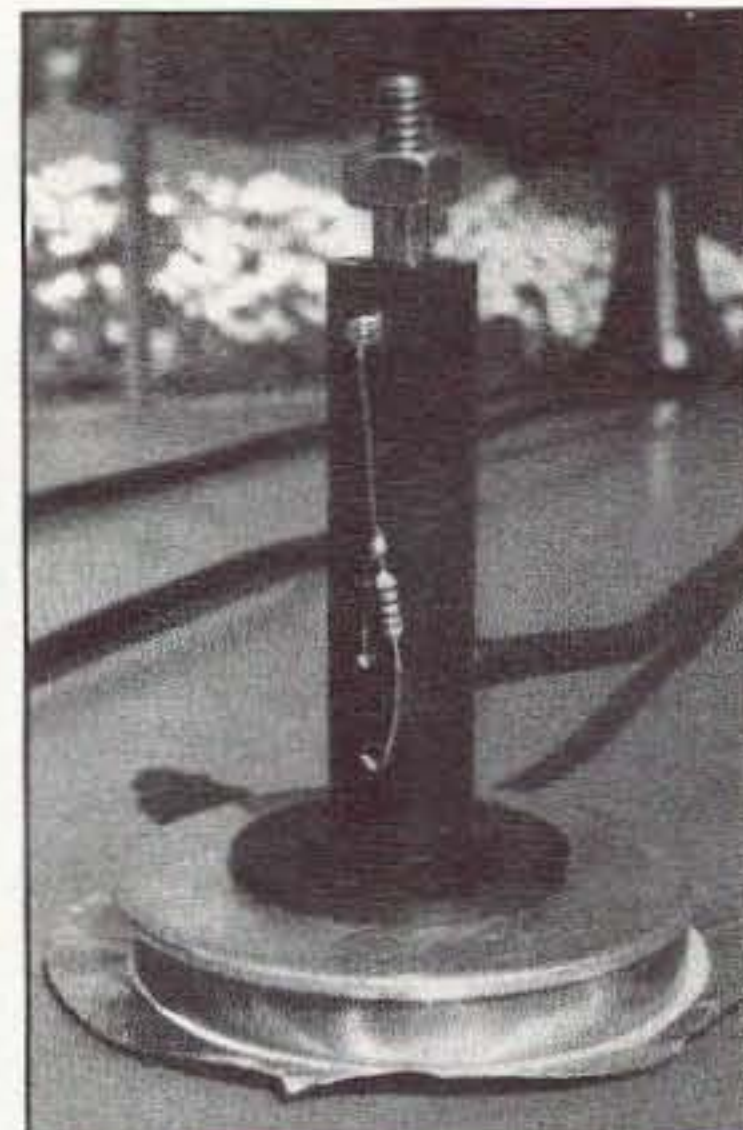
Photo B. The antenna base modified for doppler use. After taking the photo, I added some electrical tape to prevent a short from the PIN diode cathode to the resistor lead.
