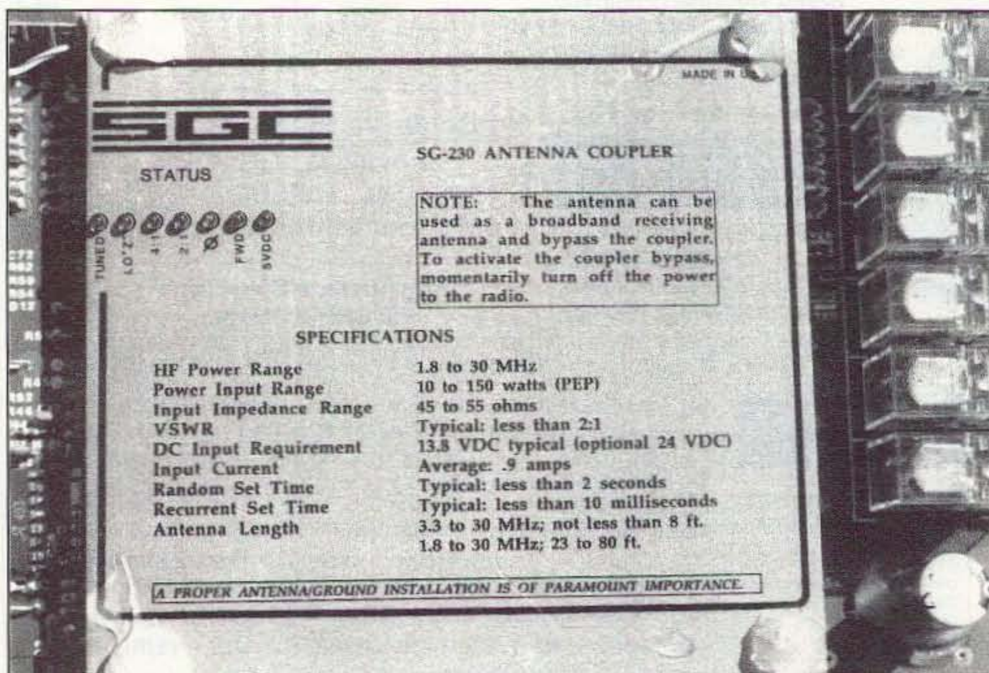
Photo D. Status LEDs on the inside of the tuner confirm that everything is working properly.
