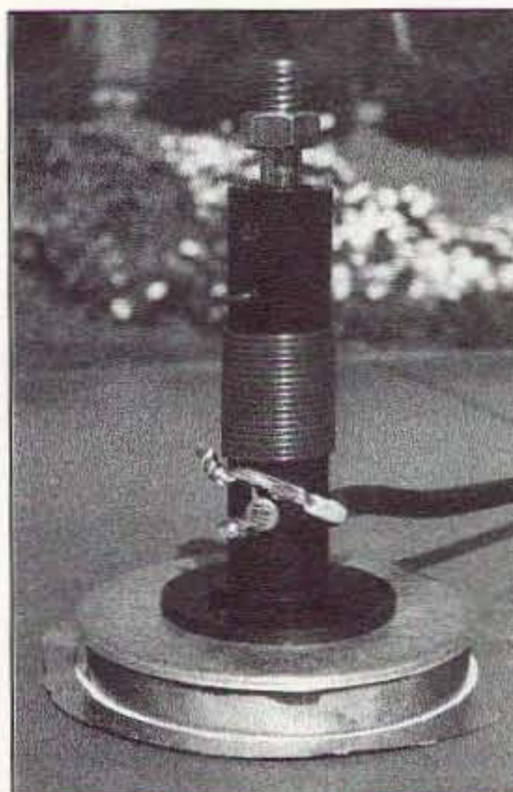
Photo A. Inside the base of the Barjan 11 meter antenna before modification. Note the white insulating paper between the magnet and the bottom foil.
