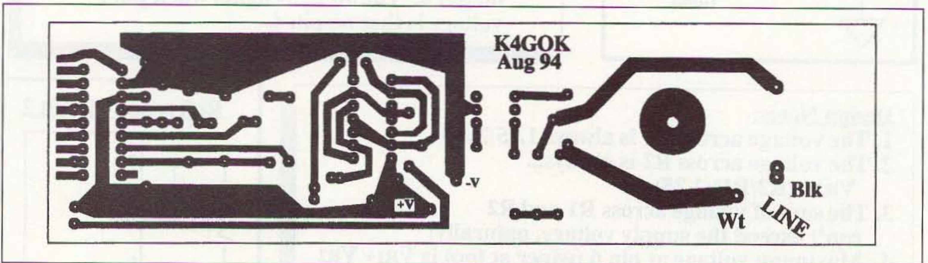
Figure 2. PCB foil pattern (view from copper foil side).
