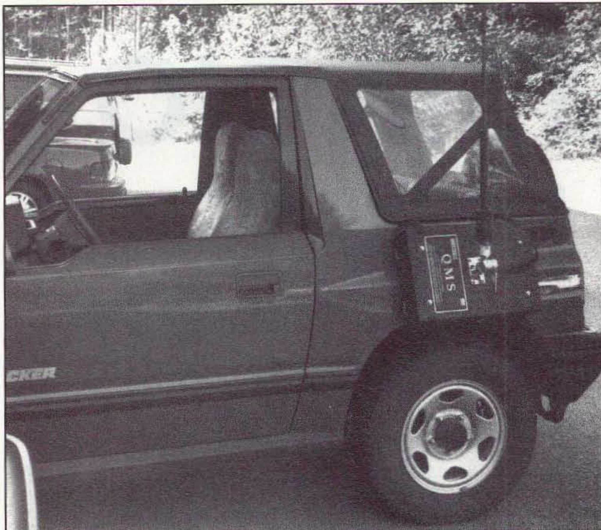
Photo G. The auto-tuner QMS-mounted on an off-the-road vehicle.
