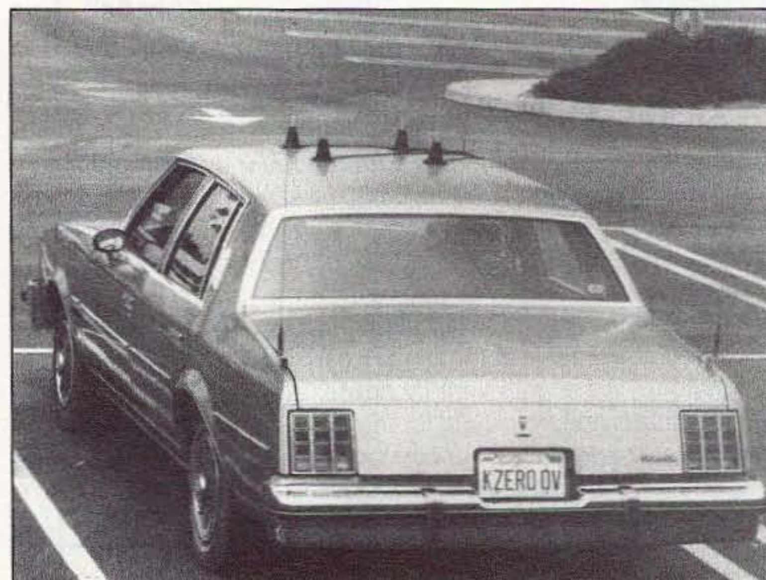
Photo D. Magnetic-mount doppler whips can be placed quickly on any vehicle with a ferrous metal top and moved about to cover a wide range of frequencies. Now my second car has RDF gear on board.
