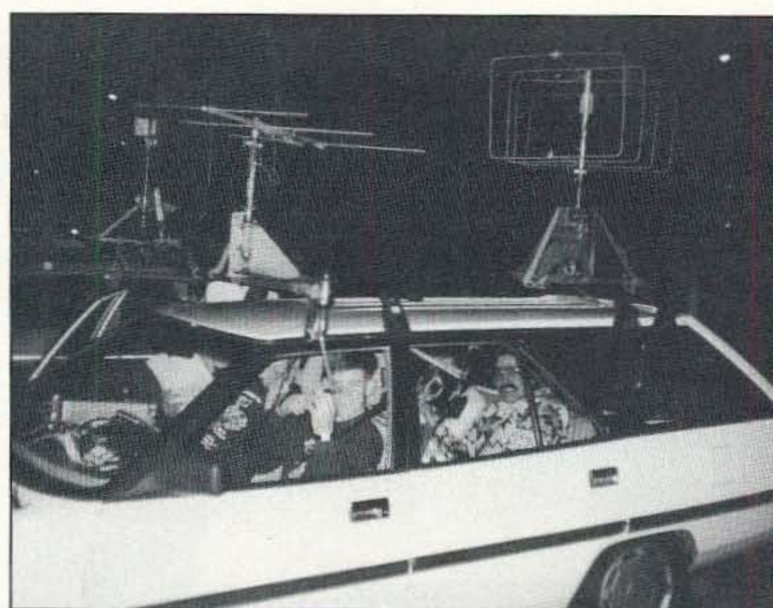
Photo E. A chain drive controls the horizontally-polarized beam for the VK3YQN team. They also have a motorized spinning quad and CRT display in back.
