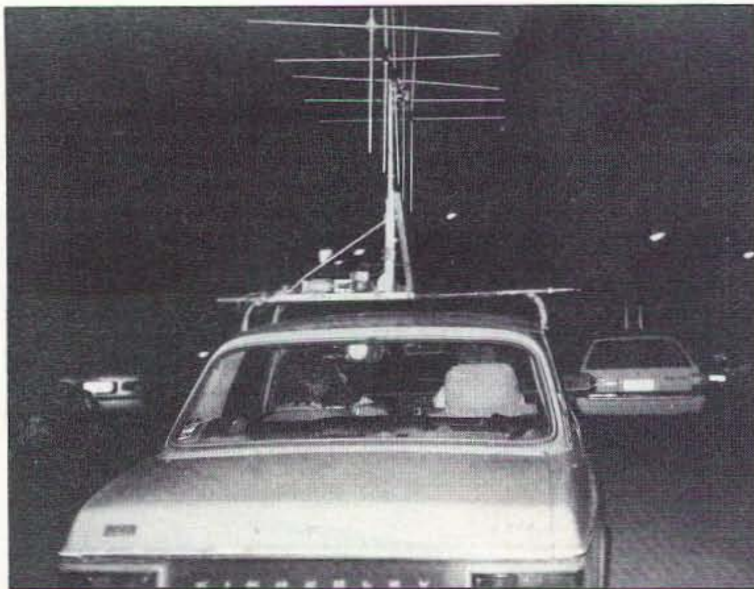
Photo F. VK3XAJ heads down the road with his 10-element dual-polarized beam on the roof and scope-tube display in the back seat. "He gets lots of attention from the police," says Mark.
