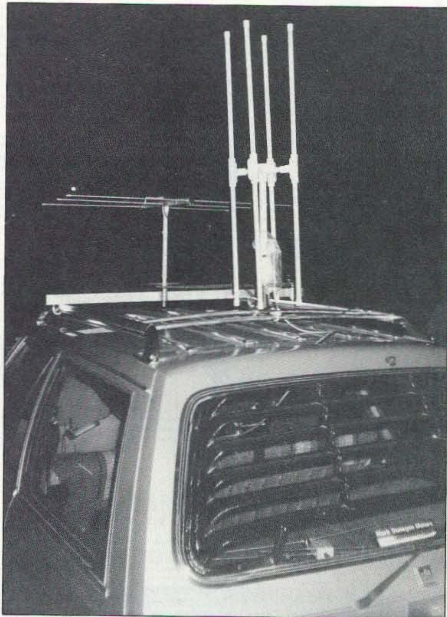
Photo C. The VK3GMZ team hunts on 2 meters with both a horizontally-polarized beam and a modified marine Doppler array.
