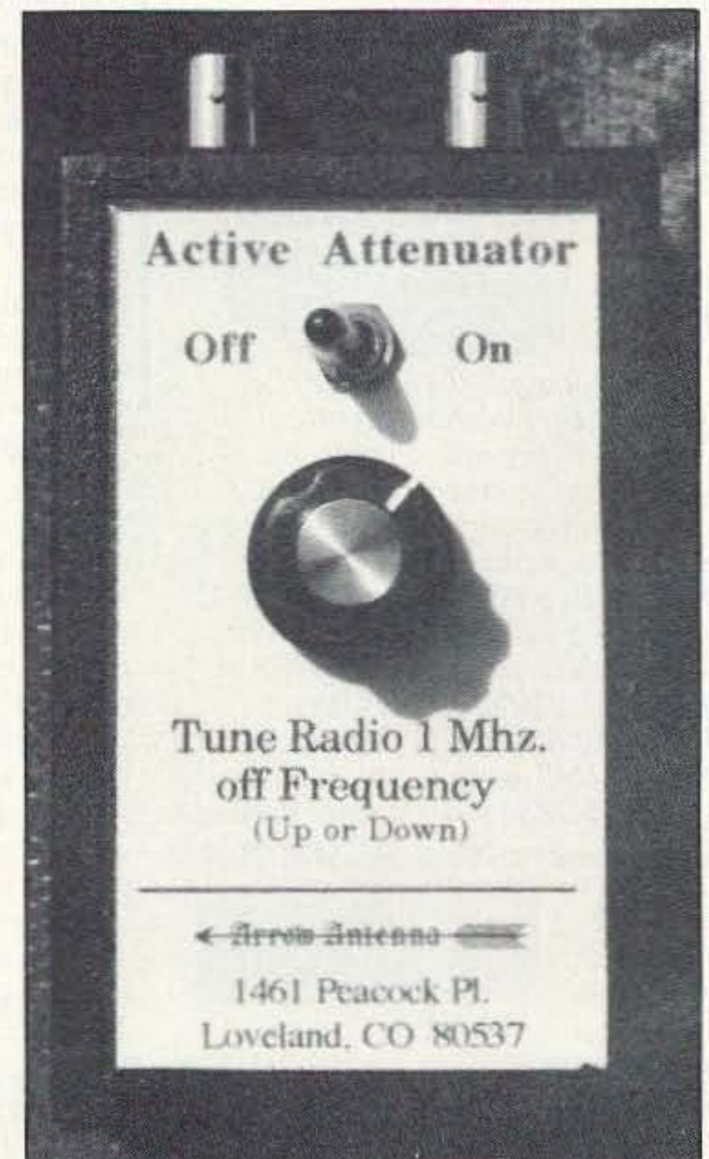
Photo C. The Arrow Antenna offset attenuator is in a 2-3/8" x 3-3/4" x 1" plastic box.
