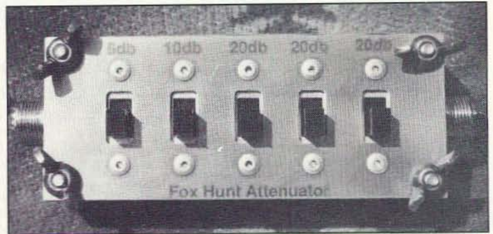
Photo A. You can build your own resistive attenuator from PC board material, switches, and resistors. Or you can buy a finished unit like this from Arrow Antenna. Its copper-clad case measures 2" x 4-3/4" x 1-1/4".
