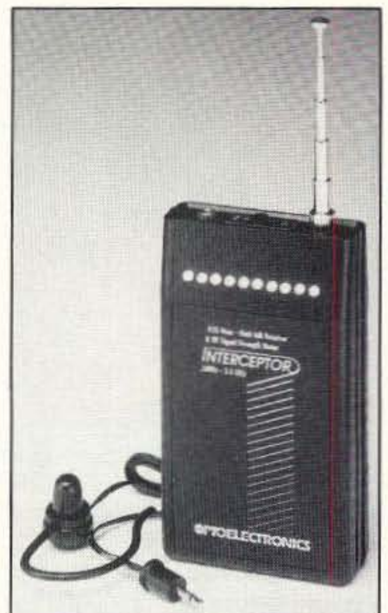
Photo A. At 4.1" x 2.4" x 0.8", the Optoelectronics model R20 field-strength meter fits into a shirt pocket.
