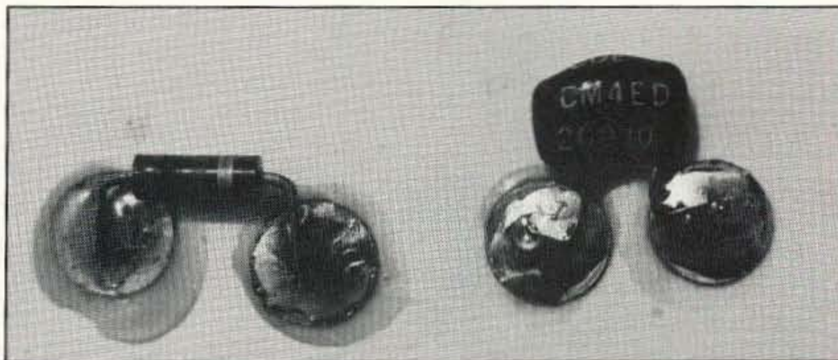
Photo B. A tight-shot of the MSM connection pads.
