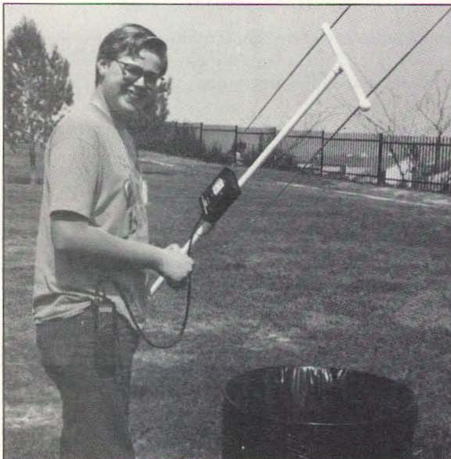
Photo A. Aha! It's in the trashcan! Jason McLaughlin KD6ICZ shows how to "sniff" out a hidden 2 meter transmitter with the Ramsey Foxhound. The unit connects to the antenna and earphone jacks of his handie-talkie.
