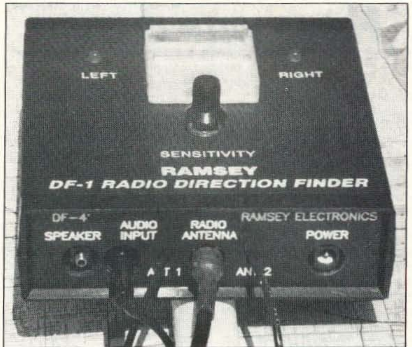
Photo C. The DF-1 circuit board is designed to fit into the optional CDF plastic case. Coax and connector locations on the revised board are different from this original model. It's wise to order the case and board at the same time to be sure they are compatible.
