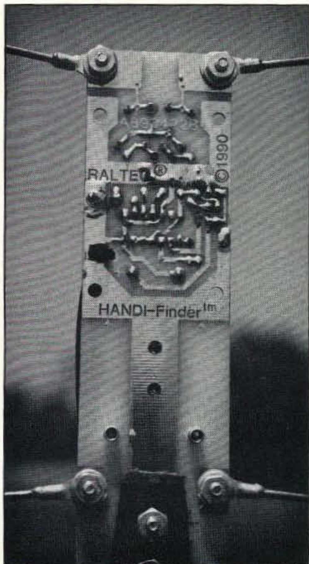
Photo B. The compact, lightweight unit is powered by a 9V battery and mounted on a paint-roller handle.
