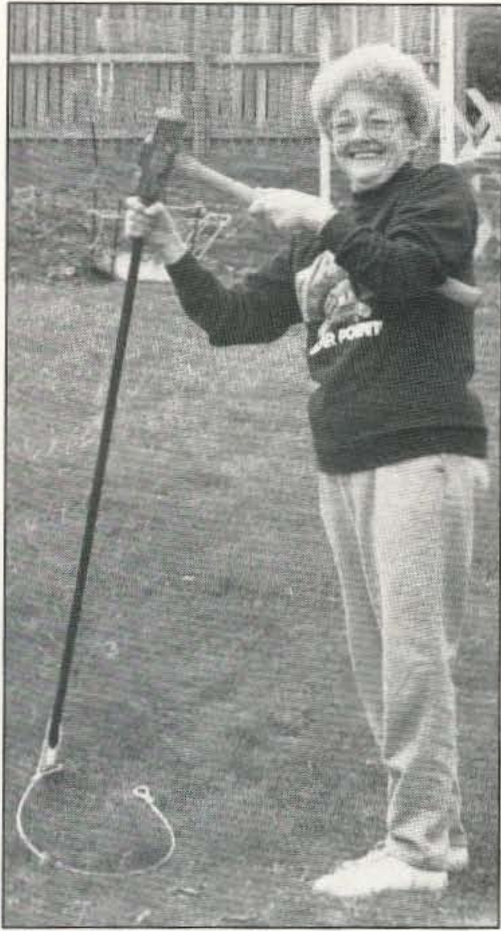
Photo B. The Duckbill can be driven into place with a sledgehammer and the DR-3 drive rod.
