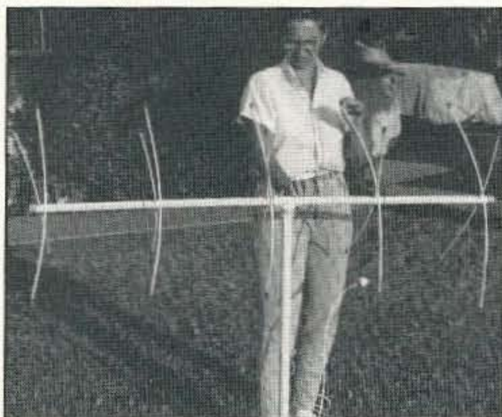
Photo B. The sturdy PVC design keeps the boom from sagging. Be sure to bow all of the spreaders in the same direction.
