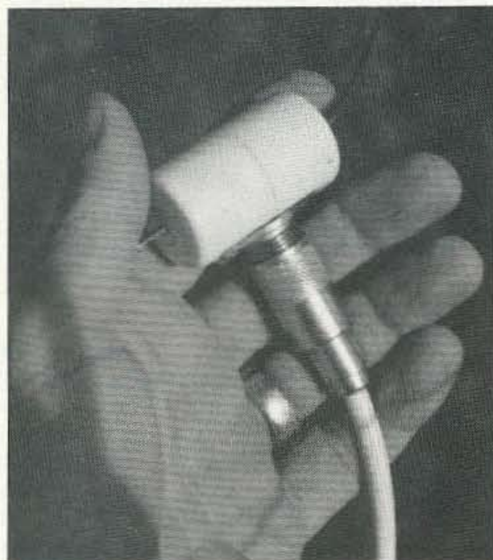
Photo D. Close-up of the feedpoint assembly.
