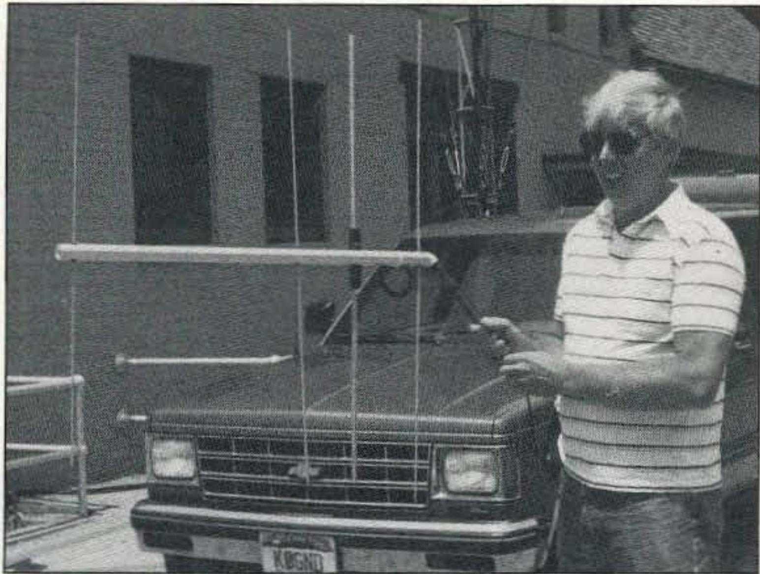
Photo D. Reynolds Davis KØGND says this yagi was carefully designed to have the perfect pattern for sniffing out the fox.
