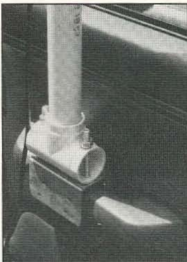
Photo A. Roger Hansen NØLIA came up with this novel idea for an armrest mount. The mast turns freely, but it took some filing to keep the fittings from sticking.
