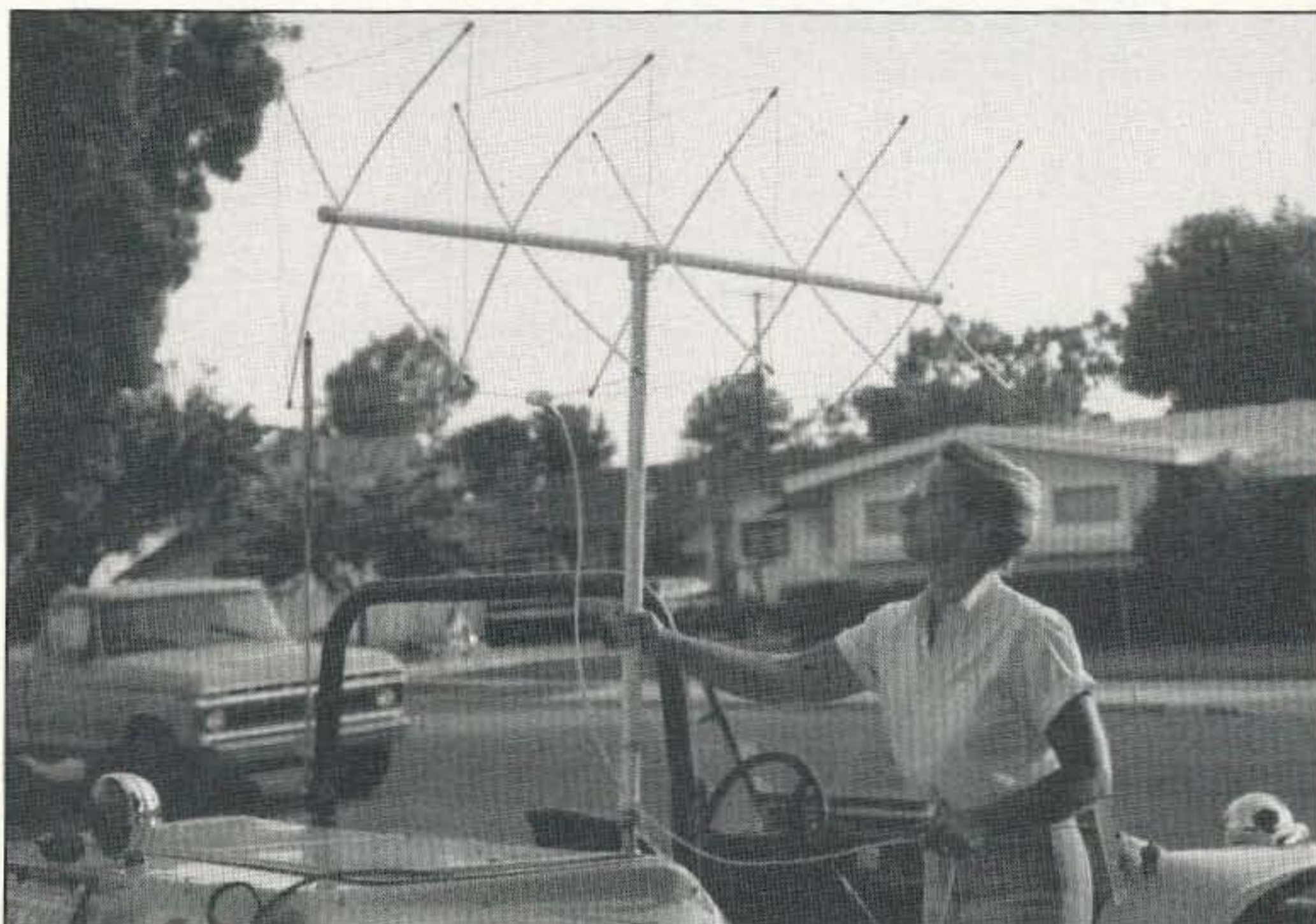
Photo A. The Cellular Security Group's 5-element quad comes complete with a PVC mast.
