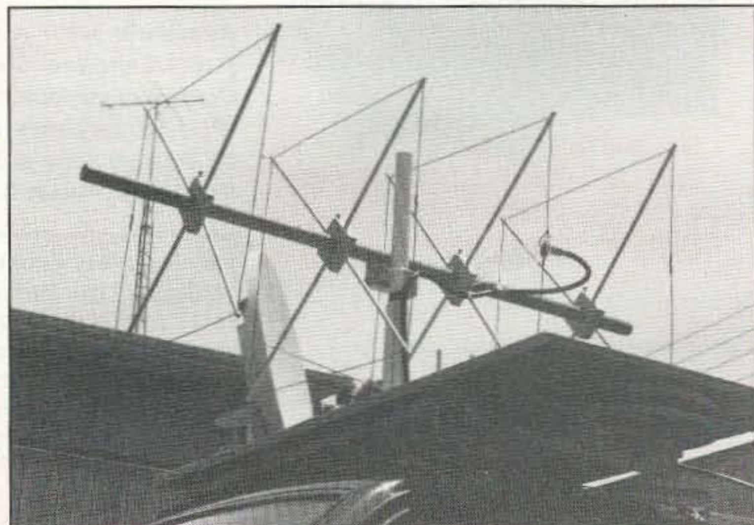
Photo C. Here's a closer look at NØNID's quad. The home-brew belt drive uses a bicycle inner tube.
