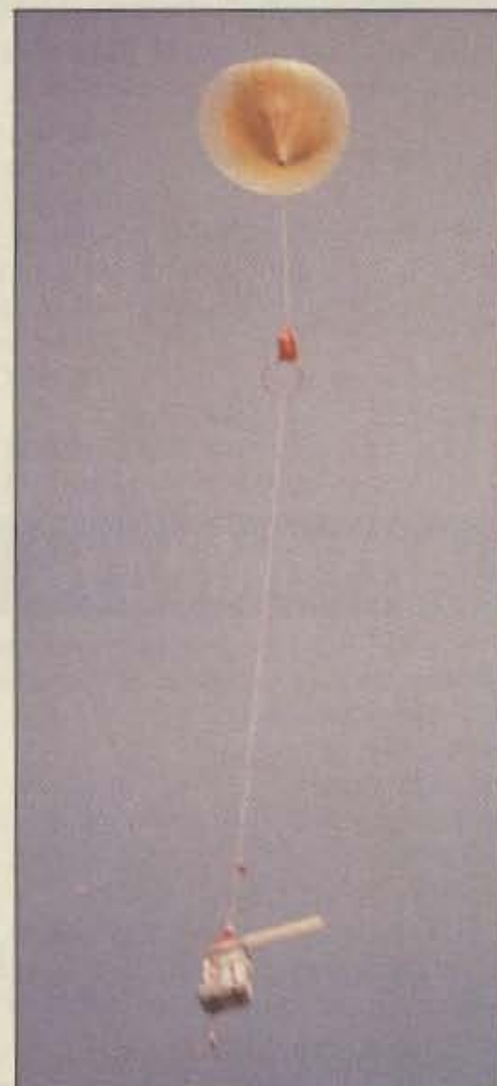
Photo C. A picture perfect takeoff. The balsa wood fin really helped prevent the payload from spinning.
