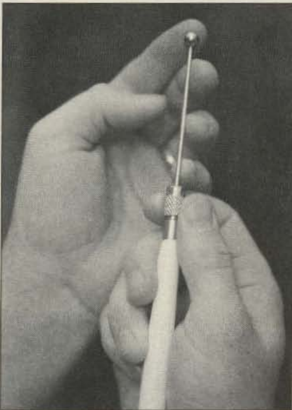
Photo C. The adjustable tip allows for fine-tuning SWR.
