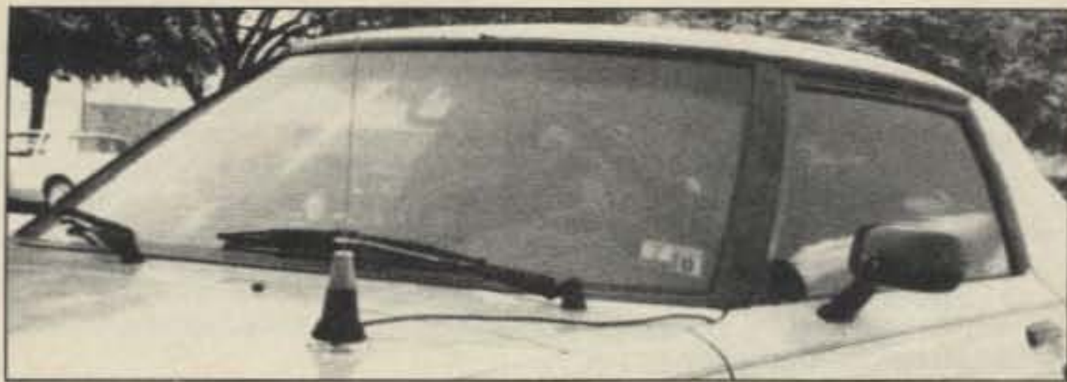
Photo D. For mobile "RS" work, a modified "CB" mag-mount placed away from the 2 meter uplink antenna does an excellent job.
