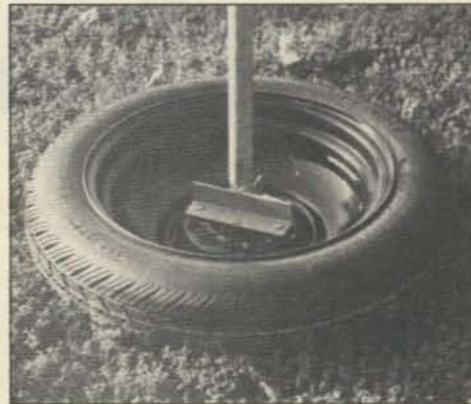
Photo. Once constructed, you can assemble this mobile mount for your antenna in about two minutes! Note that the wheel is positioned brake drum side up.
