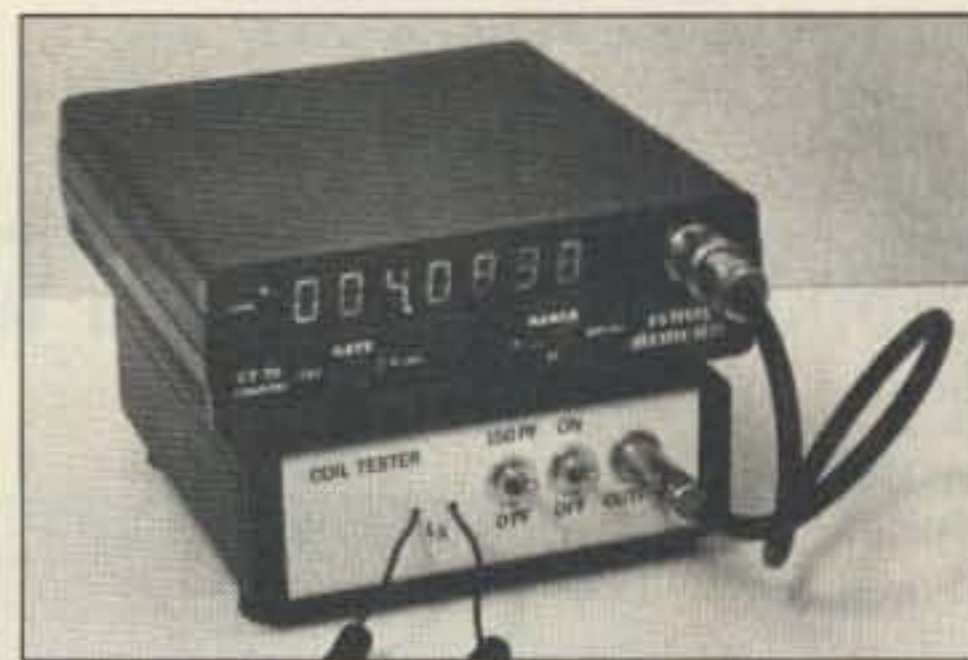
Photo B. The oscillator is housed in an instrument case. Labeling is done with dry transfer lettering on Contact™ self-adhesive plastic. A frequency counter provides the most convenient readout, but you can also use an oscilloscope, dip meter, or communications receiver.
