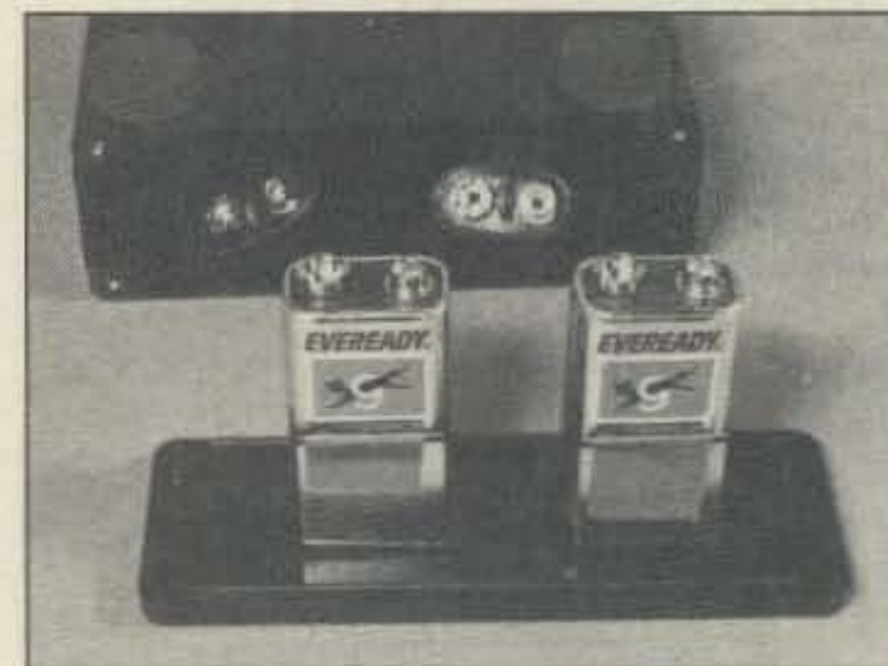
Photo D. Batteries are held by clips on the back panel. Line clips with vinyl tape to keep batteries from slipping out.
