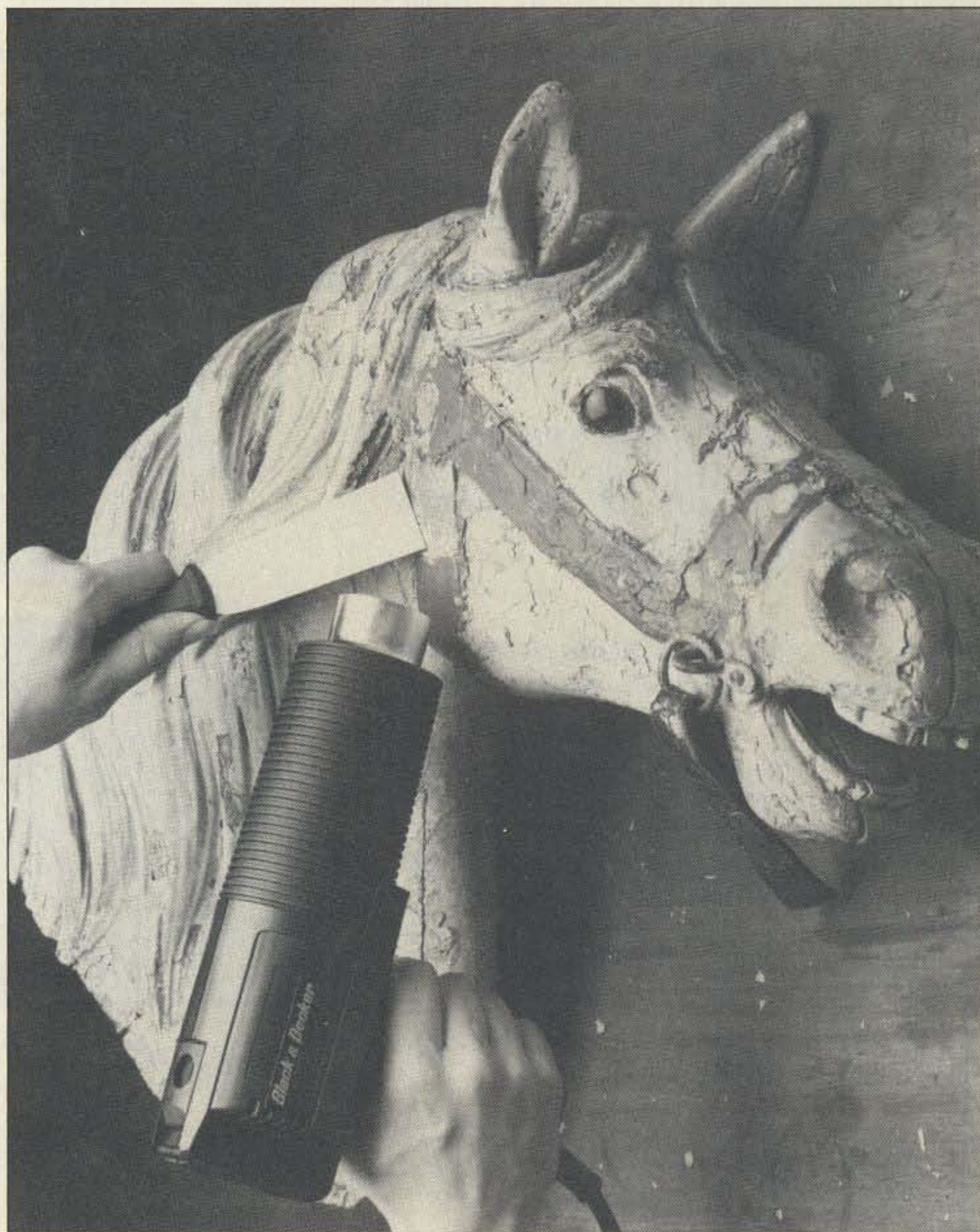
Photo A. The B&W paint stripper gun. Have your own heat guide made at a local metal shop and voila!—a cheap alternative to the industrial heat gun.
