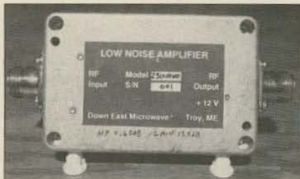
Photo C. The Down East Microwave preamp is a big help in microwave fringe areas.
