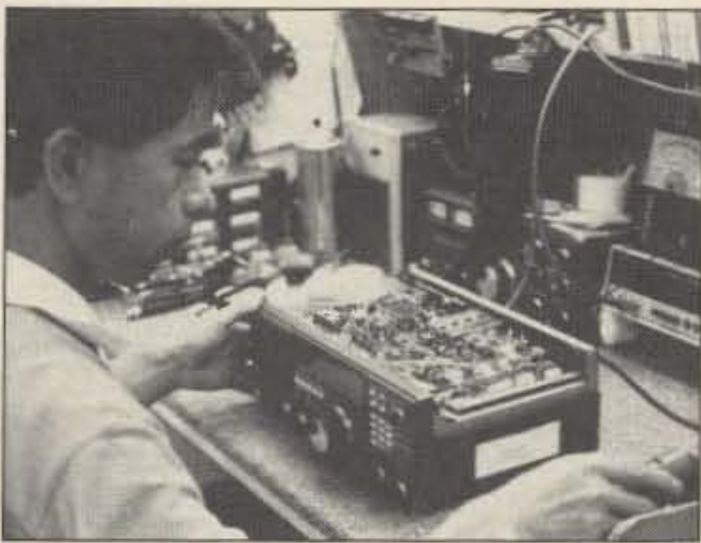
Photo C. Work begins on a base station zapped by lightning. Many lightning-struck rigs are unrepairable.
