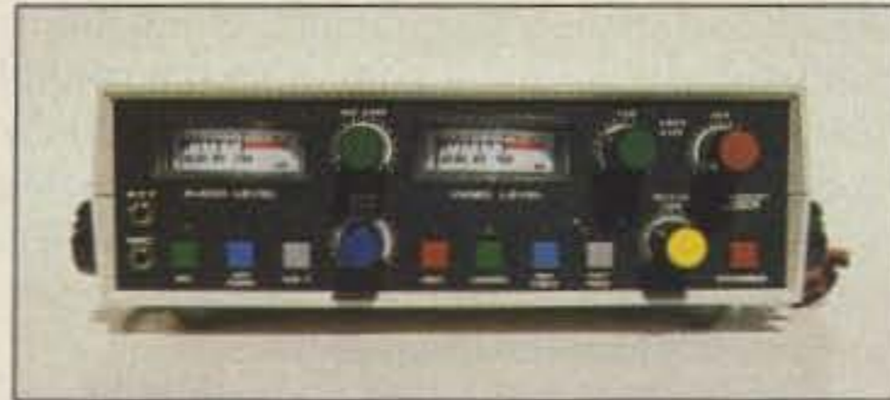
Photo A. The CU-125 control unit is the heart of TDS's ATV gear.
