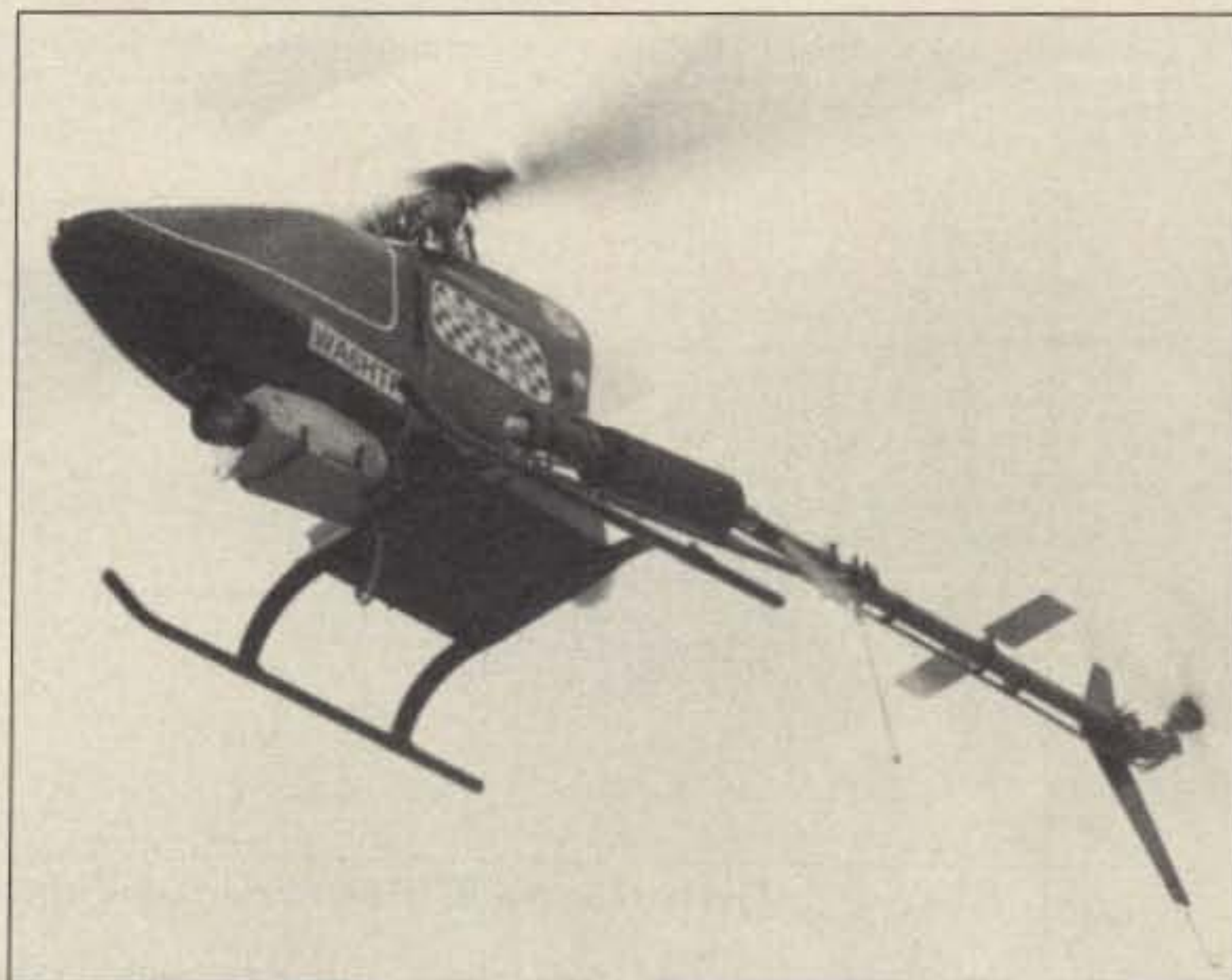
Photo. The six-foot long, 11.5 pound helicopter can go over 60 mph in three dimensions.
