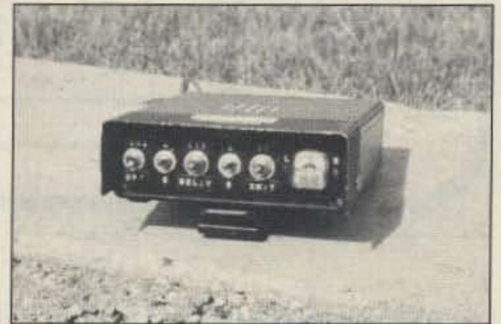
Photo B. The W9DUU DF unit. The earlier model was hand-wired. The new model uses a PCB.
