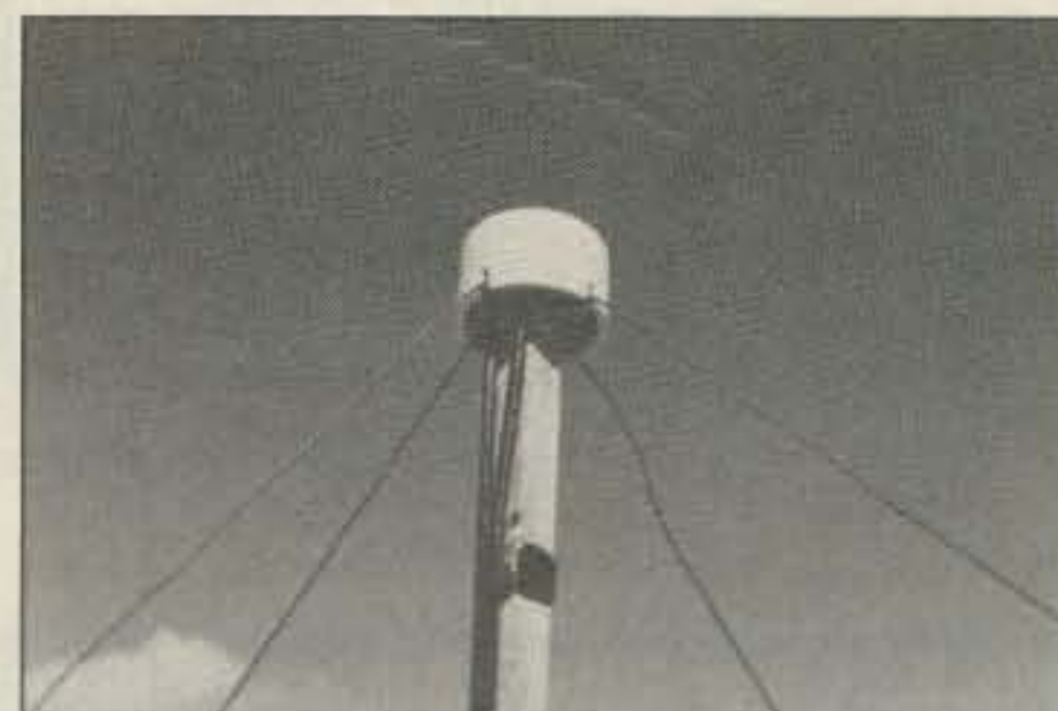
Photo C. Detail of the disc cover on the 10 meter unit.
