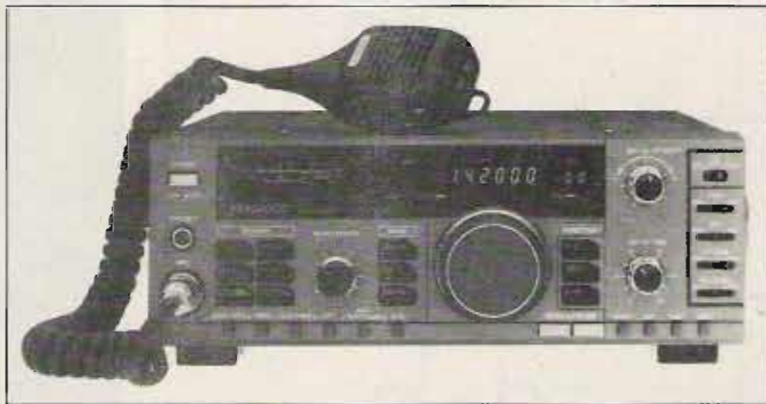
The Kenwood TS-680S. It is a twin to the 140S, with 6 meters and preamp added.
