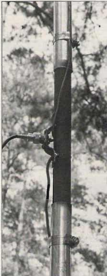
Feedpoint of the Safari Special vertical dipole. The wooden dowel has been painted to protect it from the weather.
