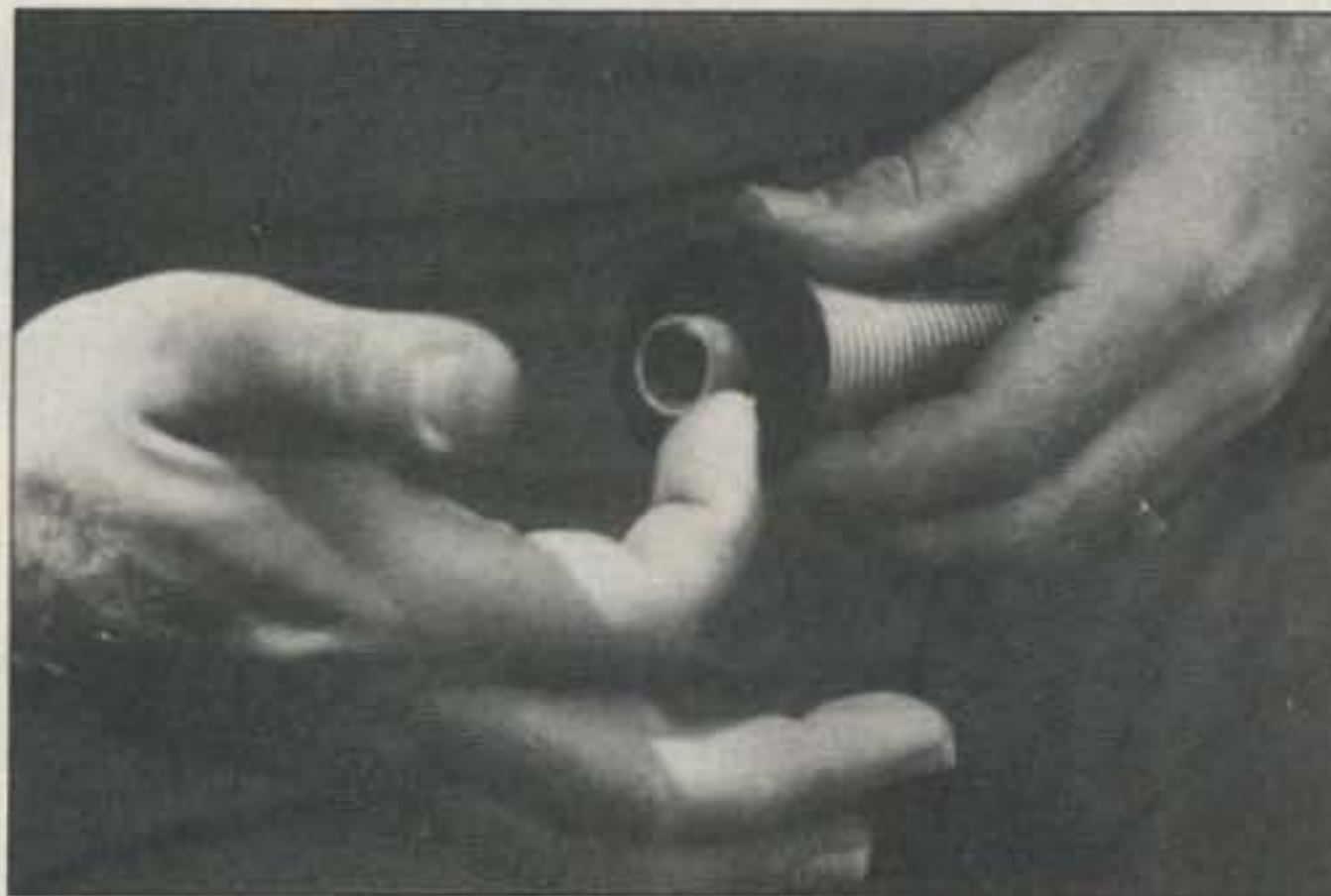
Photo C. Charles N4DKE insisted we put Penetrox not only on the aluminum parts, but everywhere there was metal-to-metal contact. [Photo by author.]
