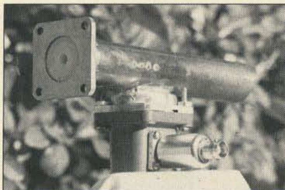
Photo A. Rear view of polaplexer showing Teflon™ transformer and four brass pins on the side of a 1" tube. Detector mounted on polaplexer.
