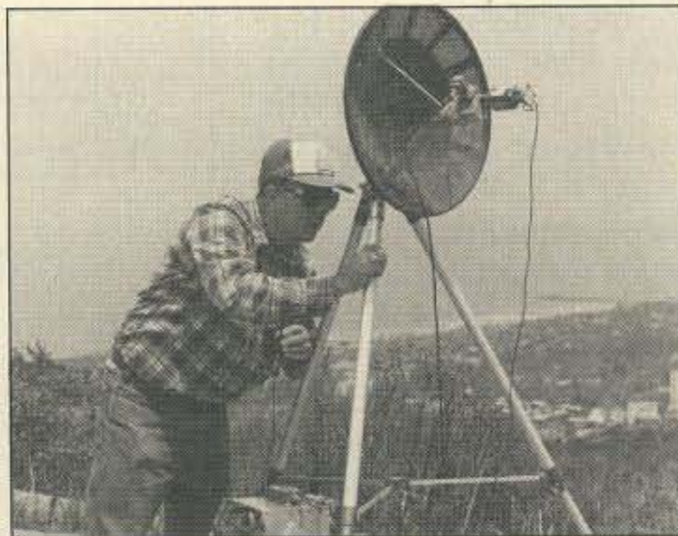
Photo D. Ed W6OYJ on Mt. Soledad, using the polaplexer, Solfan Gunn oscillator, and home-brew 30 MHz receiver. Ed is looking through a bore-sight tube mounted on the dish.
