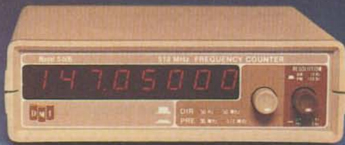
50 Hz to 512 MHz 5 1/2 X 5 X 1 1/2 1 PPM ACCURACY TCXO
