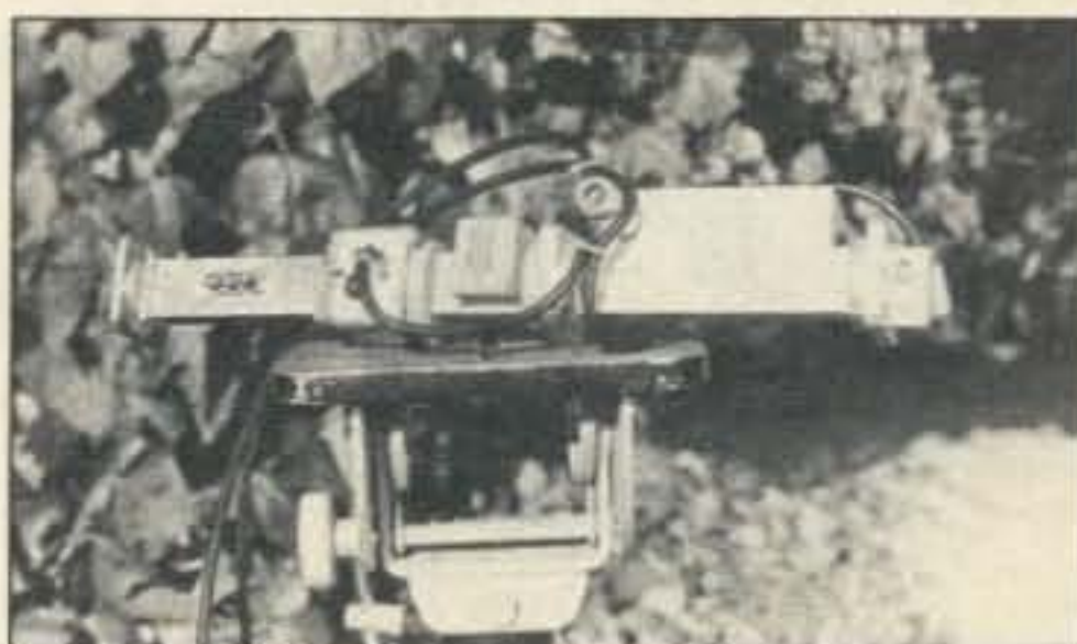
Photo C. 20 dB directional coupler CG-176 mounted between my Gunn oscillator and magnetic isolator. Forward (left) is the detector mount and the three-screw matching network.
