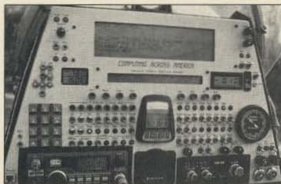
Photo A. The Winnebiko's packet station uses a Pac-Comm Micropower-2 TNC, a Yaesu FT-290 two meter radio, and a Radio Shack Model 100 computer with its display an integral part of the bike's console.
