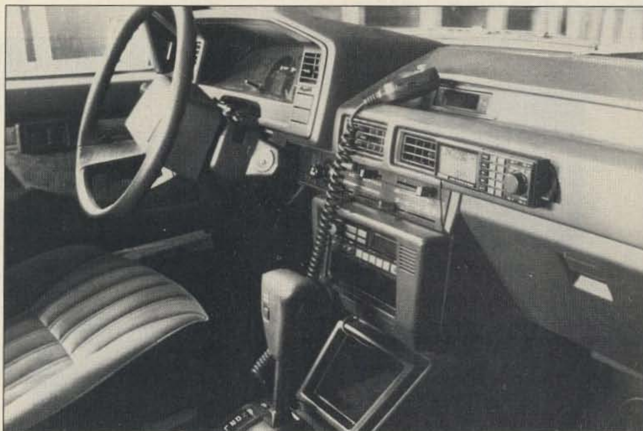
Photo B. Interior view of the 1987 Toyota Corolla LX, showing the IC-900 control head and microphone. The main interface lies underneath the driver's seat. The rest of the system is in the trunk.
