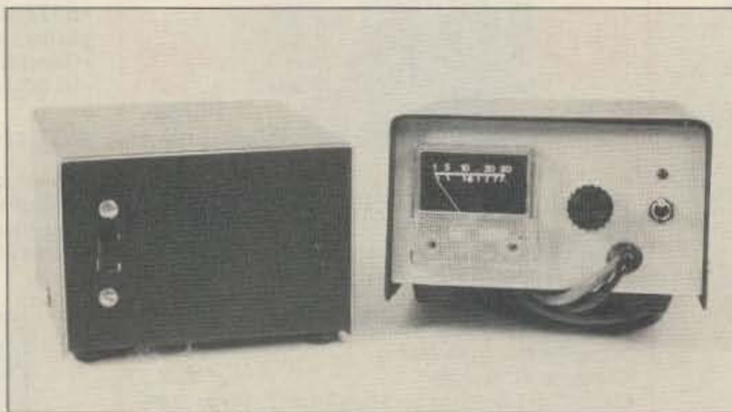
Photo A. This adjustable bench supply and 3A power-pack for a QRP rig are just two of many possible module applications.
