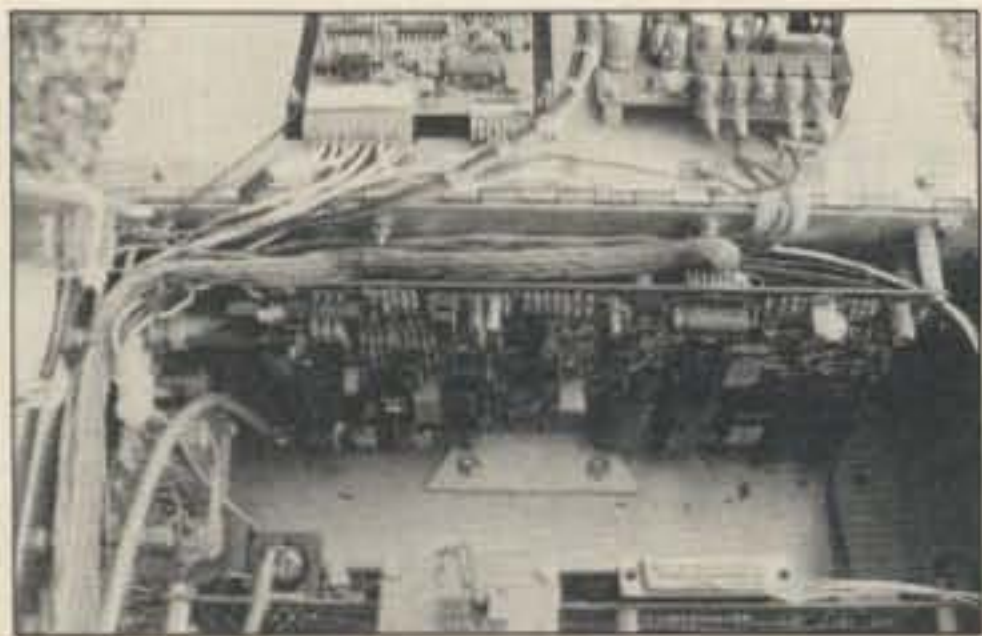
Photo B. The Pac-Comm Micropower-2 TNC, buried deep within the console, actually appears as a node in the serial crossbar network controlled by the bicycle control processor (BCP).
