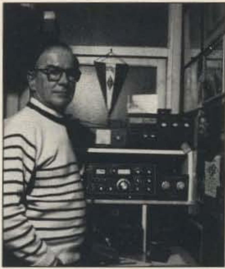
10XXR in his QTH with TS-830S and backup FT-101E . Antenna is TH3 for the HF bands and a quad loop zepplid for the LF bands.
