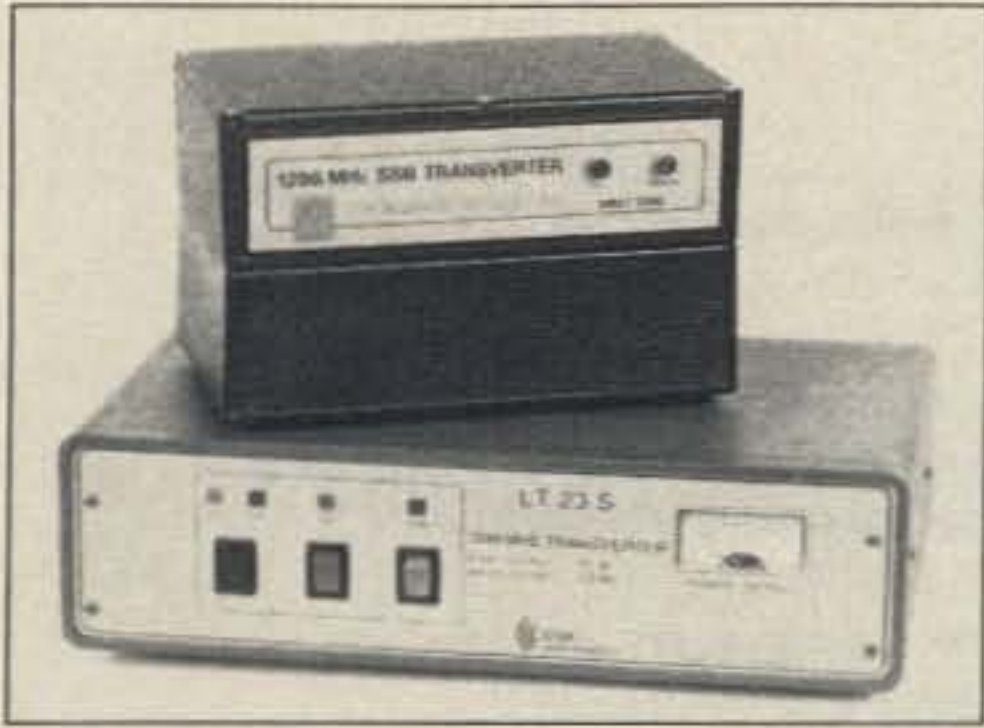
Photo C. Two transverters for 23 cm, Microwave Modules' MMT 1296/144 (top) and SSB Electronics' LT23S (bottom).
