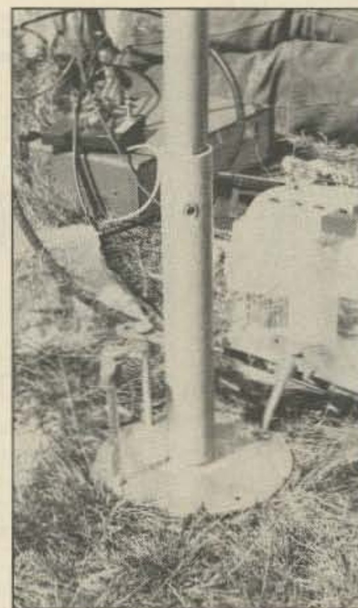
Photo B. The method used to secure the footing of the portable mast arrangement. This saved about 9 pounds from last year's tripod.
