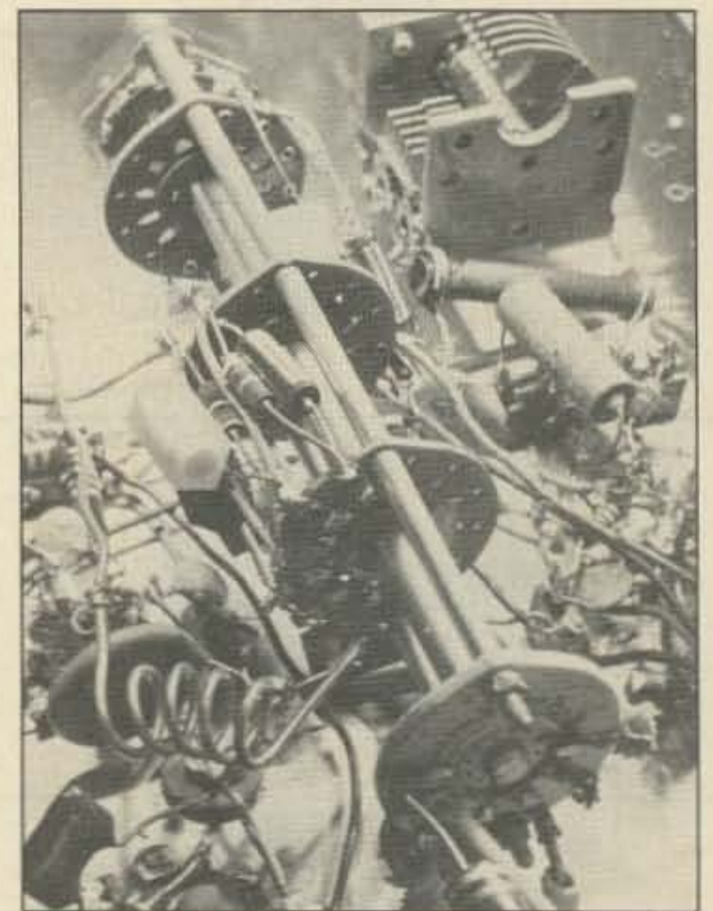
Photo A. Typical medium-power transmitter bandswitch (Allied T-150A) with four gangs or index assemblies (or wafers). The closest gang in the photo is made out of porcelain for the final amplifier. You will need at least a 3/16" screw here. The other thinner phenolic wafers behind this will accept a 1/8" screw. Before obtaining the small 0-80 hardware, check for proper minimum screw length in your own equipment. In addition, perhaps you can use the larger 1-72 or even 2-56 hardware if the wafers and corresponding holes are bigger. Also, the still smaller 00-90 and 000-120 are available. Obtain a catalog!
