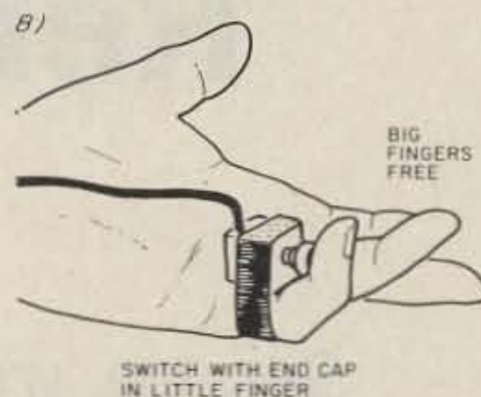
Fig. 7. (a) Remote PTT switch for an HT. (b) The remote switch in action.
