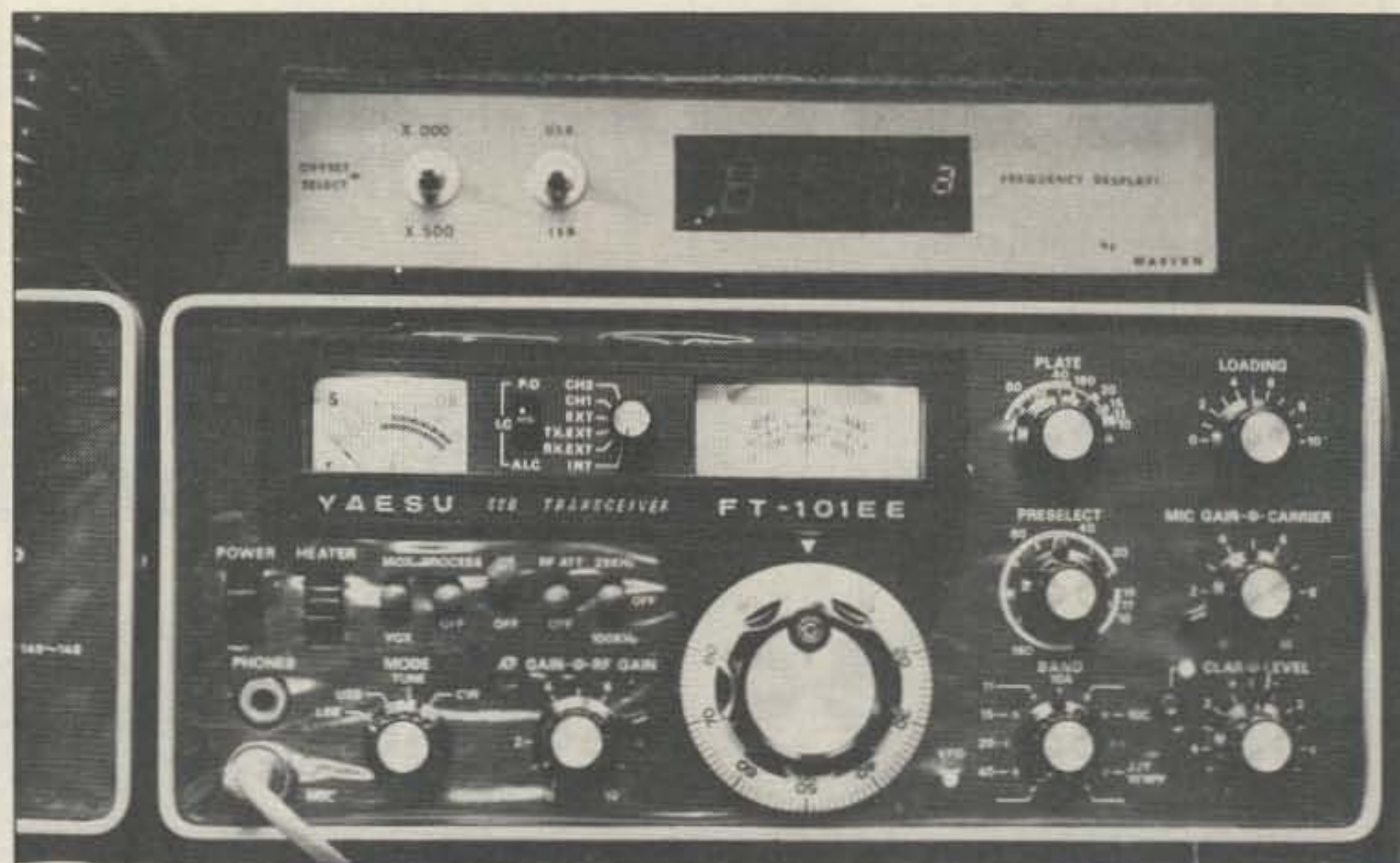
Photo C. Shown here with the Yaesu FT-101EE, this version of the simple frequency display can be used on any analog transceiver.
