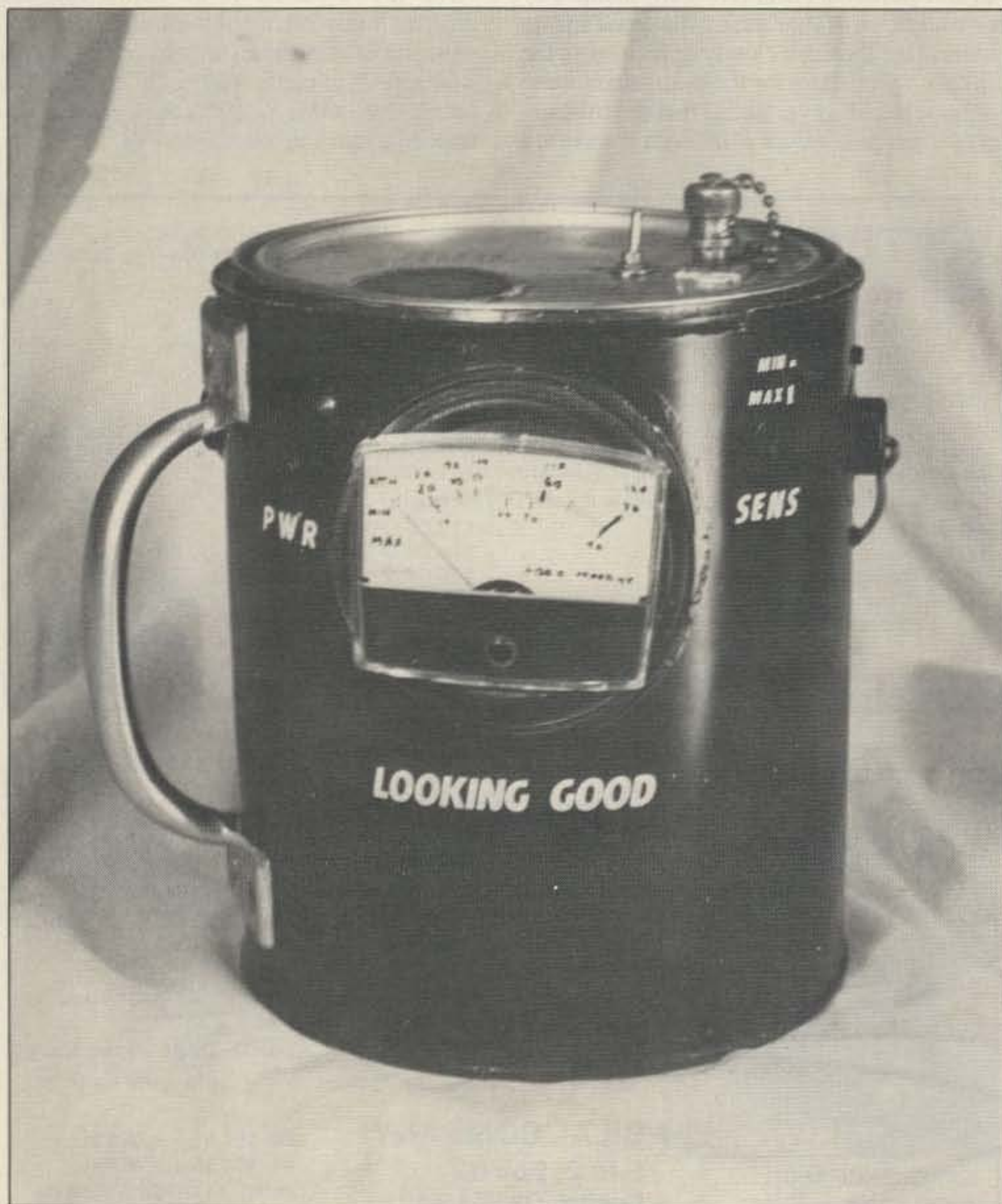
Photo A. Inside this rf-proof can lurks a Tempo S-1 HT.
