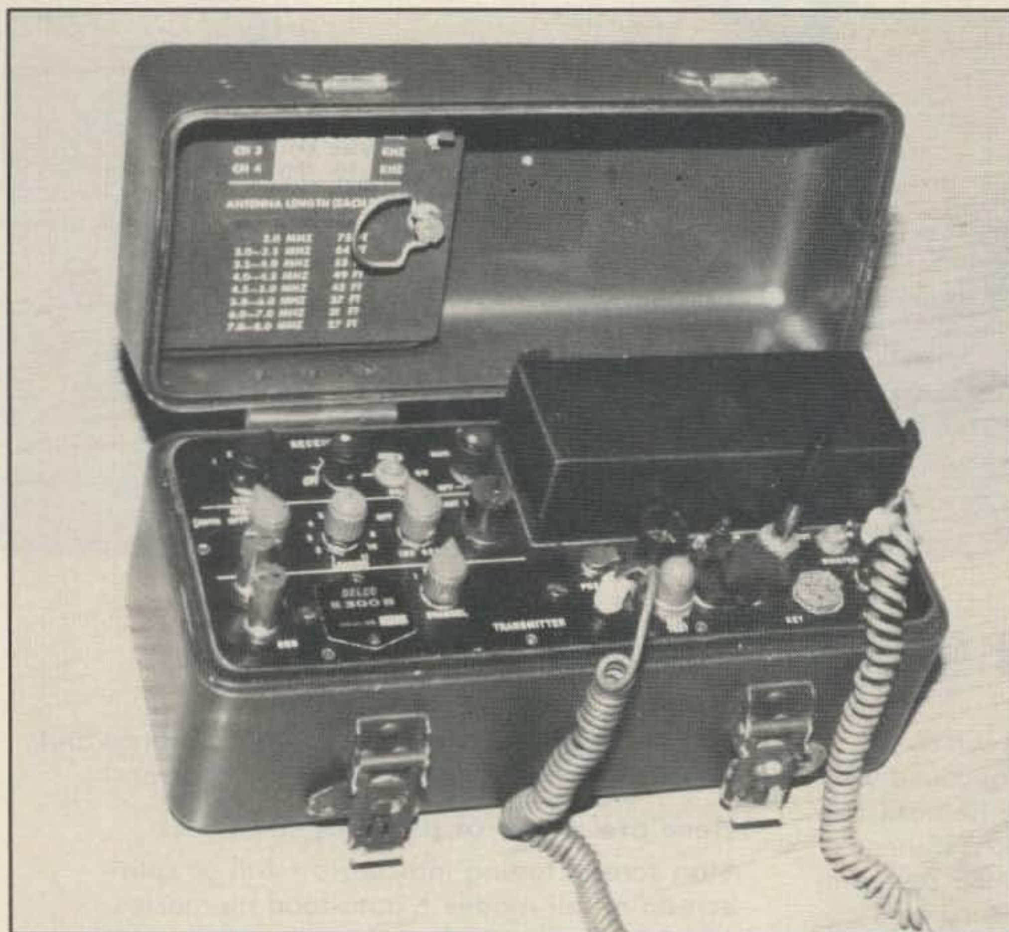
The Delco 5300B, the CIA version of the PRC-64 transceiver.
