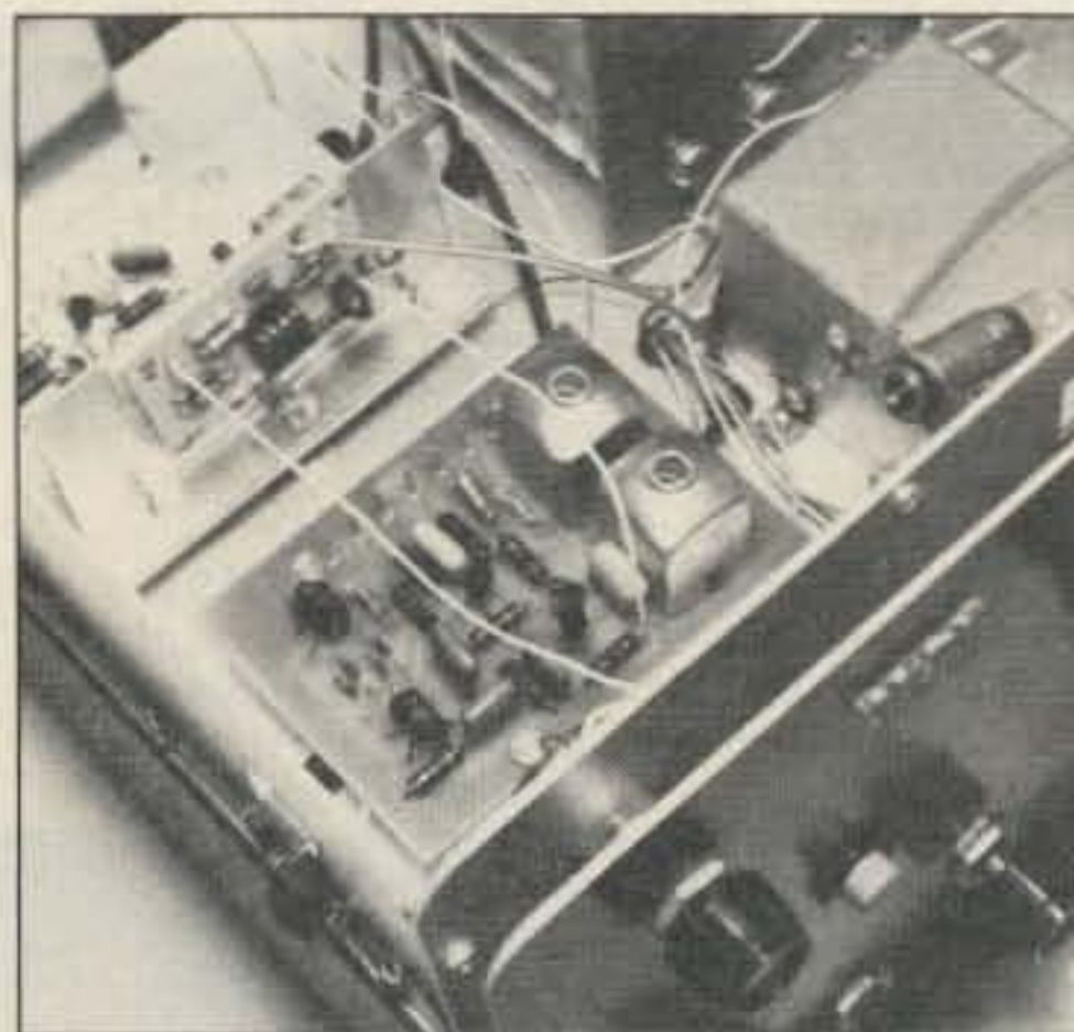
Photo B. PDQ circuit installed in a Century/21.
