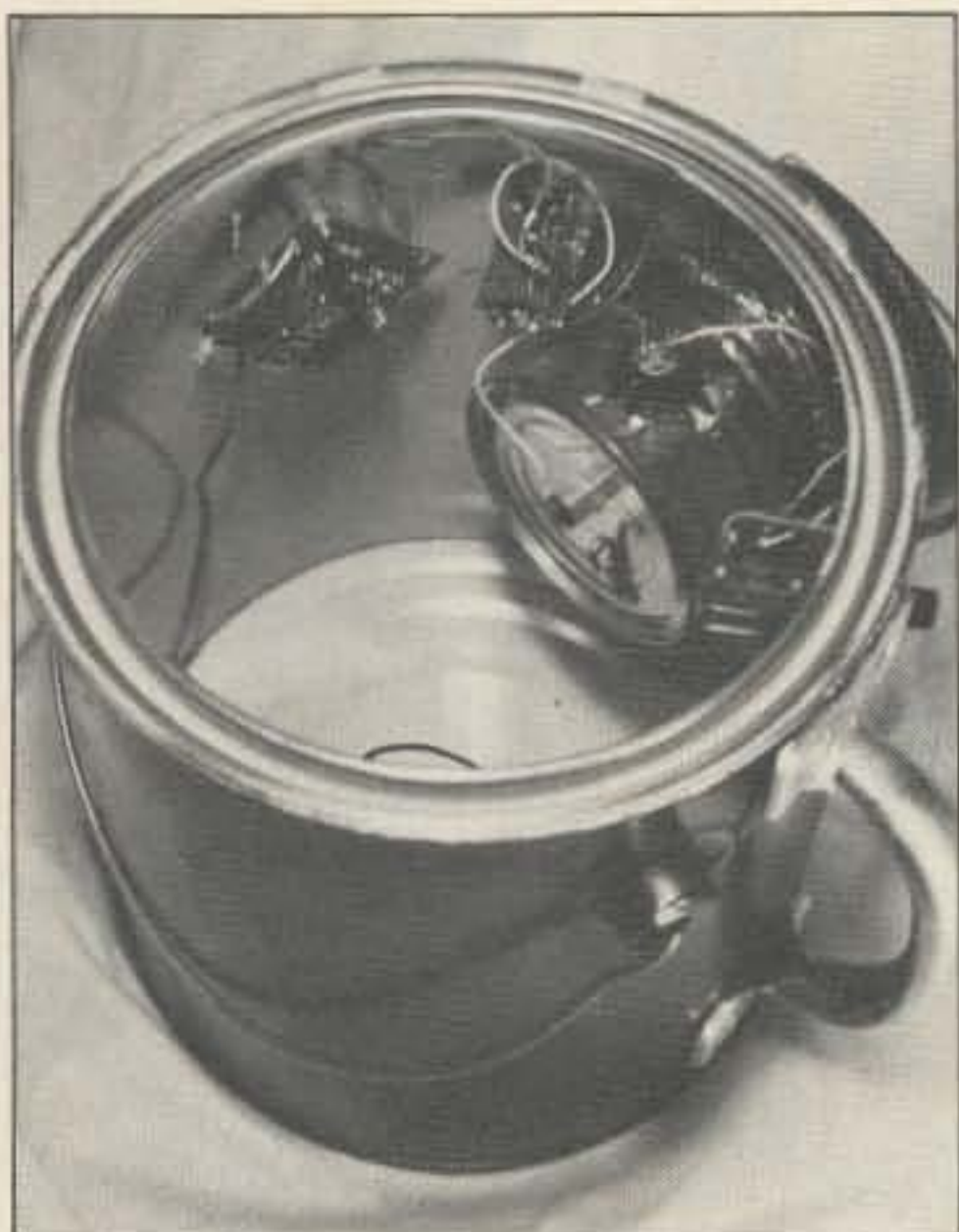
Photo C. Use a double wall for the meter mount.
