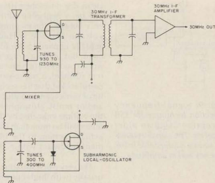
Fig. 7. Simplified circuit of the "business end" of a superhet, with subharmonic oscillator. Contrary to common assumption, the oscillator does not provide harmonics of its fundamental frequency. Rather, the needed frequency multiplication takes place in the mixer.
