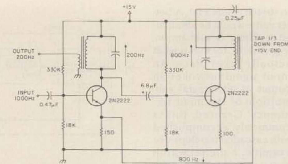
Fig. 5. An experimental transistor version of a regenerative modulator. Although this example circuit operates at low audio frequencies, the basic idea is applicable to radio frequencies as well.
