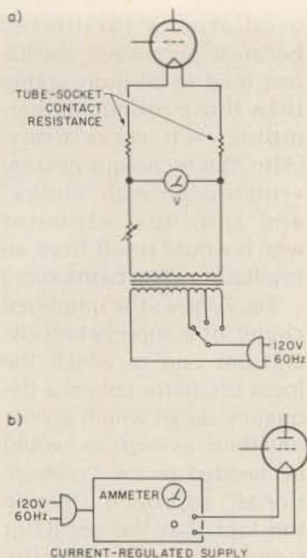
Fig. 8. Traditional and proposed methods of lighting up your transmitting-tube filaments: (a) the "good old way" and manually-adjusted voltage across tube socket may not have been so good after all; (b) proposed technique.
