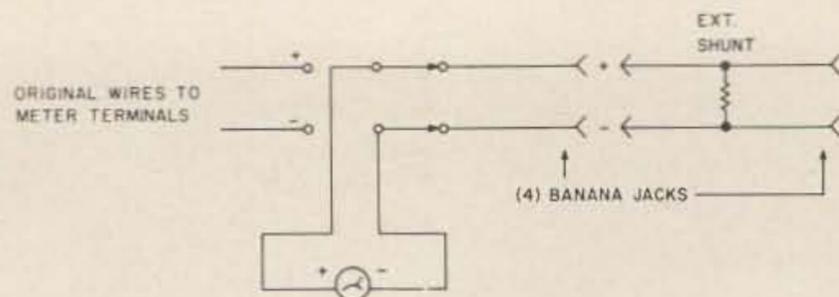
Fig. 3. Milliammeter circuit.
