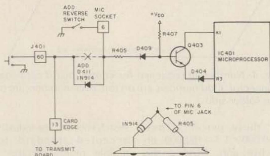
Fig. 6. Reversing switch is mounted in the microphone case. Lift one end of R405 and add D411 as shown.
