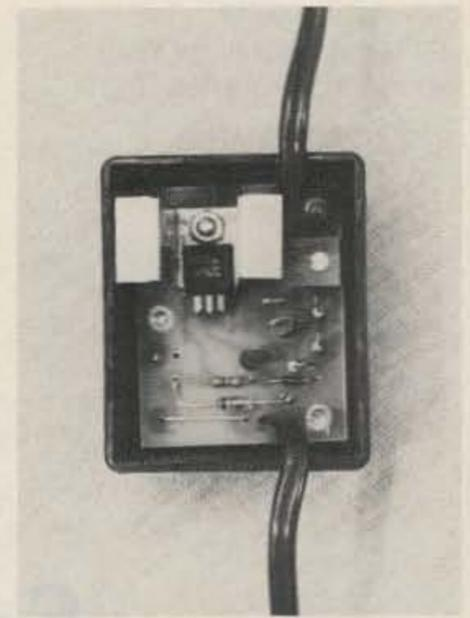
Photo C. Interior view of the dc regulator. The plastic case allowed me to use oversized heat sink for good heat dissipation.
