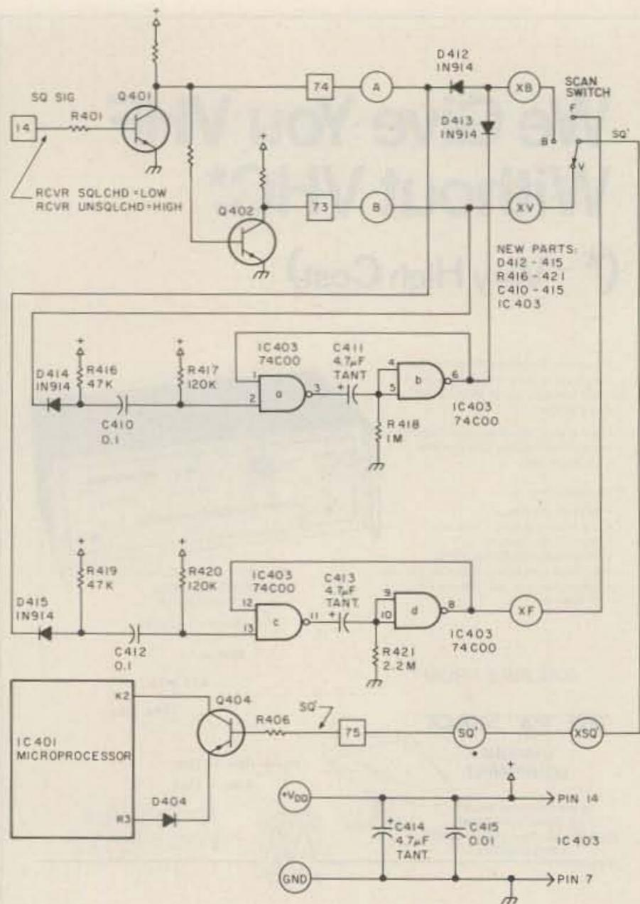
Fig. 9. Scan-control circuits after modification. Numbers in squares refer to existing control-board pin or pad numbers. Numbers in circles refer to inputs and outputs on the new board. IC403A and B and IC403C and D are wired as monostable multivibrators triggered by D414 and D415, respectively. Squelch activity enters through pin 14, upper left. Scanning is stopped while Q404 is turned on; it resumes when turned off, lower left.
