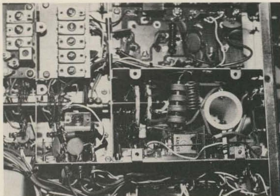
Photo E. The new trimmer C, mounted on S1E. The final amplifier compartment can be seen to the right.
