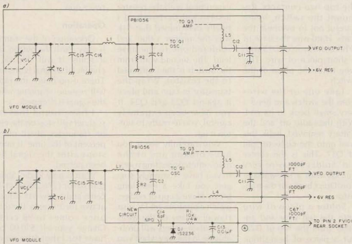
Fig. 1. Partial schematic drawings of FT-101 vfo before (a) and after (b) modification to include RIT circuitry. Components on the added board are indicated in (b).
