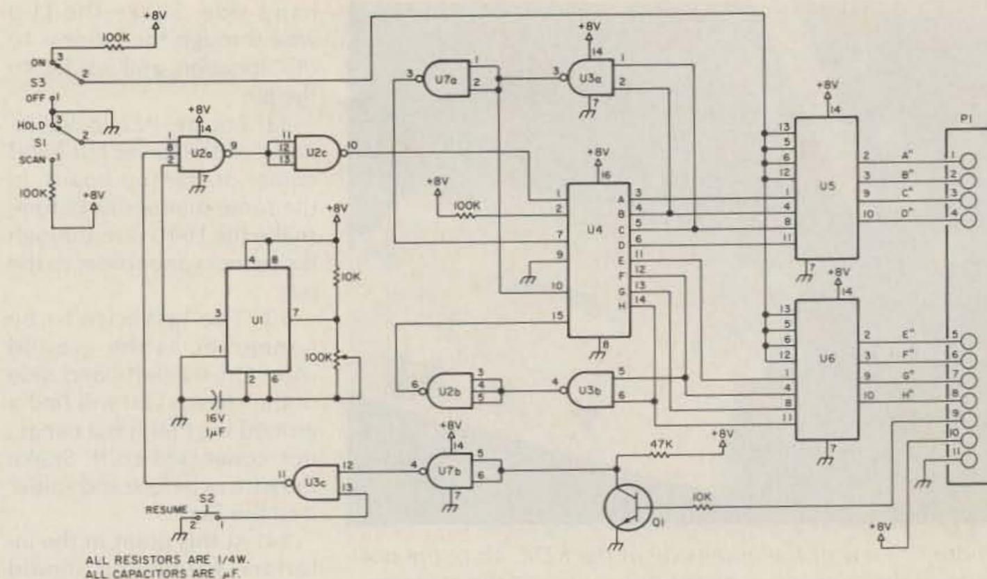
Fig. 1. Schematic of the Scan Can.
