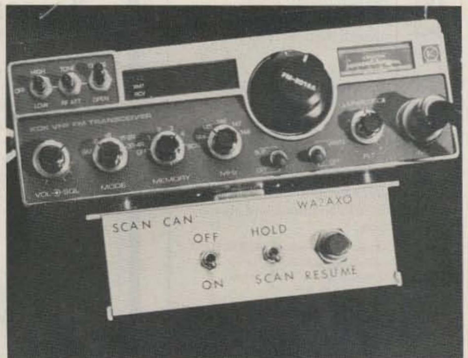
Photo B. The Scan Can mounted in operating position on the KDK.
