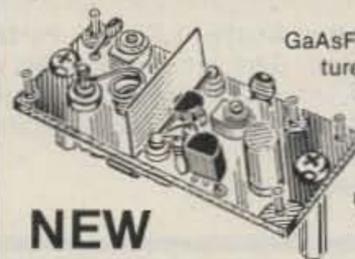
GaAsFET Preamps with features similar to LNG, except designed for LOW COST and SMALL SIZE: only 5/8" W x 1-5/8" L x 3/4" H. Easily mounts inside many radios.
