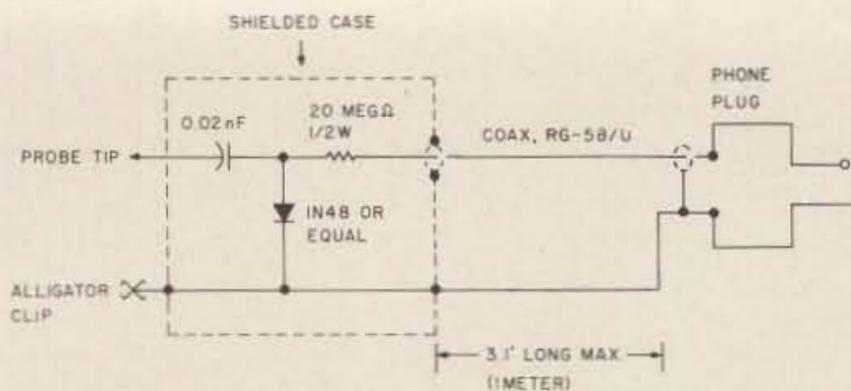
Fig. 2. Rf probe circuit.
