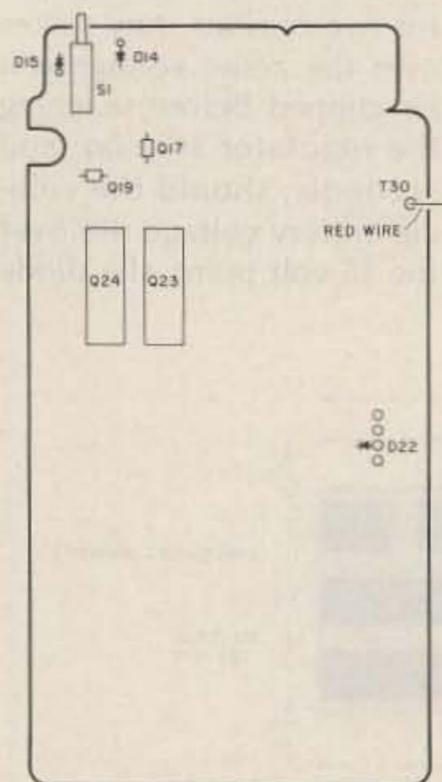
Fig. 1. The PLL board. S1 is the scan-busy switch which is to be modified. The bases of D14 and D15 must be hard-wired together. The collector of the scan transistor is spliced into the red wire at T30. The emitter is wired to the top of D22. The collector of Q17 is taken, through the switch and resistor, to the base of the scan transistor.
