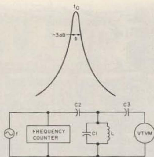
Fig. 2. How unloaded quality factor  $Q_0$  is measured.
