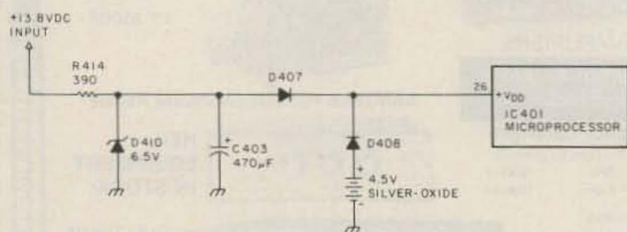
Fig. 1. Original memory-protection circuit uses three silver-oxide cells and charge-protection diode D408 to apply power to the microprocessor while the main power is off.
