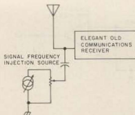
Fig. 9. Signal-frequency injection technique for SSB reception using an older receiver. The signal-frequency source is adjustable in frequency and in amplitude.
