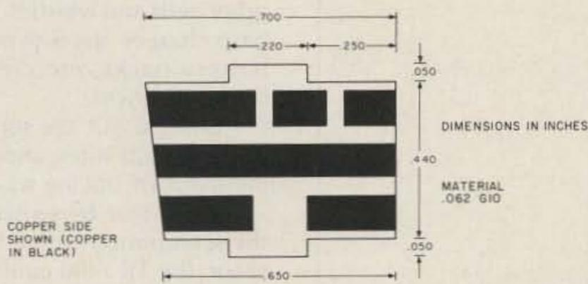
Fig. 2. PC board, external microphone.
