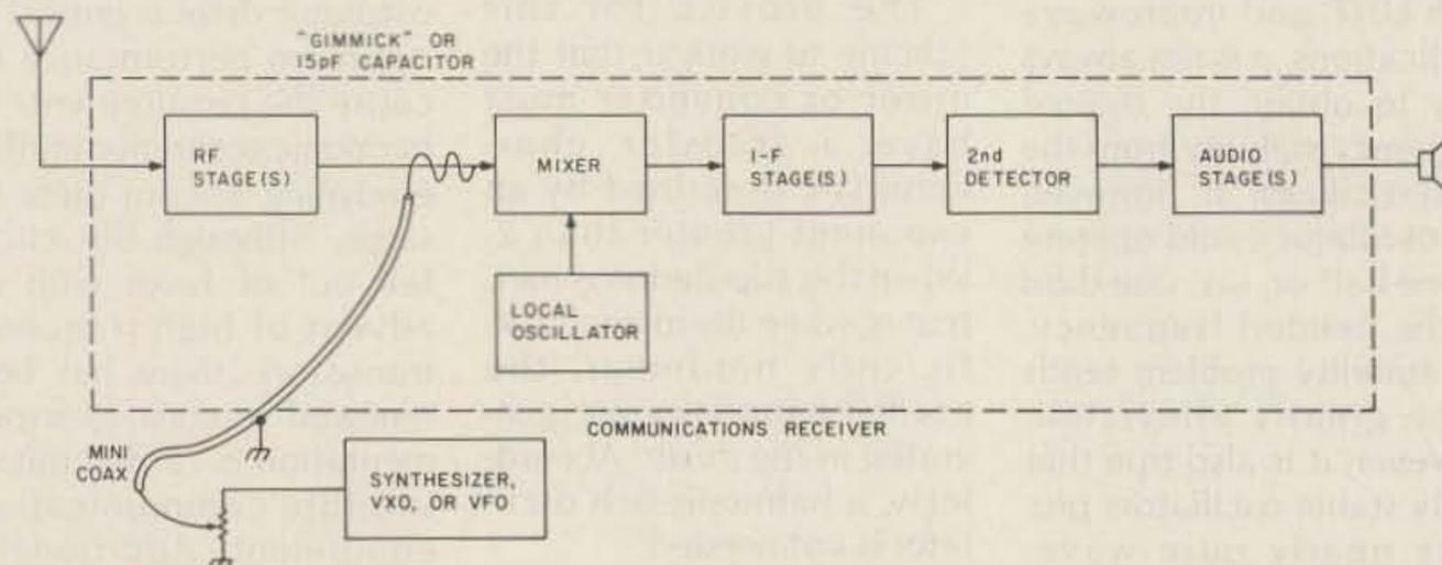
Fig. 10. A somewhat better arrangement for receiving SSB signals with an older set. In this setup, the signal-frequency injection takes place following one or more rf stages. Also, the use of a synthesizer is suggested.
