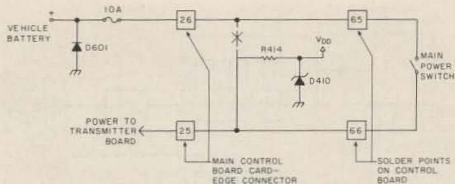
Fig. 3. Moving R414 to the cold side of the power switch eliminates current drain from the vehicle battery when powered off.
