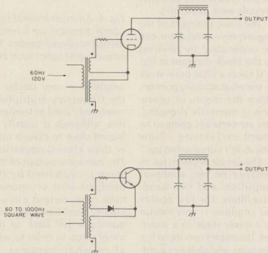
Fig. 6. Tube and transistor versions of the synchronous rectifier: Tube circuit (top) did not provide any noteworthy performance features; transistor version is capable of high-efficiency rectification for high currents and low voltages because internal voltage drop can be much less than for ordinary rectifier diodes.
