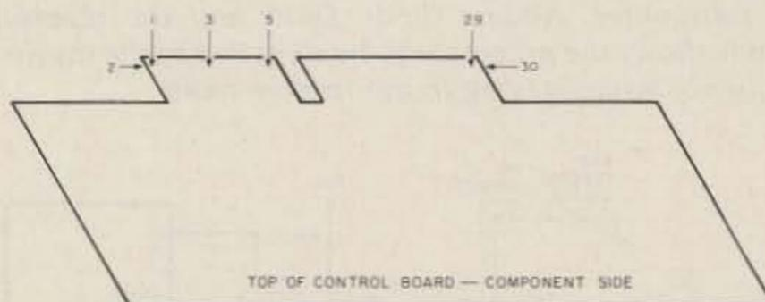
Fig. 4. Numbering sequence for control-board card-edge connector. Odd numbers are on top; even numbers are on the solder side.
