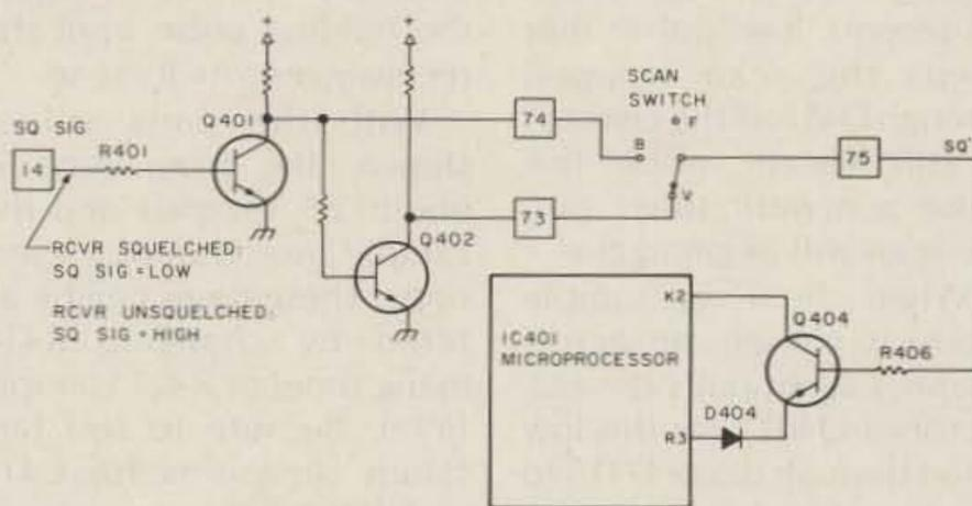
Fig. 8. Scan-control circuits before modification. Squelch activity enters board at pin 14 and arrives at scan-control switch Q404 either inverted or normal or not at all, depending upon the position of the scan switch. Scanning is stopped while Q404 is turned on; it resumes when turned off.
