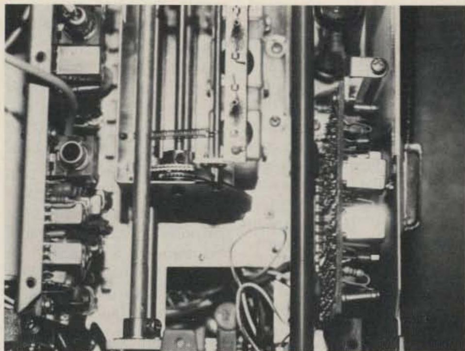
Photo C. The local board on the right and the premix board on the left, near the front of the FT-101Z.
