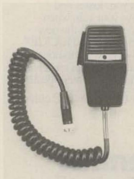
Photo A. Completed speaker/microphone. The mike cartridge is the dark circle in the white strip in the middle of the microphone.
