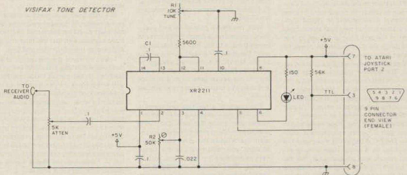
Fig. 1. Tone-detector schematic.
