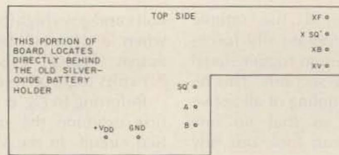
Fig. 10. Constructing the new scan-control circuits on a board this size and shape will allow them to fit neatly inside the control head between the control board and the potentiometer mounting board. The board is shown here as it would be viewed looking from the front of the Azden, down through the existing control board.
