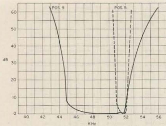
Fig. 4. Measured filter response in switch positions 5 and 9. Response continues beyond -60 dB, but this could not be measured with the simple test equipment at PAQSE.
