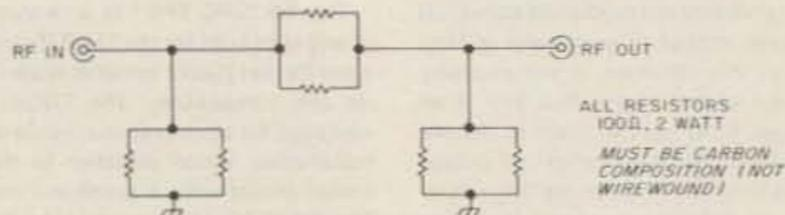
Fig. 1. A simple attenuator for padding down 10-Watt exciters to drive transverters.
