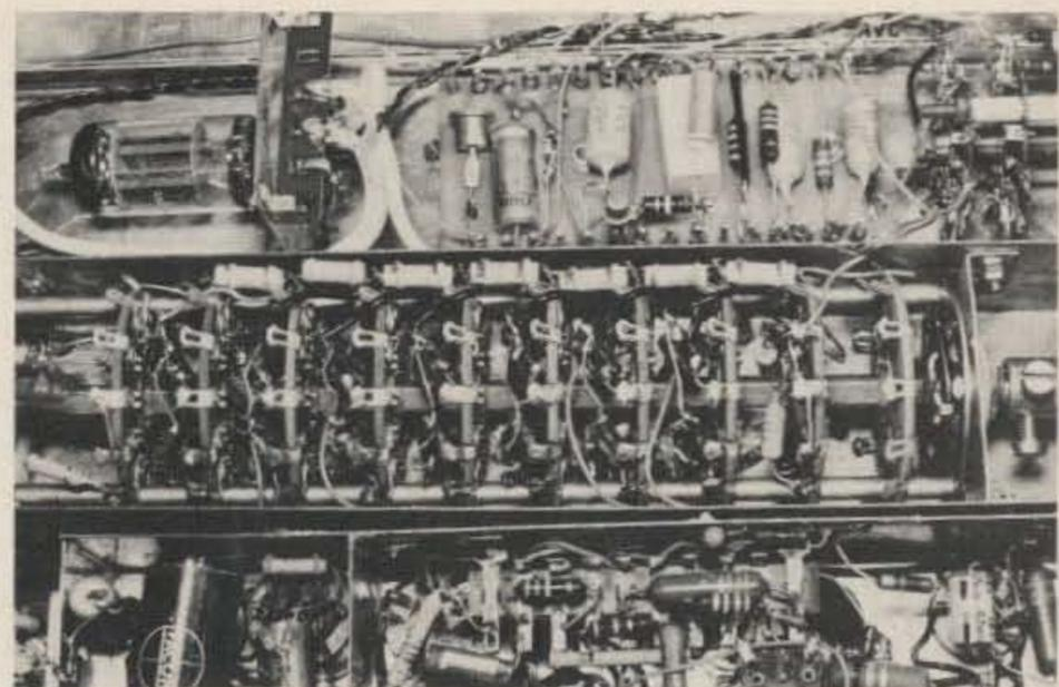
Photo B. View of the filter from the bottom of the receiver. Coupling capacitors and loading resistors are mounted directly on the switch decks.
