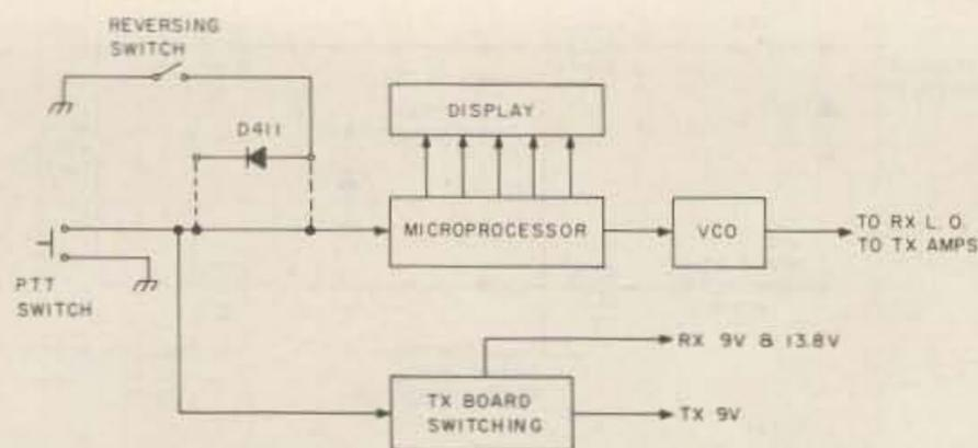
Fig. 5. Engaging the PTT switch causes the microprocessor to change the vco to the transmit frequency and causes the transmit switching to mute the receiver and turn on the transmitter. Adding diode D411 and the reversing switch allows the processor to be switched to the transmit frequency while staying in the receive mode.
