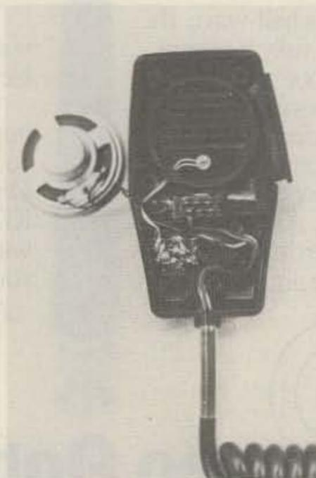
Photo B. Rear view of speaker/mike showing the microphone location. The grommet has been trimmed to allow the speaker to lie flat.
