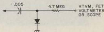
Fig. 6. A simple rf probe.
