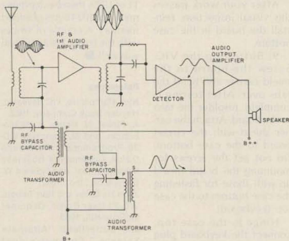
Fig. 1. Basic functional diagram of the reflex receiver. Although the stages were originally configured around tubes, it should be feasible to use solid-state devices such as transistors, FETs, or ICs.
