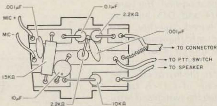
Fig. 3. Parts placement, external microphone.
