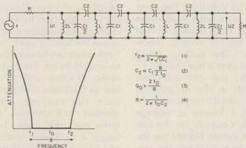
Fig. 1. Basic circuit of a capacitively-coupled bandpass filter.
