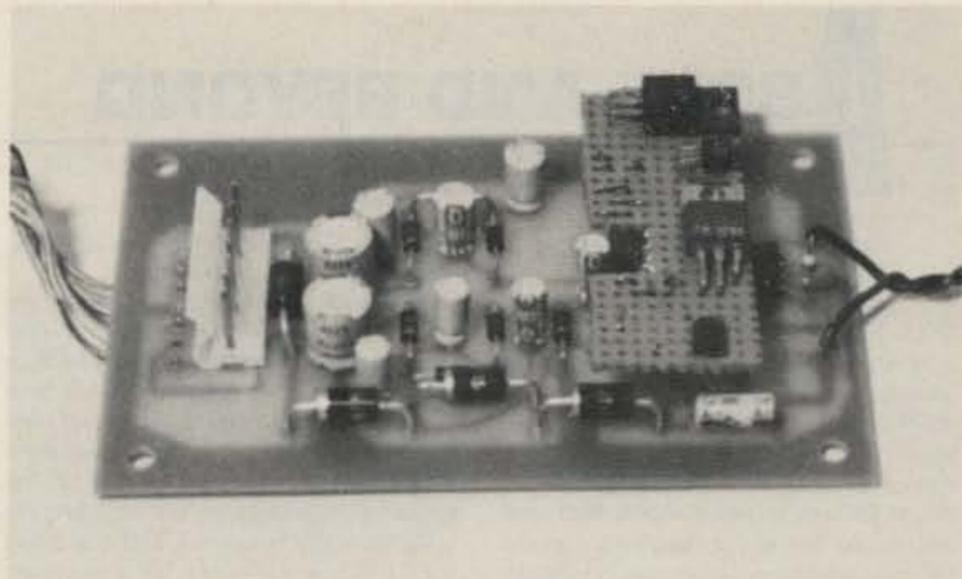
The WA1GRC TPS-1. The perfboard assembly is a modification which is explained in the text.
