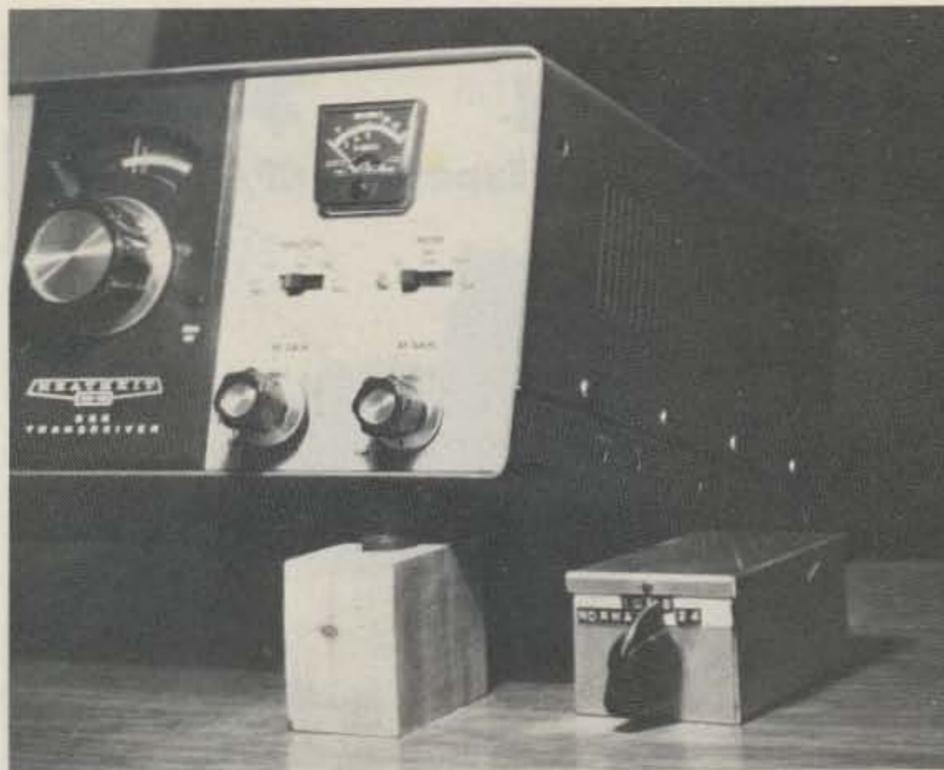
The new hfo circuits and switch are in the small box to the right of the HW-101.
