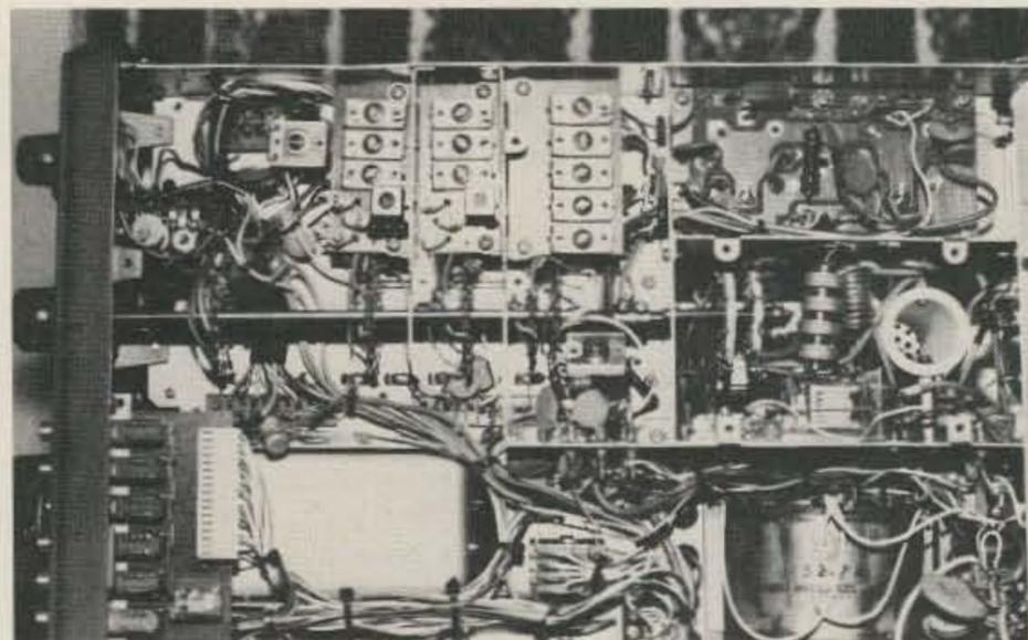
Photo B. Underside of rig showing the two new trimmers installed.
