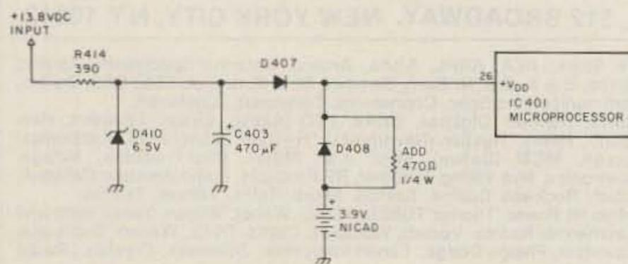
Fig. 2. Modified memory-protection circuit uses a three-cell nicad pack instead of the silver-oxide cells. Adding a 470-ohm resistor across D408 allows the nicad pack to charge whenever the radio is operated.
