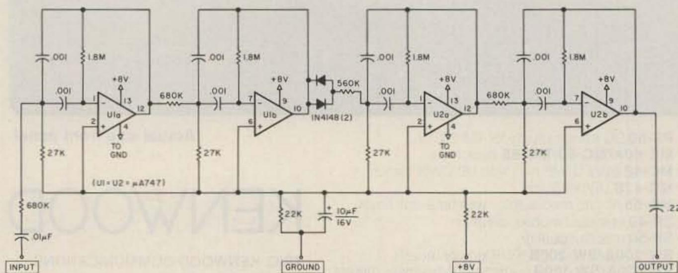
Fig. 1. Schematic diagram.
