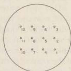
Fig. 7. Front view of the microphone jack showing the pin-numbering sequence.
