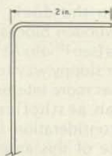
Fig. 5. The aluminum slats are bent at one end to facilitate attachment to the top and bottom of the antenna.
