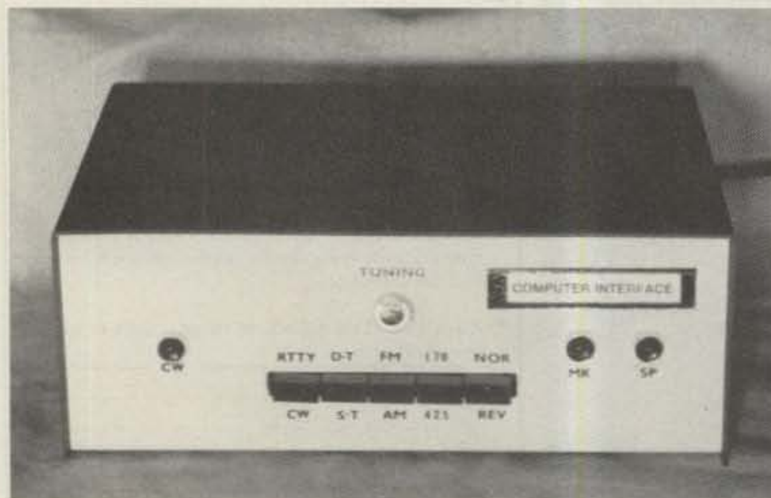
The completed interface. The round object above the switches is the tuning meter.
