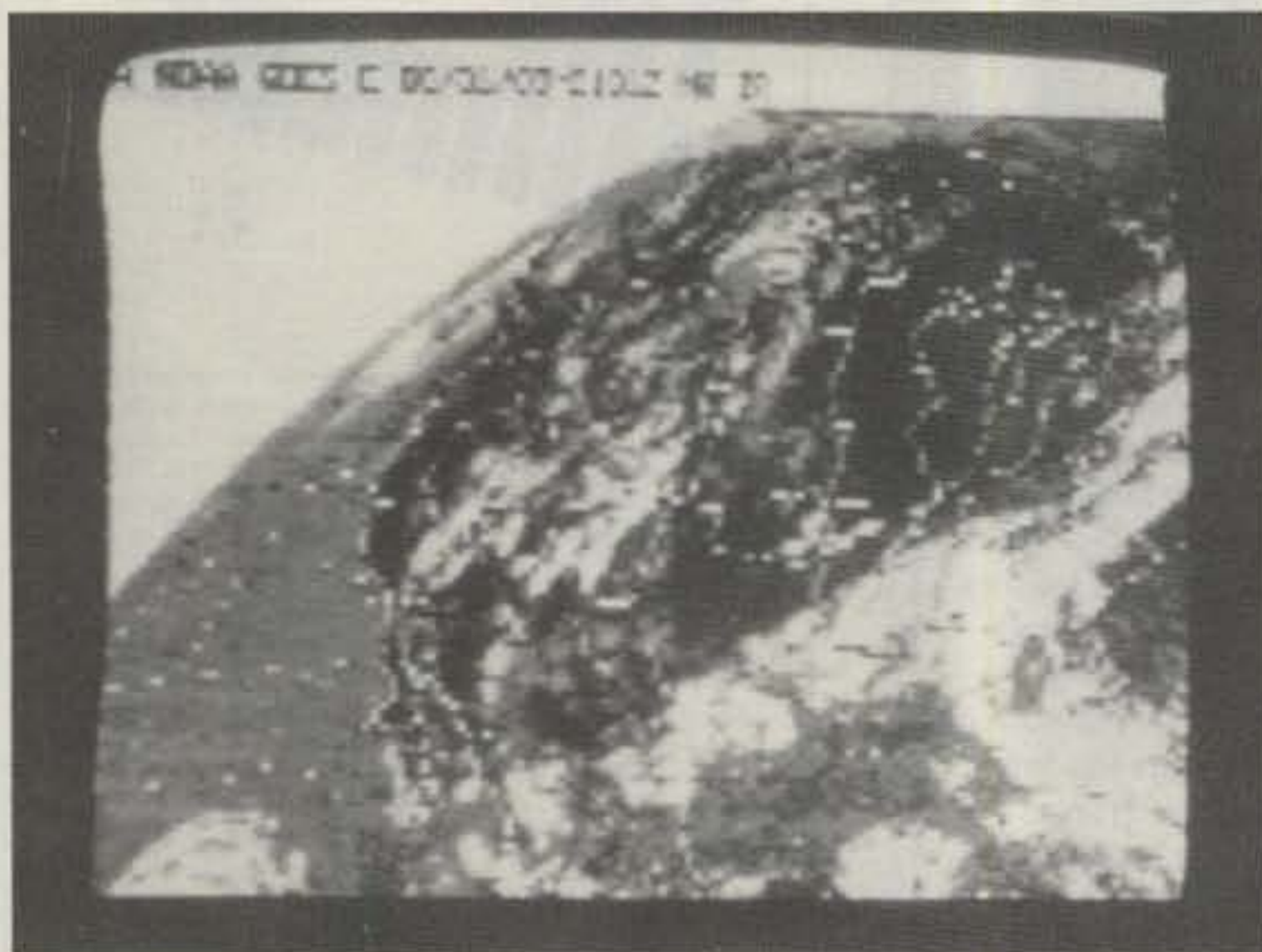
Photo A. An infrared (IR) view of the NW quadrant of the earth as transmitted by the GOES E spacecraft using the WEFAX imaging format. A major frontal system can be seen wrapping around from the Gulf Coast up into New England. Broken frontal activity can also be seen in the Rockies and Plains states. Although some of the gridding of state borders and other features can be resolved, one of the higher-resolution formats (see photos) would be required to capture all the details in a picture of this type.
