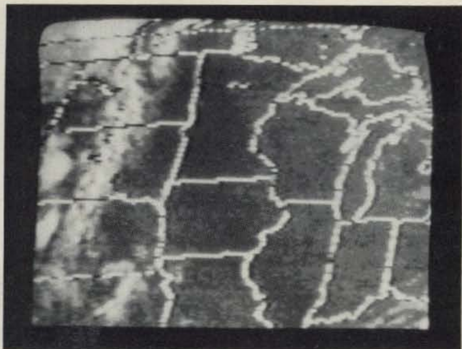
Photo E. Example of High Resolution 1 sampling of an IR WEFAX frame such as in Photo A. It shows a frontal system extending down the central Dakotas into Nebraska.
