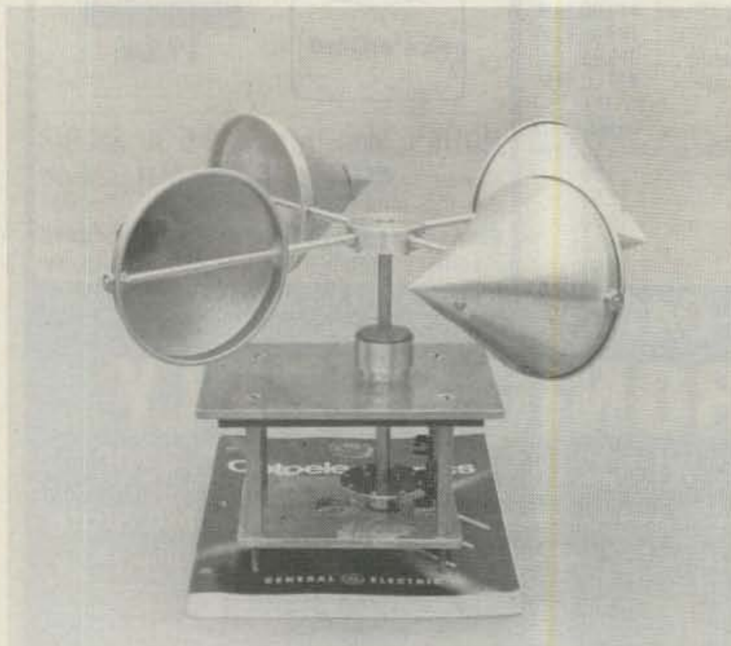
Photo A. Anemometer head with weather cover removed.
