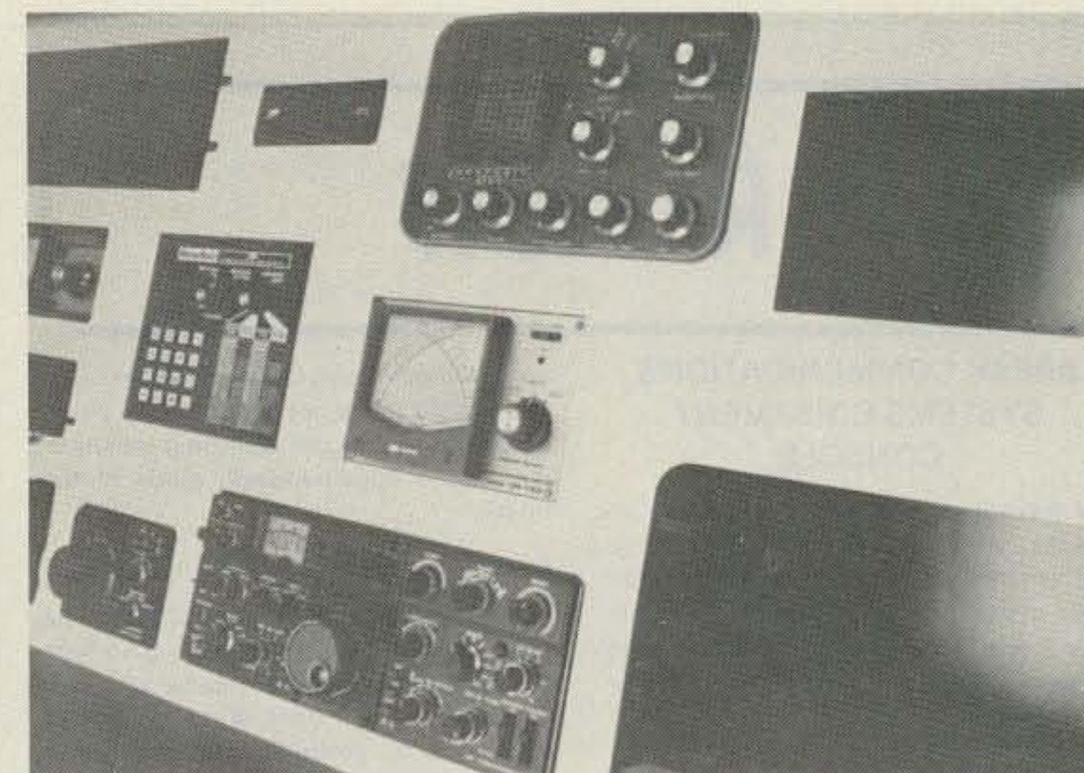
Only the faceplate of each piece of gear protrudes through the front panel, giving the console a sophisticated look.
