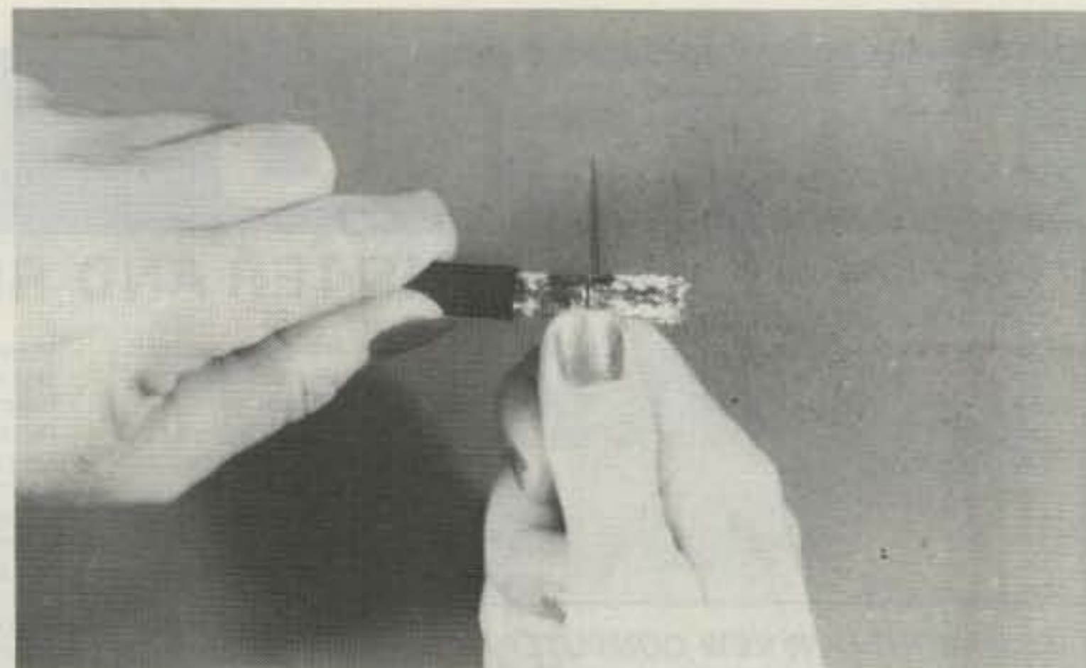
Photo B. Use a sharp knife to cut through soldered braid and insulation.
