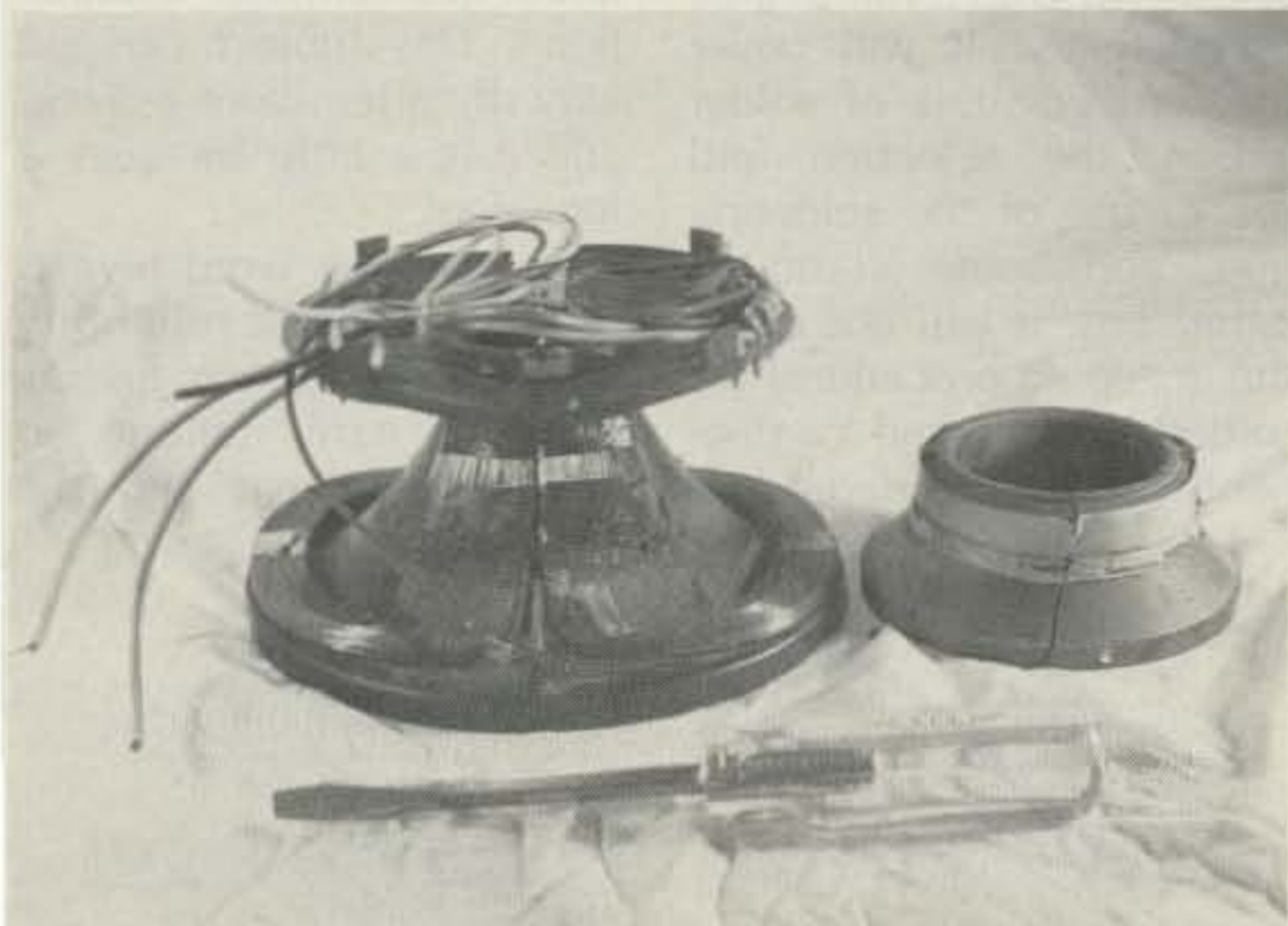
Photo B. The ferrite core is removed from the deflection yoke by releasing the metal restraining band or by cutting the masking tape that holds it in place.
