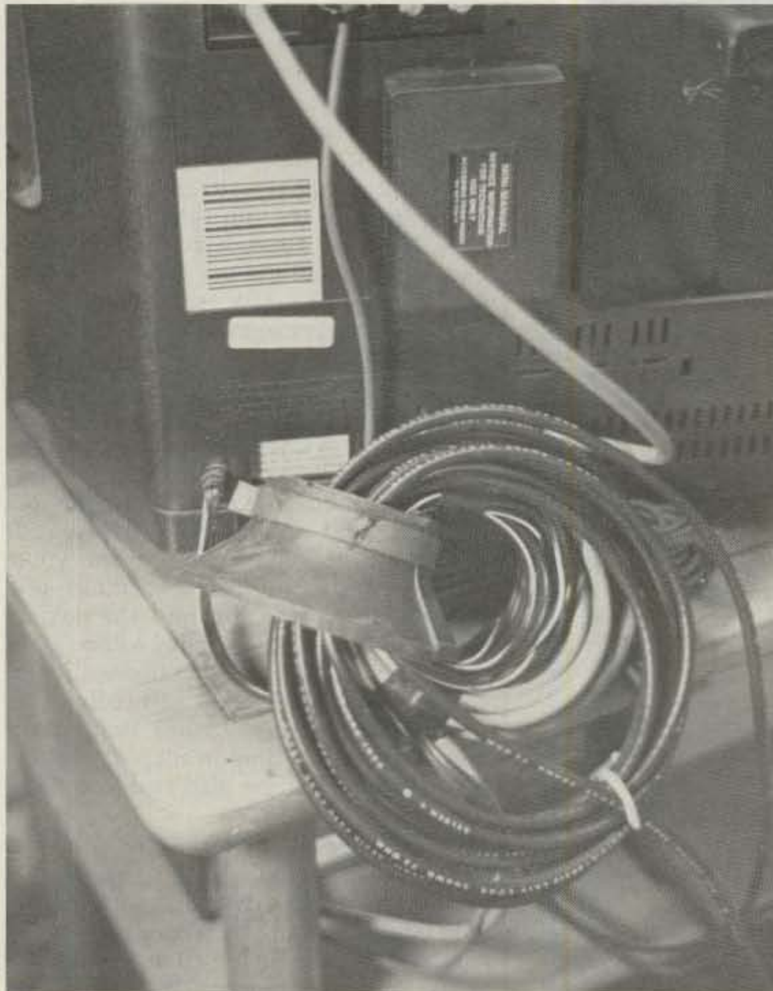
Photo A. The TVI cure in place. The antenna coax and TV power cord are wound in opposite directions through the core to minimize coupling effects.
