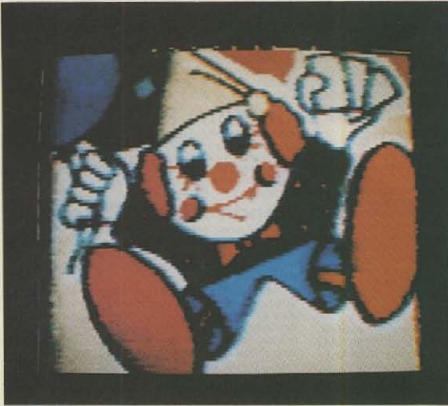
Photo F. A color-SSTV picture displayed on a TI color monitor attached to the K6AEP prototype display board. The picture was received over amateur radio on 28.680 MHz by the TRS-80C and saved on tape. The picture was generated by W00UNB in St. Louis, Missouri.
