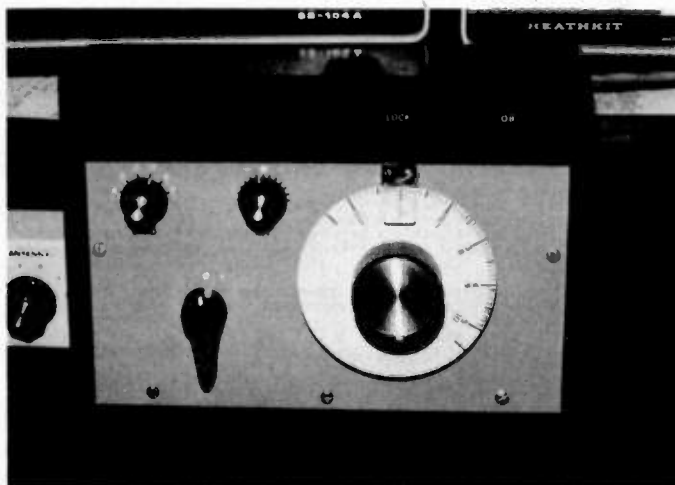
Vfo in operating position, showing panel layout.
