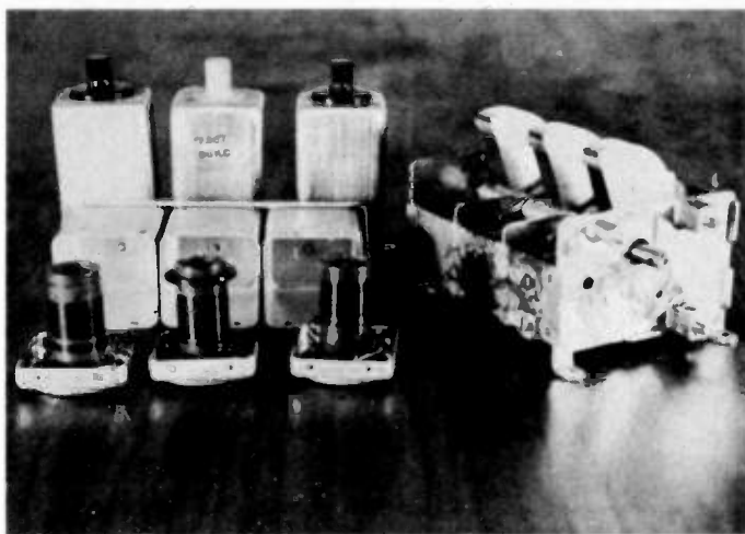
Photo B. The parts used showing a modified variable capacitor.
