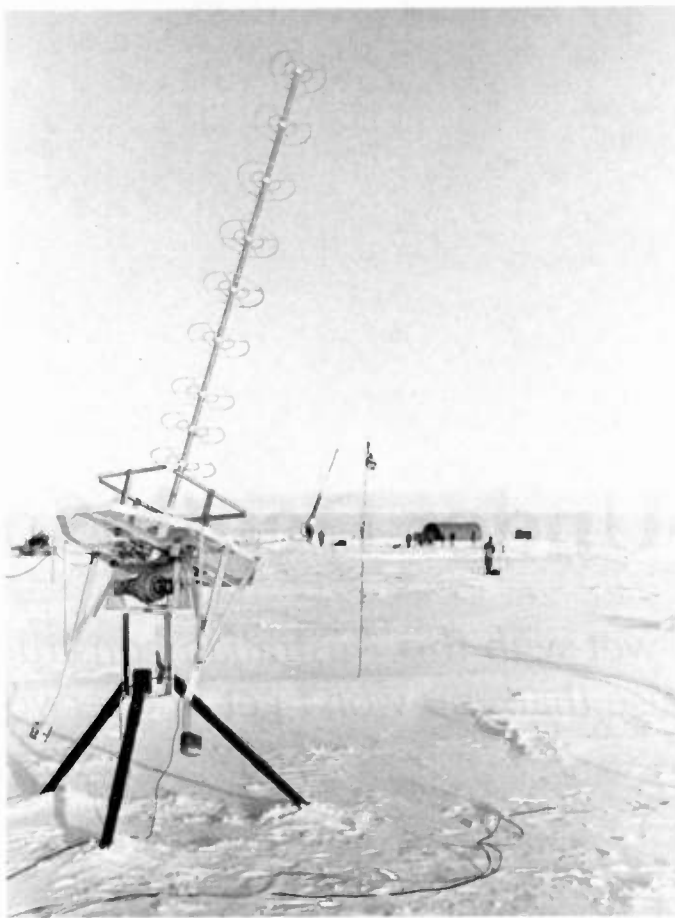
The P-Band antenna at Siple Station, Antarctica, is used to receive data from Nike-Tomahawk rockets launched into the magnetosphere (US Navy photograph).
